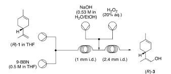
**Figure 1.** Schematic representation of hydroboration–oxidation flow setup. i.d. = inner diameter.
