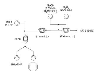
**Figure 2.** Schematic representation of the flow generation of 9-BBN coupled to the hydroboration–oxidation sequence of (*R*)-**3**.
