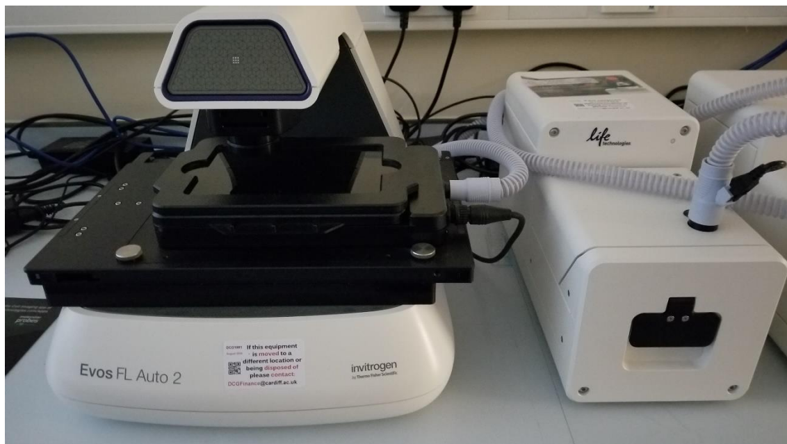
Figure 2.10: EVOS® FL2 Auto Imaging System with EVOS® Onstage Incubator, which provide the environment condition at 37°C, 5% CO 2 for cells, and record the cells via the various zoom of microscope.
