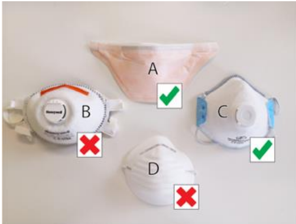
Figure 5: Compatibility of different respirator models with MGS-reprocessing at 1800 W for 90 seconds. Kimberley-Clark N95 respirators (A) and a metal free FFP2 respirator (C) showed no signs of damage following reprocessing. A Honeywell FFP3 respirator (B) and generic unbranded PPE (D) were both damaged by the microwave procedure.
