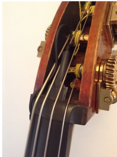
Fig 7.2: Nut pickup detail
