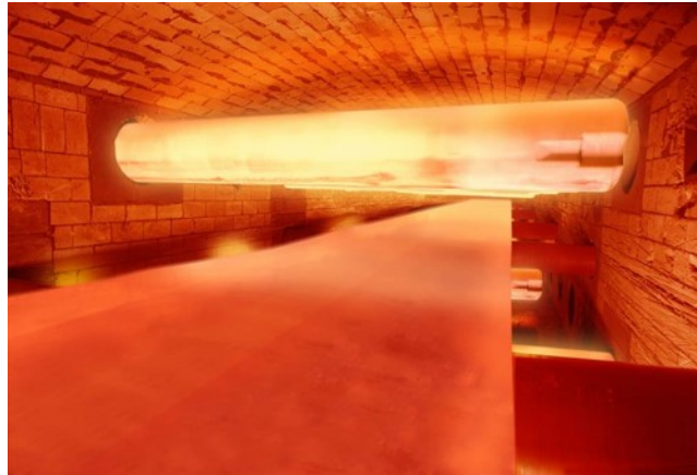
Figure 1.2: Radiant tubes inside an electrical steel annealing furnace.
