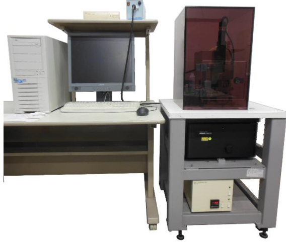
Figure 3.12: ENT-1100 nanoindentation instrument (accessed at Keio University, Japan).
