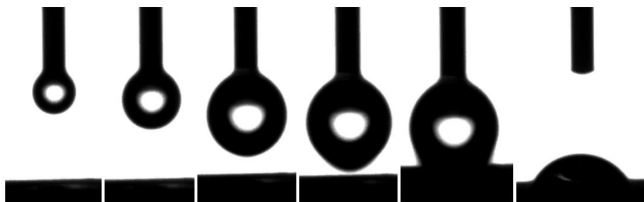
Figure 3.9: The process of placing the liquid droplet on the sample surface.
