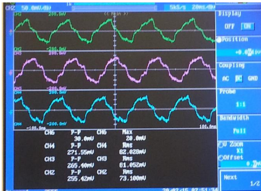
Figure 11. Inverter output currents under load condition
