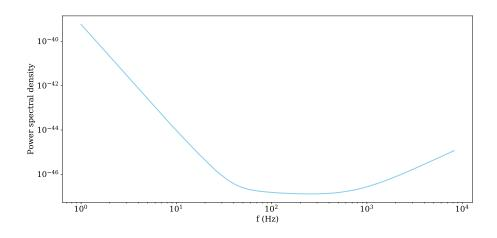
Figure 1.1: Idealised sensitivity curve for aLIGO at design sensitivity.
