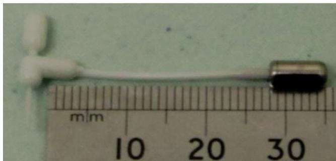
*Figure 7-1. Miniaturised catheter system prior to implantation.*
