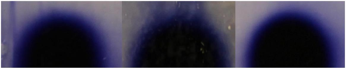
**Figure 5-10. The distal edge of distributions in the agarose gel from an 18 mm step length catheter infused at a) 0.1 ml/hr, b) 0.3 ml/hr, c) 0.6 ml/hr.**
