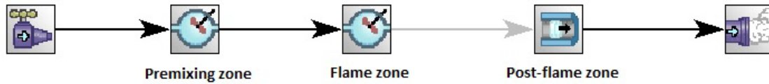
Fig. 8 Simple chemical reactor network model of the 15 mm Bunsen burner in CHEMKIN
