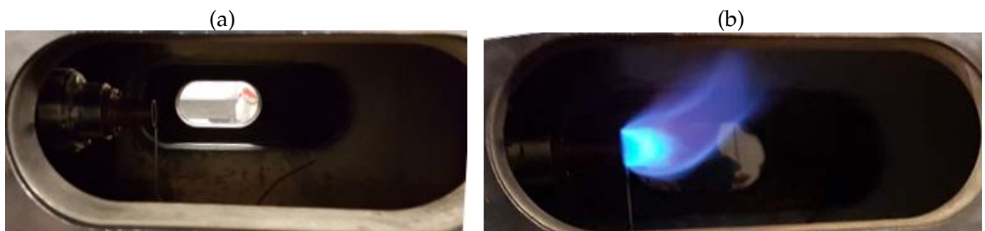
Fig. 2 25 mm Bunsen burner horizontal set-up, as installed (a) and with CH 4 -air flame (b).
