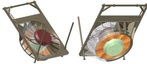
FIGURE 2.18: Very low head turbine (MJ2 Technologies, 2011)
