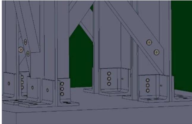
FIGURE C.18: Steel to steel and steel to concrete connections
