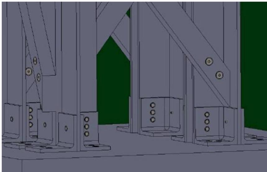
FIGURE C.26: Overview of steel to steel and steel to concrete connections
