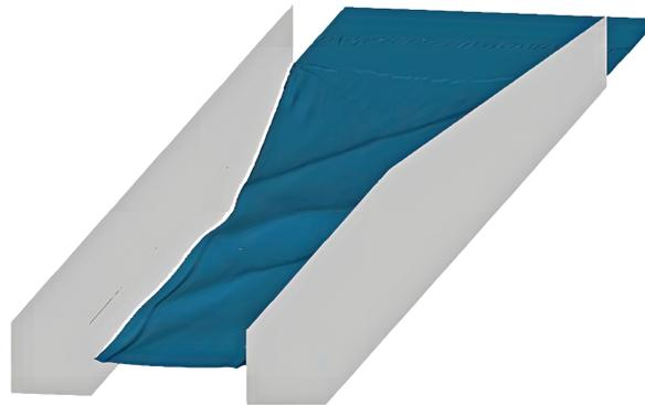
FIGURE 7.6: Time-averaged three dimensional water surface
