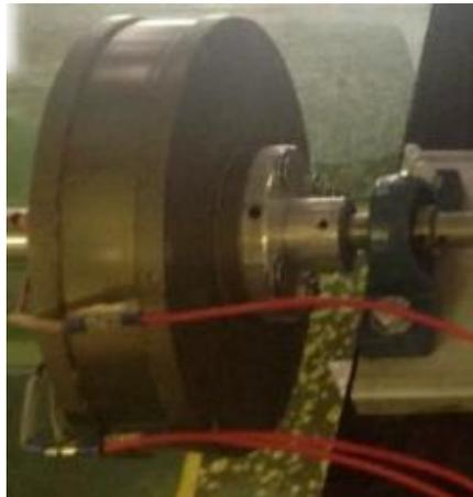
FIGURE 3.10: DVE200 Permanent magnet, three phase off-the-shelf generator
