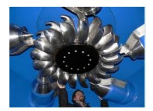
FIGURE 2.12: Pelton Turbine (Hydrolink, 2009)
