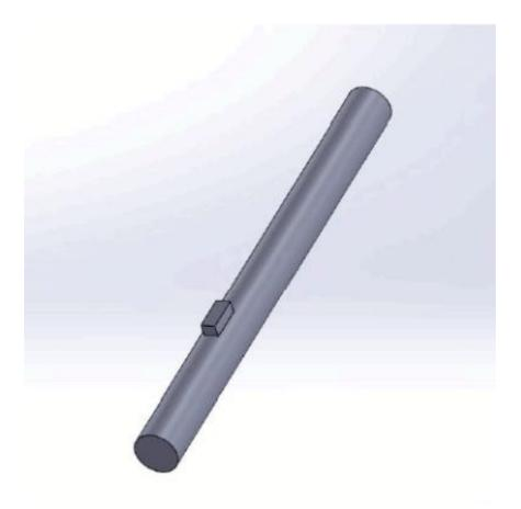
FIGURE C.31: Runner shaft, 0.06 m diameter stainless steel
