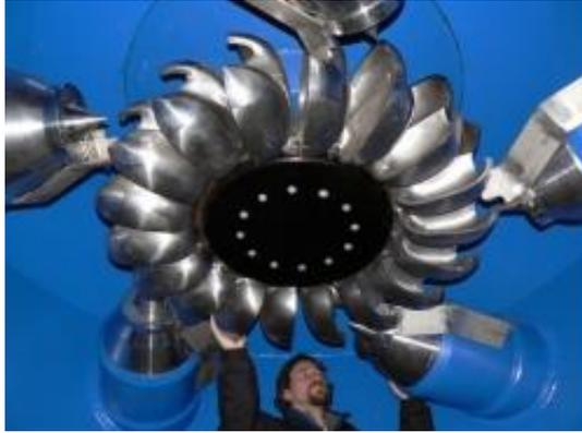
FIGURE 2.12: Pelton Turbine (Hydrolink, 2009)
