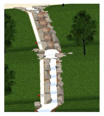
FIGURE C.2: Visualisation of the site including the two-section flume next to the stream and two spillway turbines
