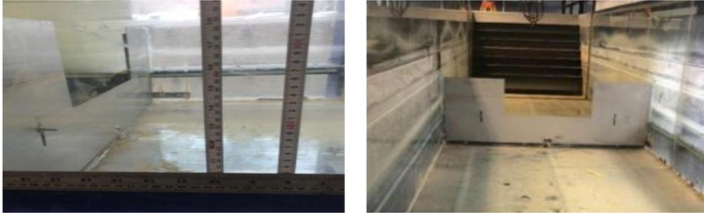
FIGURE 3.4: Laboratory rectangular weir set up
