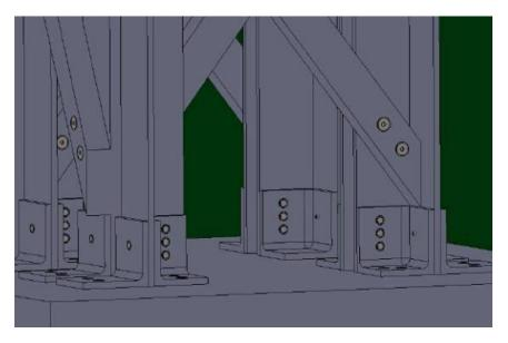
FIGURE C.26: Overview of steel to steel and steel to concrete connections
