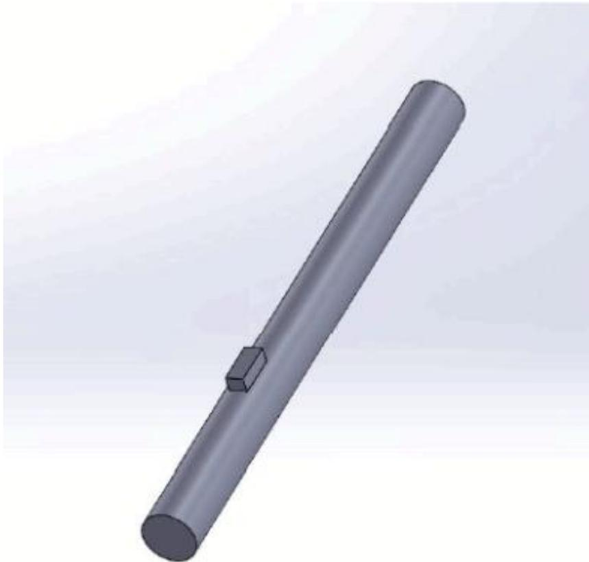
FIGURE C.31: Runner shaft, 0.06 m diameter stainless steel
