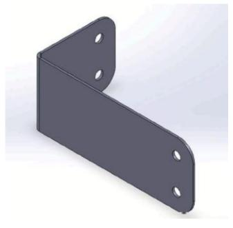
FIGURE C.16: Contraction connection L-bracket
