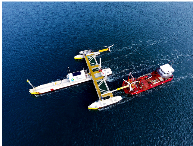
Figure 2.3: The PLAT-I platform using 4 of the Schottel SIT250 devices [33].
