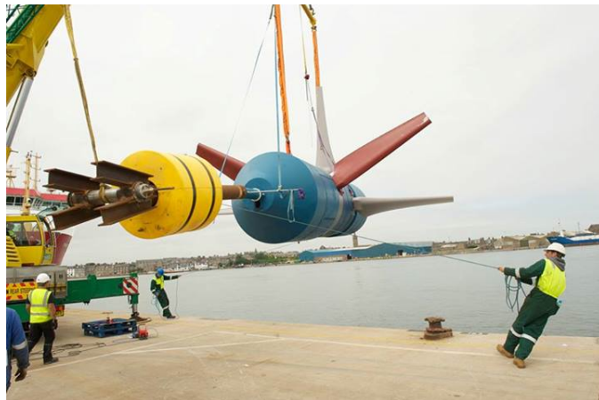
Figure 2.5: The contra-rotating CoRMat device developed by Nautricity [36].
