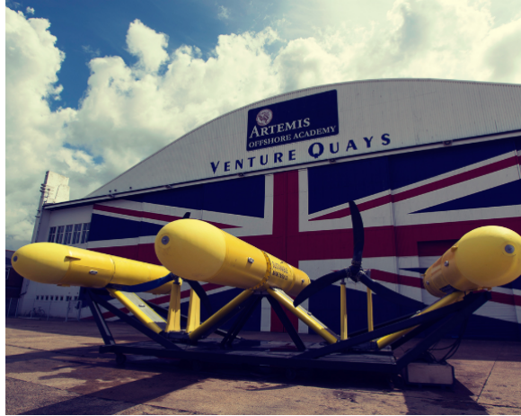
Figure 2.4: The PLAT-O platform using 4 of the Schottel SIT250 devices [34].
