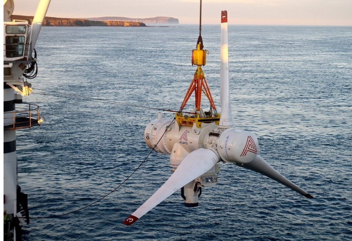
Figure 2.2: The AR1500 device from Atlantis that is currently deployed in the Pentland Firth [31].
