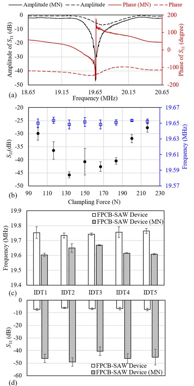
Fig. 2. Characterization of the FPCB-SAW device. (a) The amplitude and phase of the reflection coefficient  $S_{11}$  of the FPCB-SAW device with and without the matching network (MN). (b) The relationship between the  $S_{11}$  / the Rayleigh mode frequency and the clamping force. The reproducibility in (c) the Rayleigh mode frequency and (d) the minimum  $S_{11}$  of the reassembly of the FPCB-SAW device with and without the MN.
