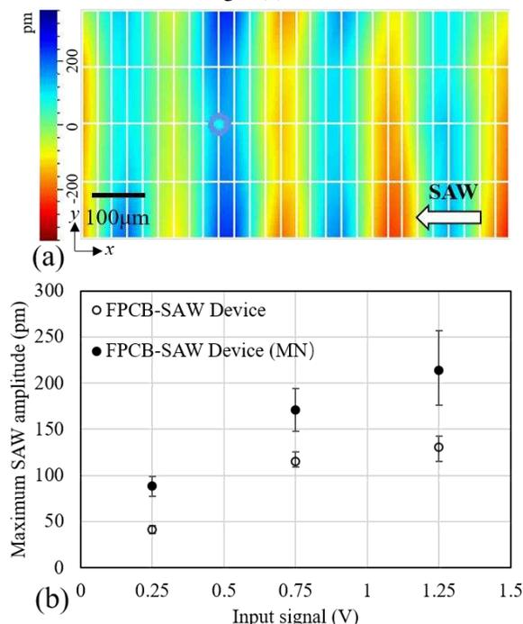
Fig. 4. Surface vibration of the FPCB-SAW device. (a) The vibration pattern of the SAW traveling on the surface at the input voltage of 1.25 V. (b) The comparison of the maximum SAW amplitude of the FPCB-SAW device with and without the matching network at a series of the input signals.
