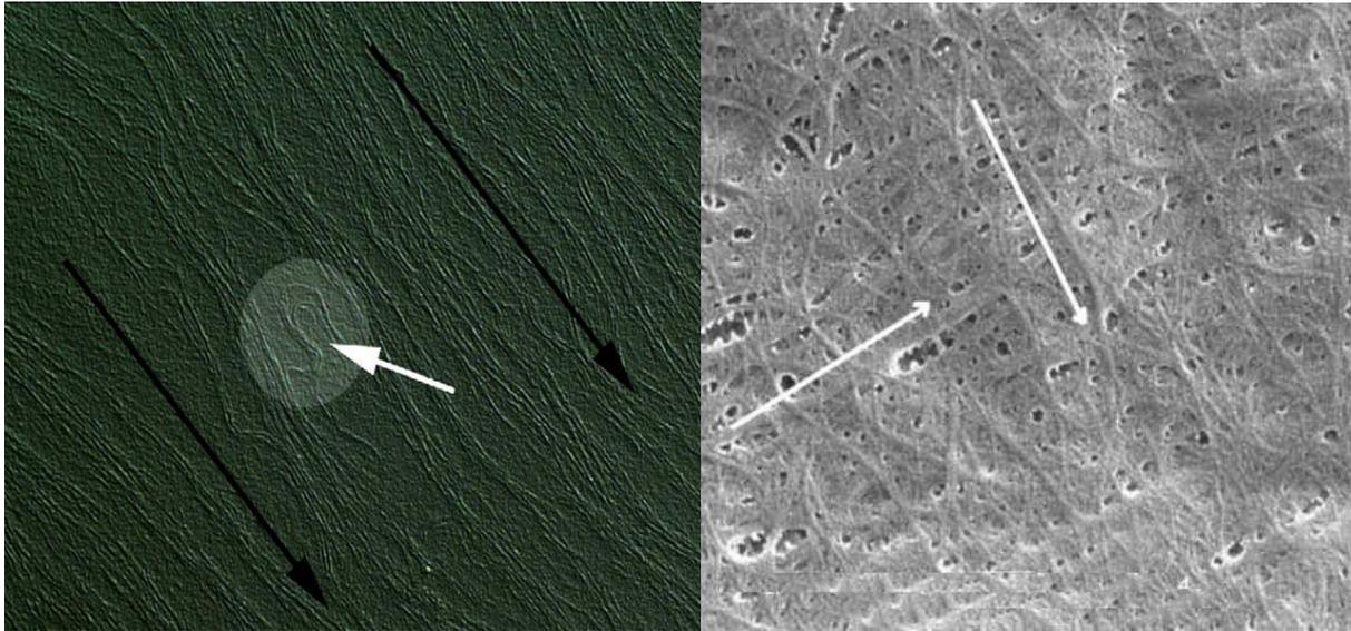
**Figure 1.14: Spin coating method of collagen deposition.**
