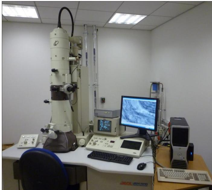
**Figure 3.1: JEOL 1010 Transmission electron microscope.**
