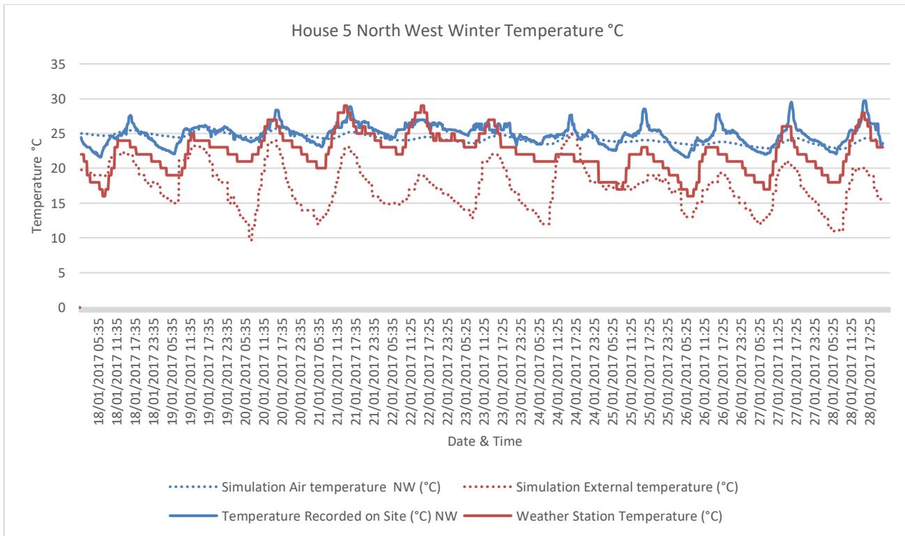
Figure 7.22 - House 5 Simulation Temperature Comparison Winter – NW
