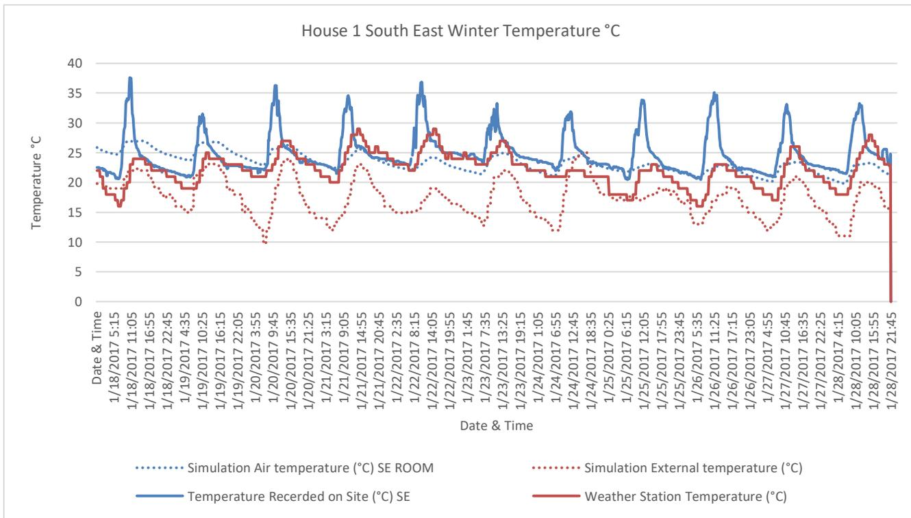
Figure 7.6 - House 1 Simulation Temperature Comparison Winter – SE
