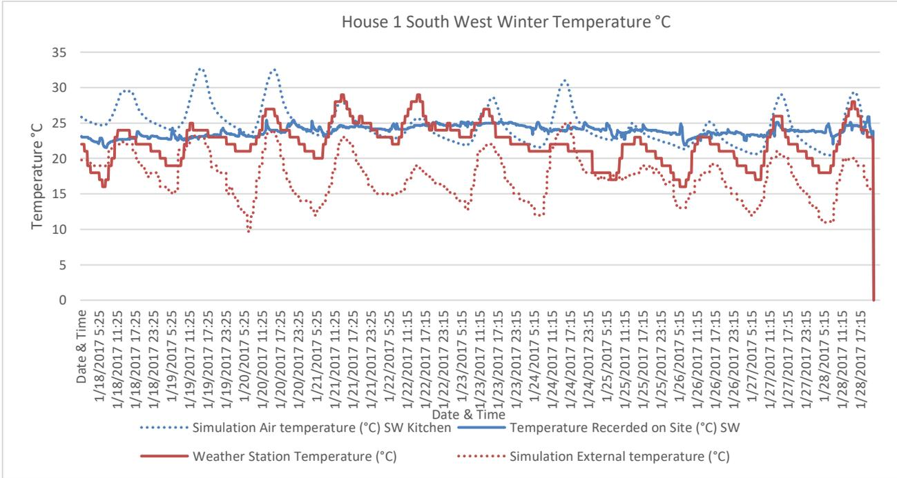
Figure 7.7 - House 1 Simulation Temperature Comparison Winter – SW
