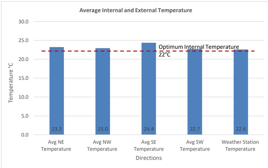
Figure 4.27 - Average Internal and External Temperature - Case Study 1
