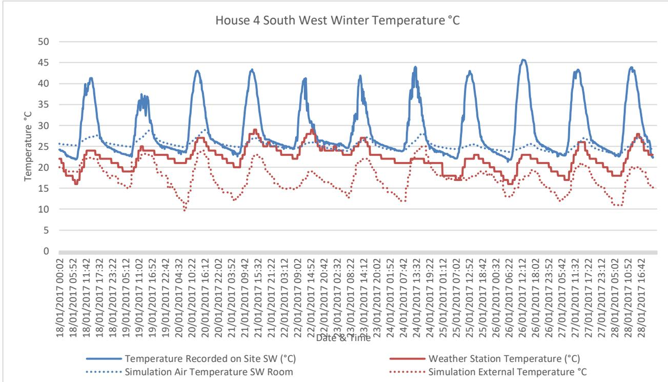
Figure 7.19 -House 4 Simulation Temperature Comparison Winter – SW
