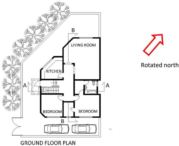
Figure 7.26- North Arrow Rotated  $90^\circ$  West – Study 1
