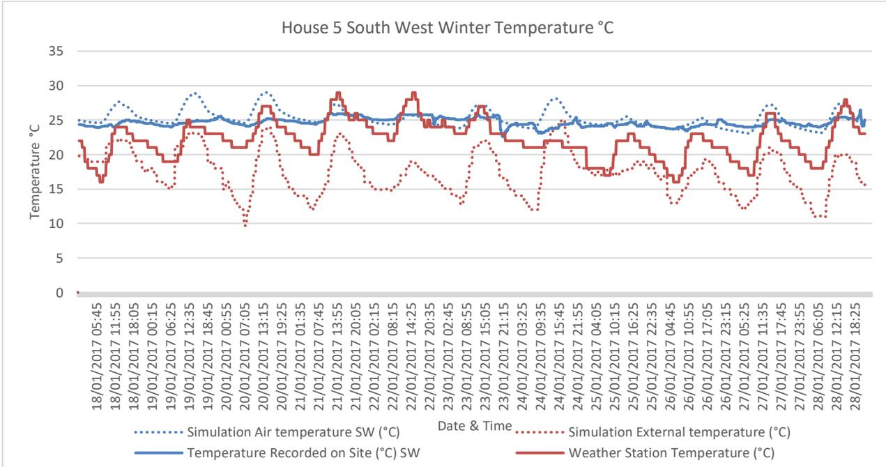
Figure 7.23 House 5 Simulation Temperature Comparison Winter – SW
