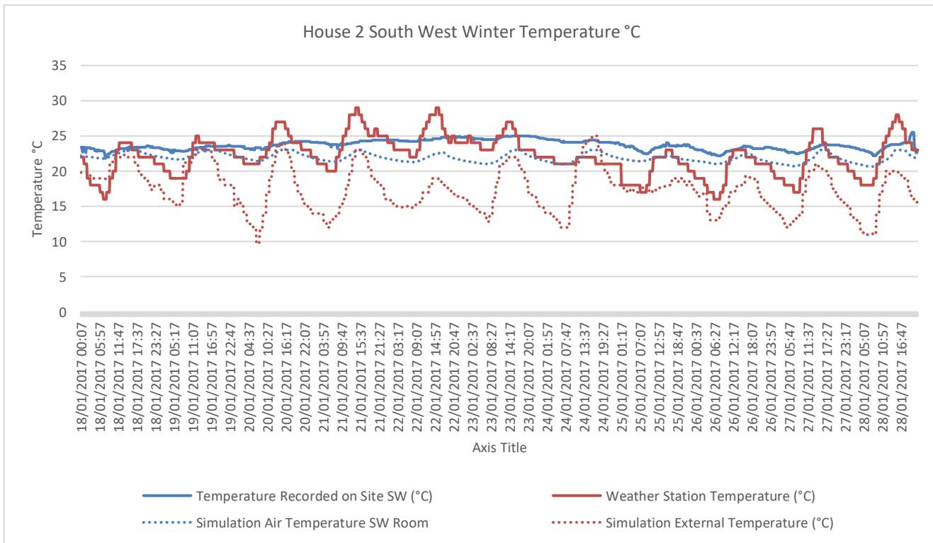
Figure 7.12 -House 2 Simulation Temperature Comparison Winter – SW
