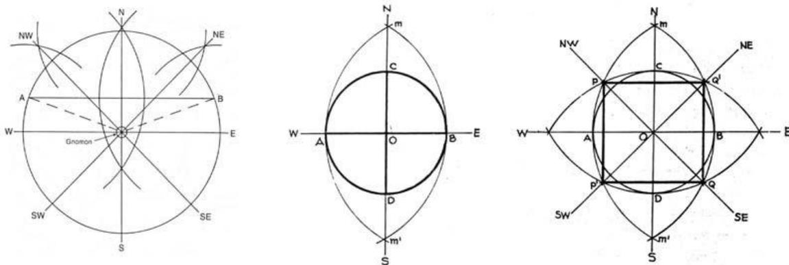
Figure 2.2- Traditional method of determining orientation (Dagens, 1994)
