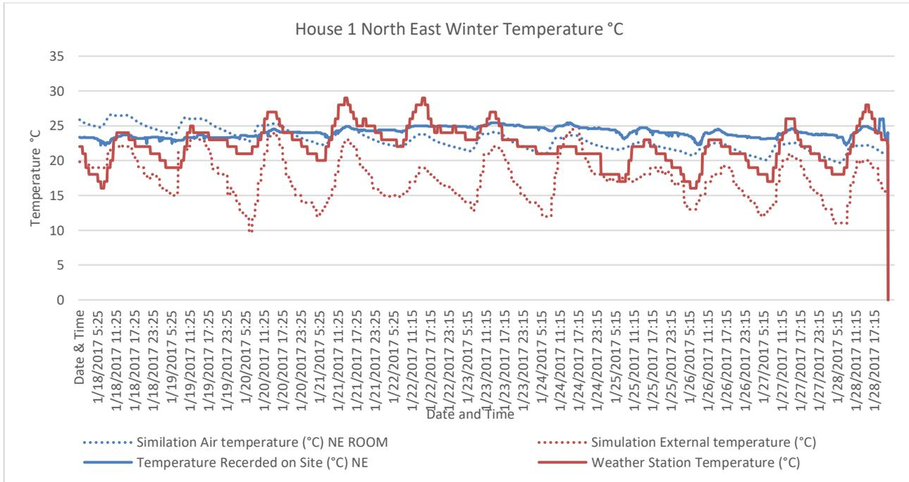
Figure 7.5 House 1 Simulation Temperature Comparison Winter – NE
