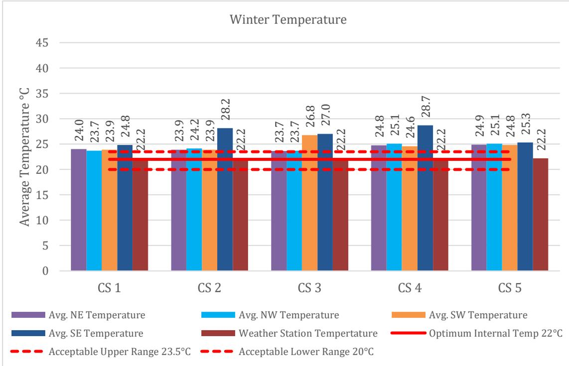
Figure 6.2- Comparison of Average Internal Temperature of Case Studies (CS) in Winter
