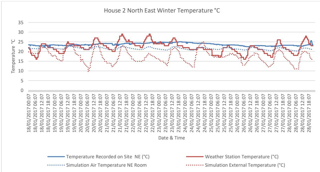
Figure 7.9 -House 2 Simulation Temperature Comparison Winter – NE
