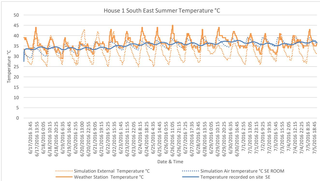
Figure 7.2 - House 1 Simulation Temperature Comparison Summer – SE
