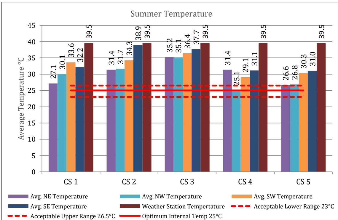
Figure 6.1- Comparison of Average Internal Temperature of Case Studies (CS) in Summer
