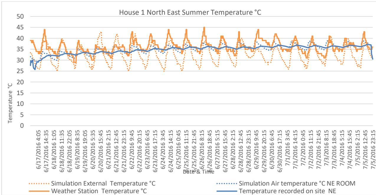
Figure 7.1 – House 1 Simulation Temperature Comparison Summer – NE
