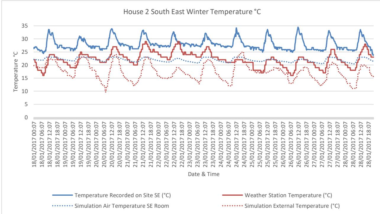
Figure 7.11 House 2- Simulation Temperature Comparison Winter – SE
