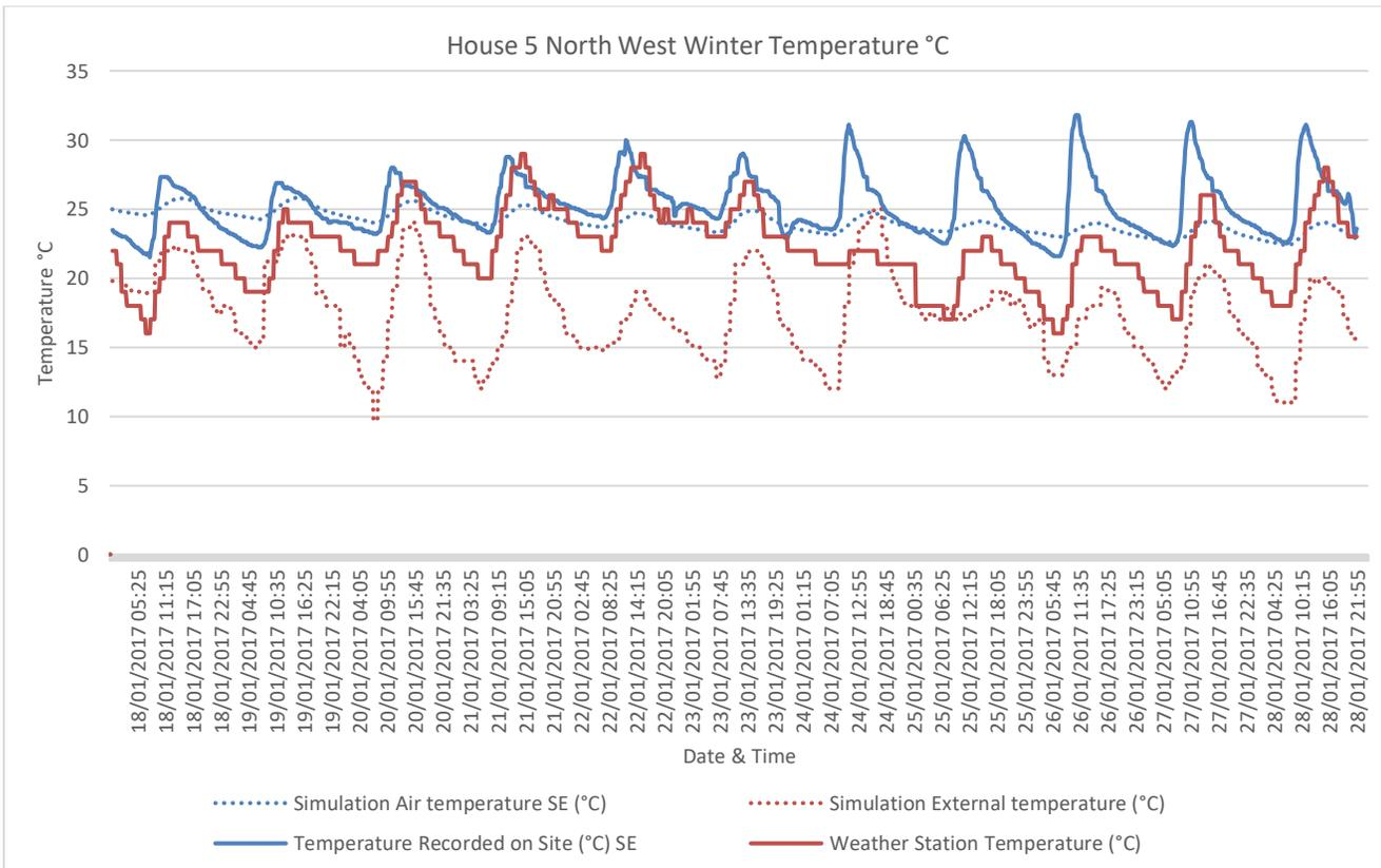
Figure 7.24 House 5 Simulation Temperature Comparison Winter – SE
