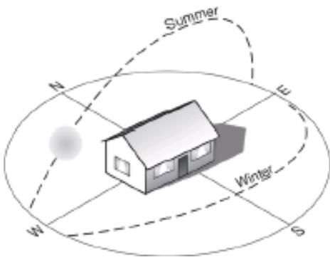
Figure 2.14- Preferred orientation for buildings in hot and humid climate (Anon., 2012)
