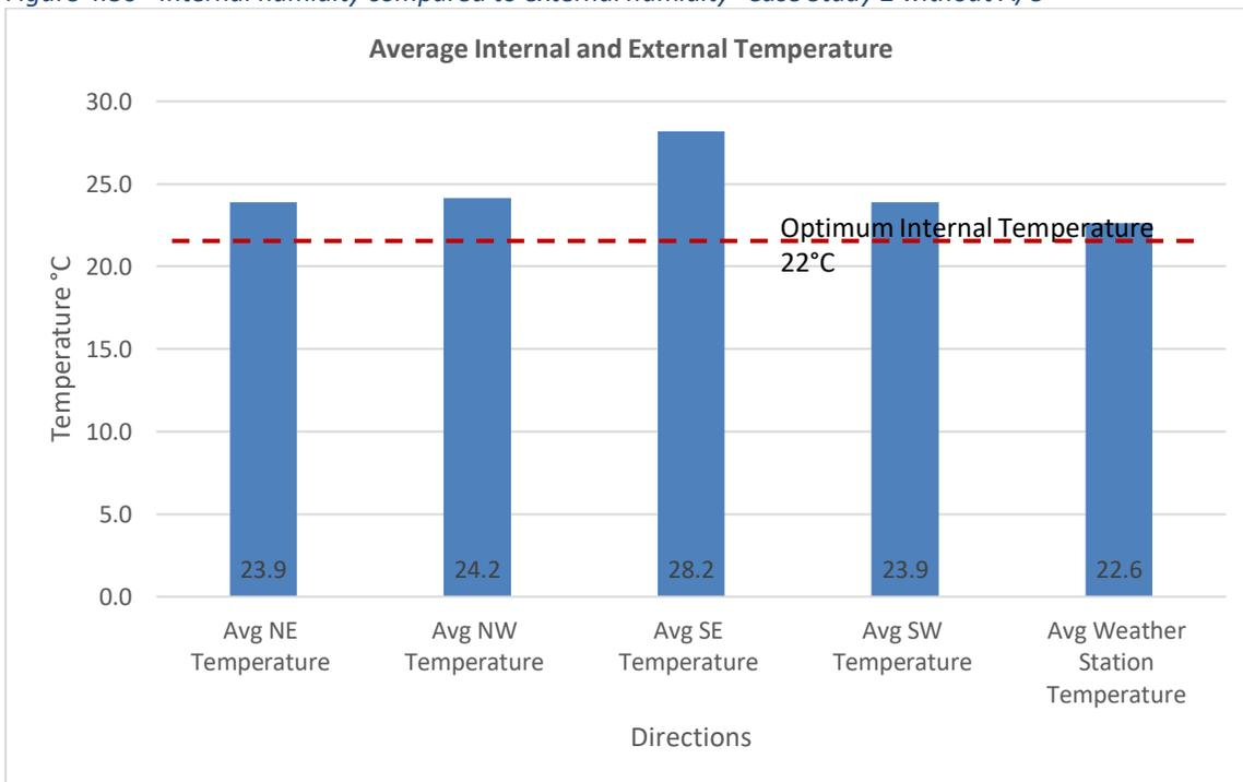
Figure 4.31- Average Internal and External Temperature - Case Study 2
