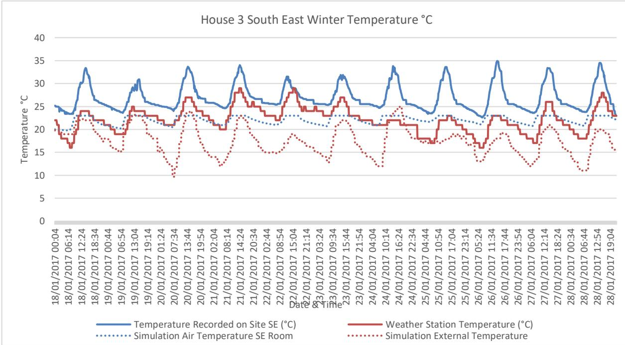
Figure 7.15 -House 3 Simulation Temperature Comparison Winter – SE
