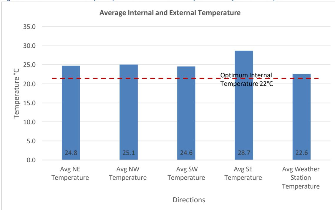
Figure 4.39 - Average Internal and External Temperature - Case Study 4
