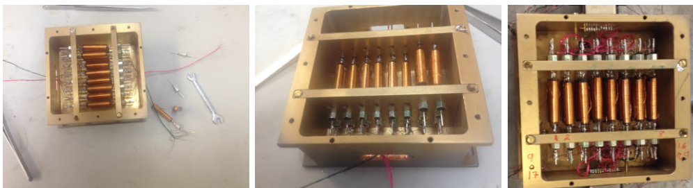
Figure 4.7: The appearance of filter box during and after implementing its elements inside it. The filter's components follow the circuit diagram given in Fig. 4.2.
