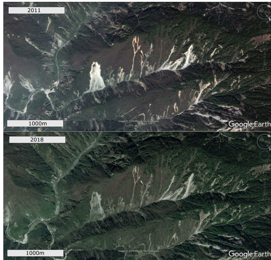
Figure 46 Satellite imagery of vegetation colonisation of areas affected by landsliding. Vegetation rapidly recolonises the bare sediment (white patches in the satellite image) following the earthquake. Growth of vegetation is a sign of stabilisation but remote sensing by itself cannot determine the root structure of the colonising vegetation which prevents estimation of any increase in cohesion.
