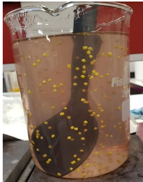
Figure 8.6: Suspension of plastic pellets in hydrogel solution.
