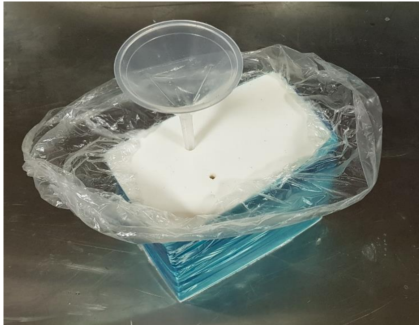
Figure 6.22: Assembled ventricle mould. Shown is the assembled silicone mould within a plastic bag that has been wrapped tightly to the mould with tape. A funnel has also been inserted into the mould to show how material is cast into it.
