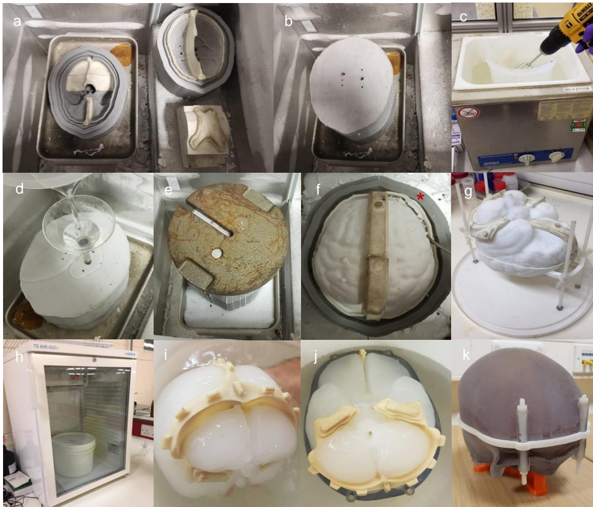
Figure 6.43: Casting, freezing and thawing of the hydrogel brain and assembly into the skull. a) assembled upper and lower mould halves and partially demoulded CO ventricle mould, all inside freezer; b) assembled mould in freezer, ready for casting; c) post-refrigeration agitation of hydrogel solution in ultrasound bath with whisking motion; d) casting of hydrogel into assembled brain mould; e) mould after 24 hour freezing with 20 kg weight on top; f) removal of top mould half after freezing and chiselling away of mould locating bands*; g) frozen brain with trapped inserts placed into thawing cap; h) frozen brain and thawing cap inside water bucket, placed inside incubator; i) defrosted brain with trapped inserts replaced with dural septa (bucket drained for photo); j) defrosted brain and dural septa positioned into the top skull half for oil extraction; k) assembled skull.
