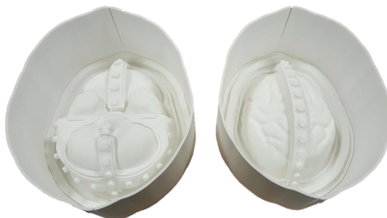
Figure 6.15: 3D printed top (right) and (left) bottom positive moulds.
