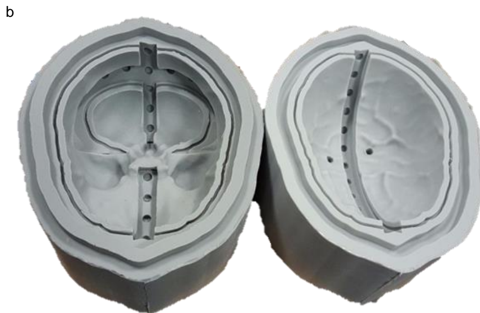
Figure 6.16: Casting of the expandable silicone halves. a) positive mould in vacuum caster; b) cast silicone top (right) and bottom (left) negative moulds.
