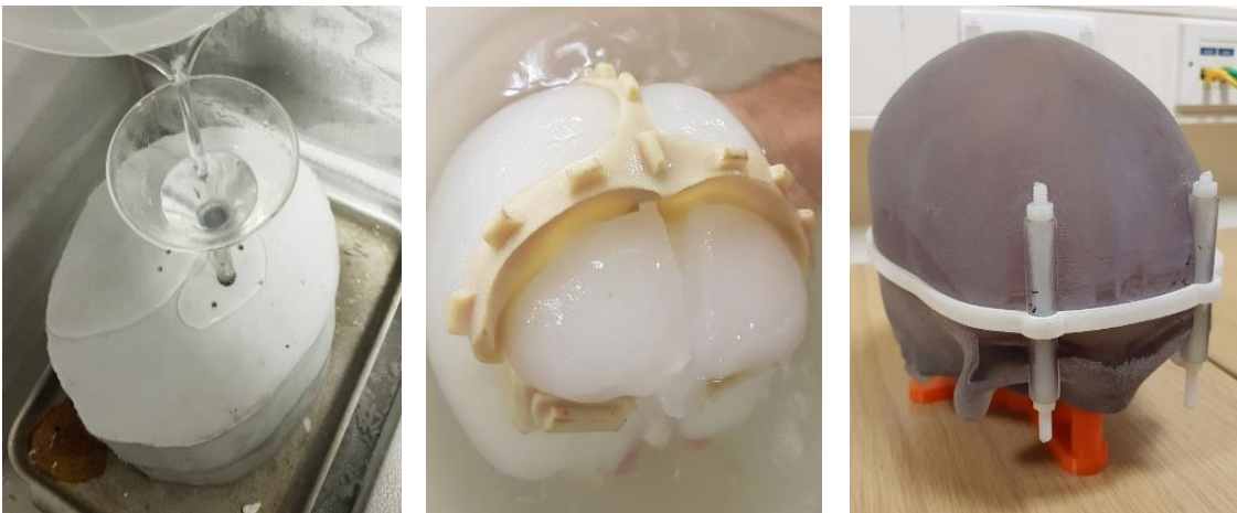
Figure 6.1: Chapter storyboard showing casting of the non-tethered model's brain with the composite brain mould (left), the non-tethered model's formed brain with dural septa (middle) and assembled non-tethered model (right). Images are reshown and discussed later in the chapter.
