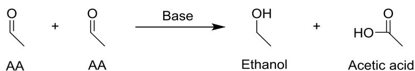
Scheme 4.3 Cannizzaro disproportionation of two AA molecules to form ethanol and acetic acid in the presence of a base
