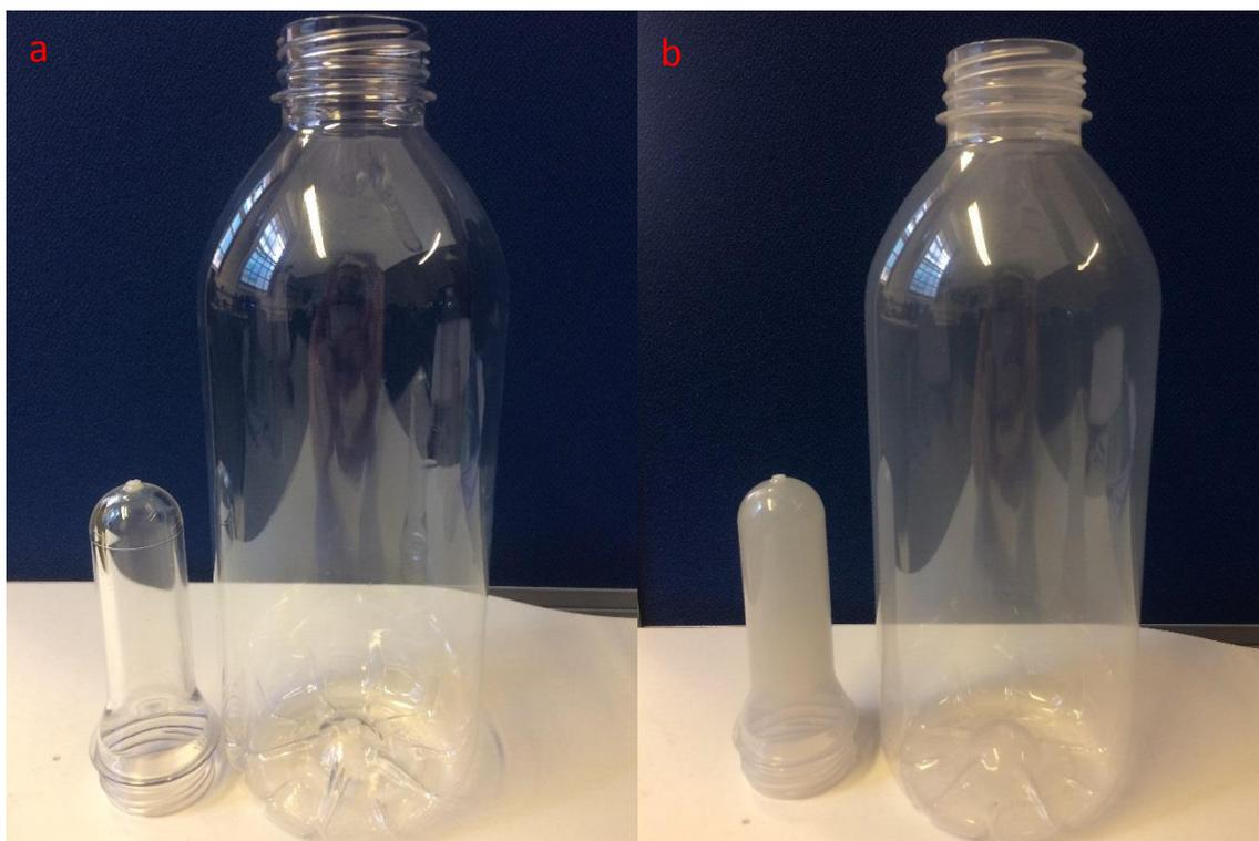
Figure 5.11 PET preform (left) and bottle (right): a = blank PET, b = PET loaded with 500 ppm  $\text{CeO}_2 \text{U}_3$  (25-75  $\mu\text{m}$  sieve fraction)
