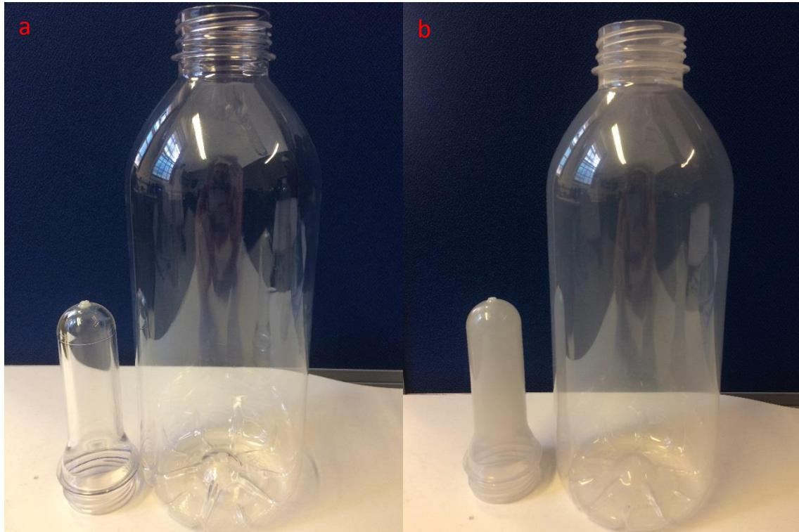
Figure 5.11 PET preform (left) and bottle (right): a = blank PET, b = PET loaded with 500 ppm CeO<sub>2</sub> U3 (25-75  $\mu\text{m}$  sieve fraction)
