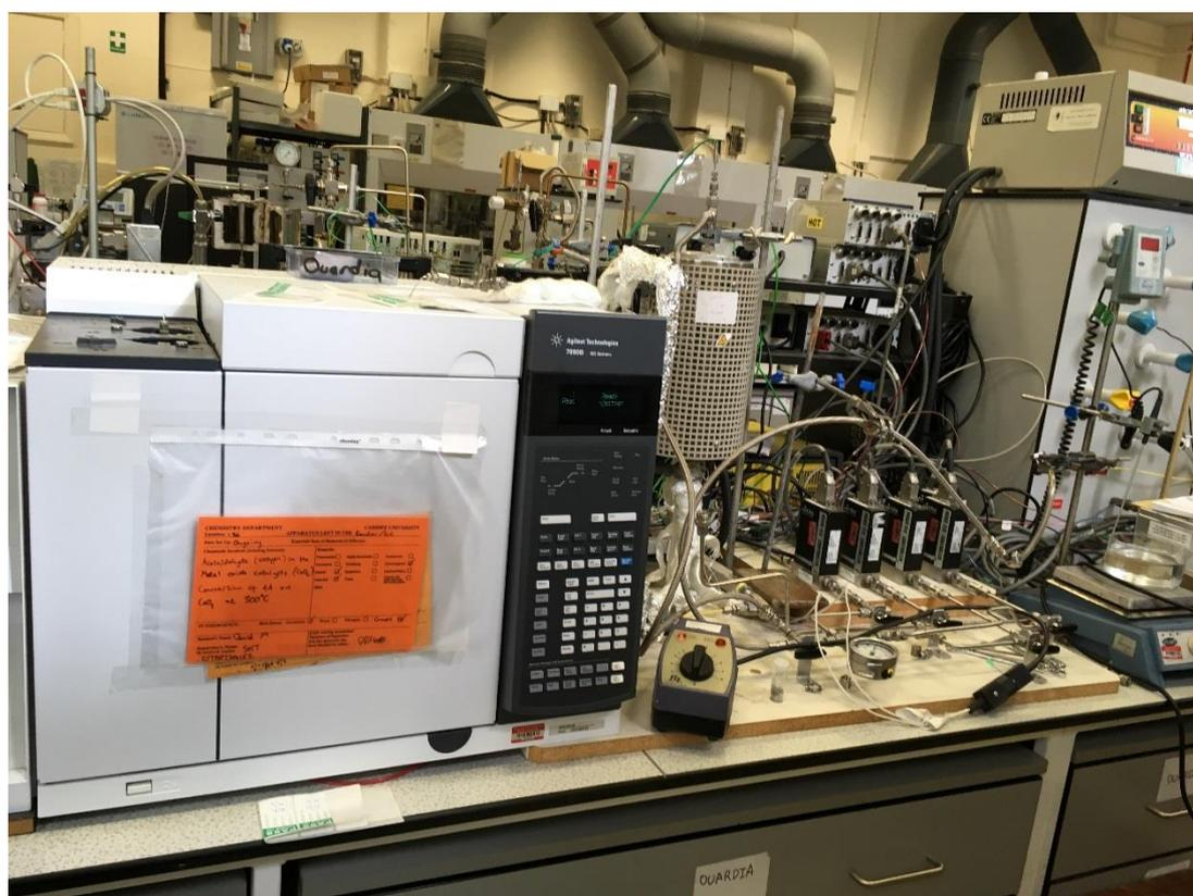
Figure 2.4 Photograph of continuous flow fixed-bed gas phase reactor with tubular furnace containing vertical reactor tube and online GC analysis
