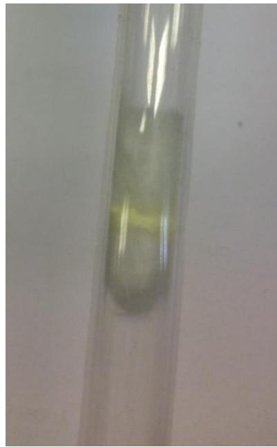
Figure 2.3 Photograph of ceria catalyst bed between quartz wool plugs within quartz reactor tube
