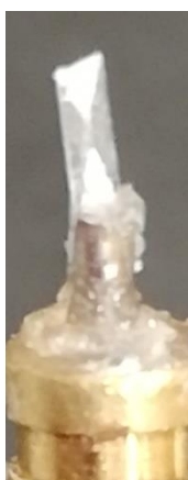
Figure 5.21 Image of the ‘hourglass’ shape that appeared on a single crystal of TBB.
