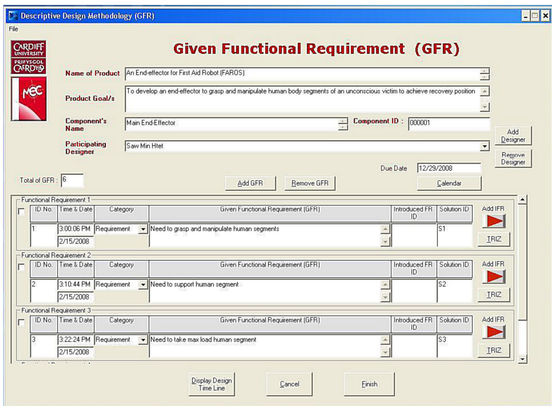
Figure 6.4 A snapshot of the modified text-based user interface of GFR for the descriptive design prototype tool that was integrated with the TRIZ-based ideation tool
