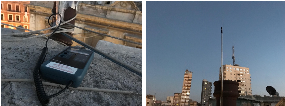
Figure 6-2 placement of hotwire anemometer over the roof
