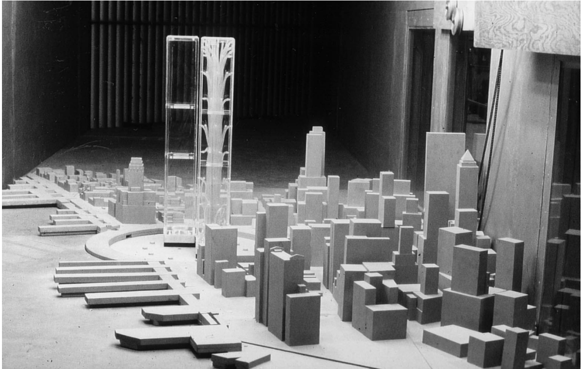
Figure 4-28 wind tunnel model of the new York trade center a study by Dr. J.E.Cermak and A.G.Davenport in the Colorado State (Plate, 1999).
