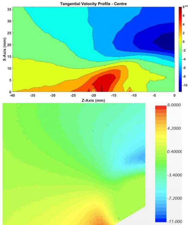
Figure 6 – Experimental (top) and numerical (bottom) profile of tangential velocity vector on the cross-sectional plane.
