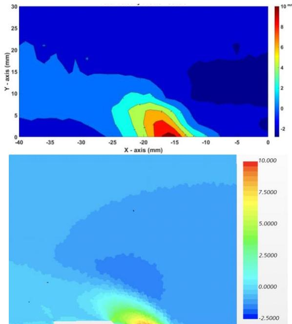
Figure 3 – Experimental (top) and numerical (bottom) profile of axial velocity vector on the axial plane
