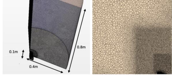
Figure 1 – generated mesh with computational domain and burner dimensions.
