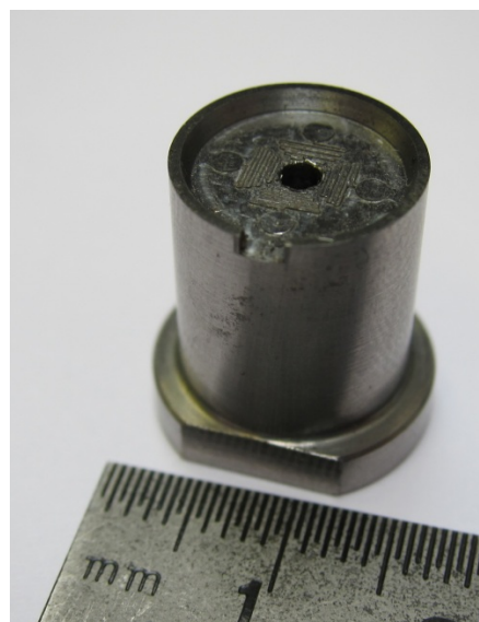
Figure 5-2 Steel mould insert incorporating test structures for microfluidic part and central bore hole for 2 mm ejector pin
