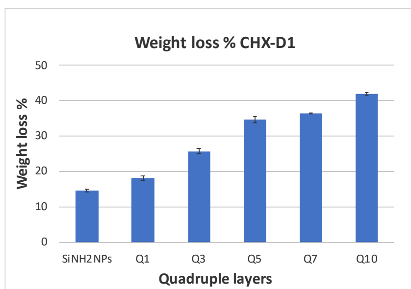
Figure 4.29b: Weight loss % among the QL for the matrix including CHX-D1. Mean ± SD (N=1, n=2).
