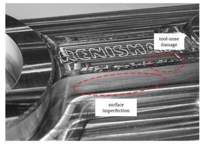
Figure 7.3. Outer-surface condition of the Con-Rod for arbitrary part (unknown cutting tool state)
