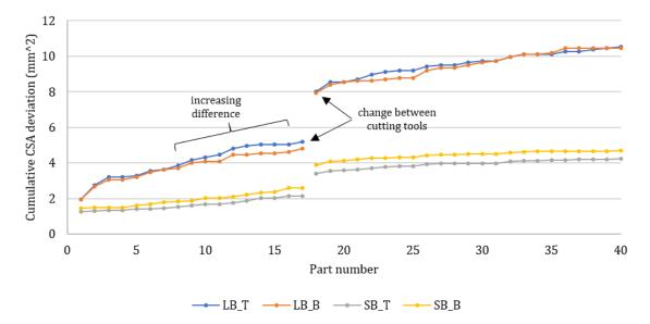
Figure 7.4. Cumulative CSAM deviation for 40 of the manufactured Con-Rods
