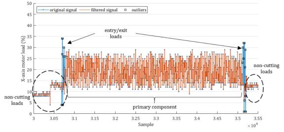
Figure 6.17. Single Slot signal components (SB004-1)
