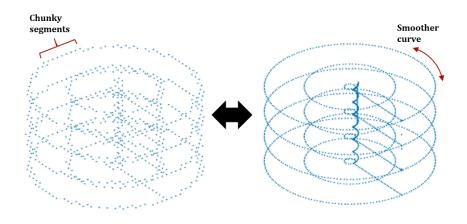
Figure 4.10. Comparison of XYZ before and after correction of byte processing (axes omitted)
