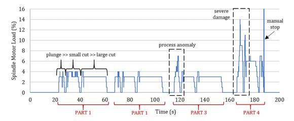
Figure 5.27. Single Cylinder spindle motor load for a 10mm cutting tool (with failure)
