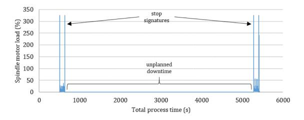
Figure 8.6. Evidence of stop signatures in the SML signal for abnormal MTData set
