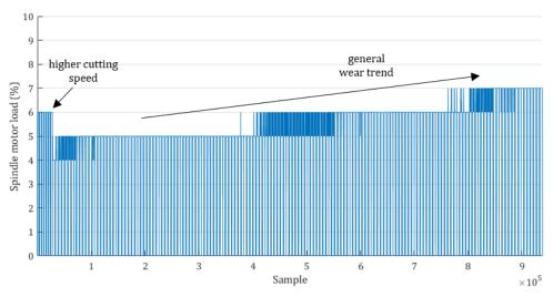
Figure 6.9. Raw SML signal for all 12mm Slots (SB003 and SB004026)
