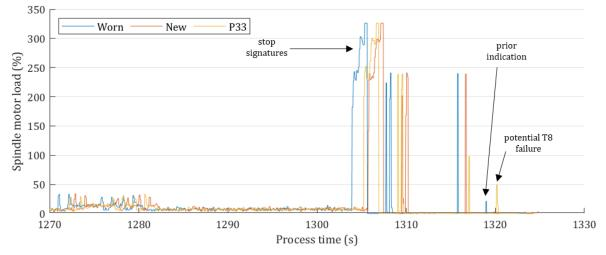
Figure 8.8. Final 60 seconds of the cutting process for T8 (possible cutting tool failure)
