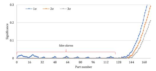
Figure 6.8. Upper QSUM moving average for SB peripheral wear, with 1, 2, and  $3\sigma$  thresholds
