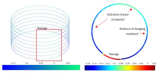
b. Single Cylinder (isometric view)c. Arbitrary, annotated, part (top view)Figure 5.14. Example 3D plots of geometry variation in the Cylinder applications
