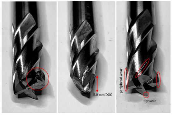
a. BUE b. Tooth shear c. Flank wear Figure 5.1. Observed cutting tool states following Cylinder application
