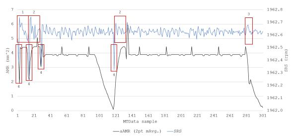
Figure B.14. Material removed per cut compared with the equivalent SRS
