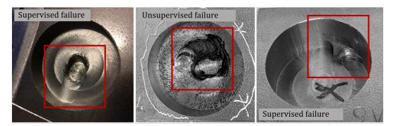
Figure B.1. Cutting tool failures for both minimum and maximum material removal
