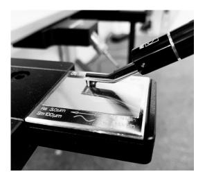
Figure 3.15. SFM-A2 acting on the  $3.0\mu m$  roughness specimen
