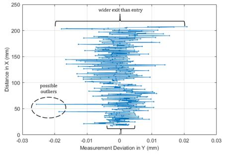
Figure 6.3. Surface waviness along Slot wall
