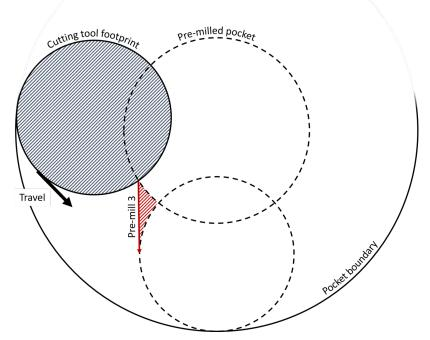
Figure B.8. Final pre-mill overlap for circular partial cut
