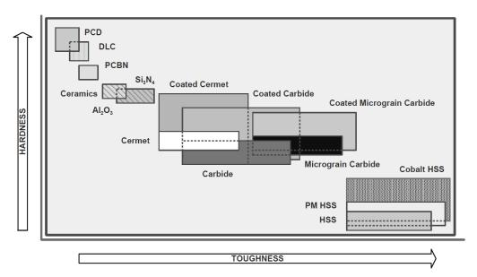
Figure 2.3. Material hardness versus toughness, reproduced from Astakhov and Davim (2008)
