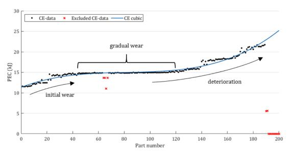
b. Cubic best-fit for CE PEC excluding process outliers Figure 5.32. PEC plots for CD and CE illustrating general trend
