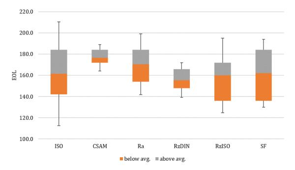
Figure 5.23. Box-plot comparison of the geometry and surface finish measures estimates for EOL
