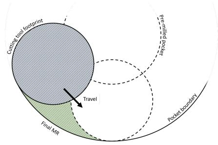
Figure B.10. Final region of metal to be removed during circular partial cut
