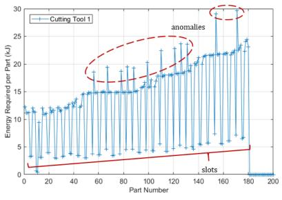
Figure 5.25. PEC for CD prior to Hampel filter
