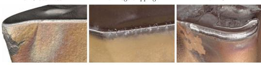
d. Plastic deformation e. Thermal cracking f. Abrasive flank wear Figure 2.4. Images of different wear mechanisms, reproduced from Sandvik Coromant (2020b)
