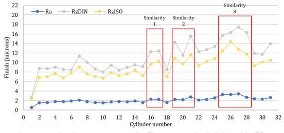
Figure 5.15. Roughness measurements for CD, comparing Ra, RzDIN, and RzISO
