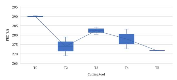
Figure 8.5. Spindle motor PEC results for the laboratory-made OMI-bodies
