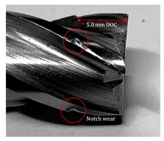
Figure 5.2. Flank and notch wear observed following Cylinder application
