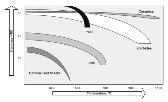
Figure 2.2. Material hardness versus temperature, reproduced from Astakhov and Davim (2008)
