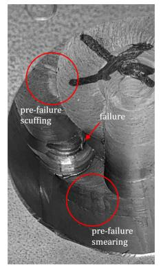
Figure 5.5. Cutting tool failure with minimal workpiece damage
