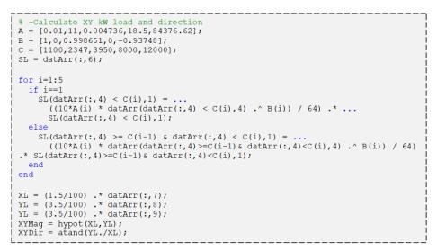
Figure 4.26. MATLAB script for implementing conversion of percentage load data
