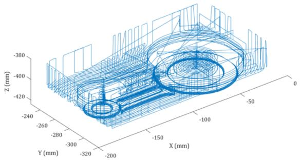
Figure 7.9. 3D process plot using axis position data (Con-Rod #2)
