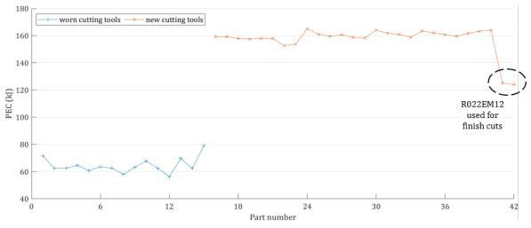
Figure 7.18. R021EM12 PEC per part for all 42 Con-Rods (one Con-Rod is one part)
