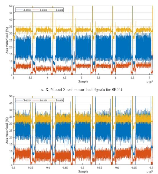
b. X, Y, and Z axis motor load signals for SB026
