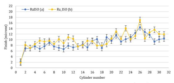
Figure 5.16. Comparing RzISO for each side of the slot wall (set CD)
