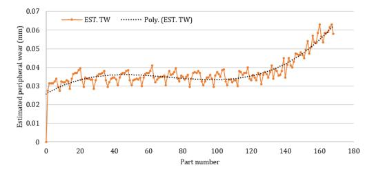
Figure 6.6. Estimated (average) peripheral edge wear based on the upper width of a 12mm Slot
