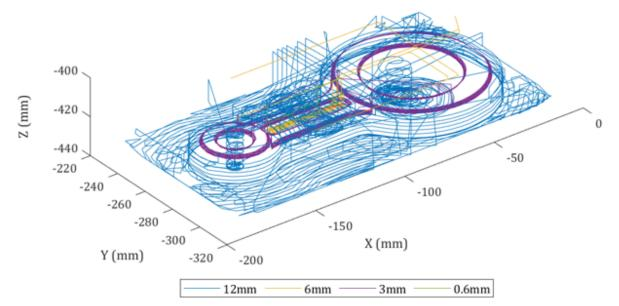
Figure 7.12. 3D process plot for optimised cutting process (Con-Rod #26)
