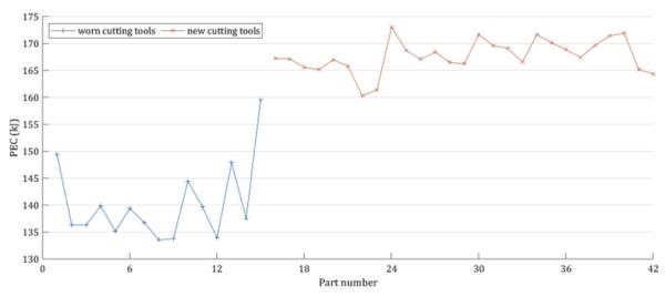
Figure 7.19. Combined PEC per part for all 42 Con-Rods (one Con-Rod is one part)
