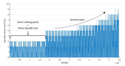
Figure 5.29. Unprocessed spindle motor load line plot for CD
