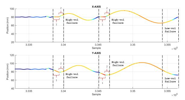
a. X and Y position plots indicating spindle load
