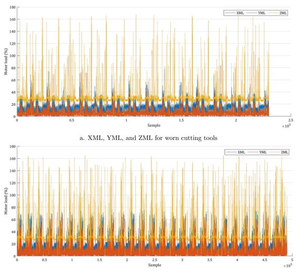
b. XML, YML, and ZML for new cutting tools
