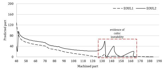
Figure 6.13. SB response plot for PEC e-fit predictions of cutting tool condition
