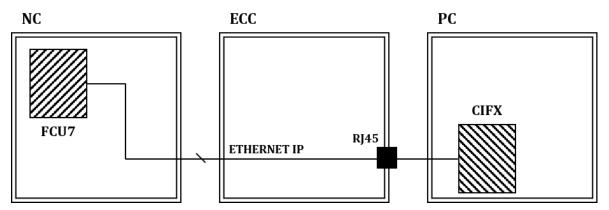
Figure 3.4. Basic wiring schematic for COMX-CIFX physical connection
