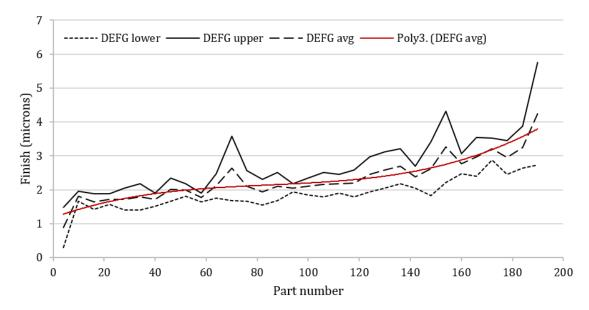
Figure 5.17. Surface finish envelope plot for CD, CE, CF and CG, showing the combined average trend
