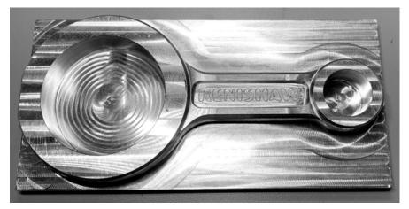
Figure 7.1. Photograph of the Con-Rod application
