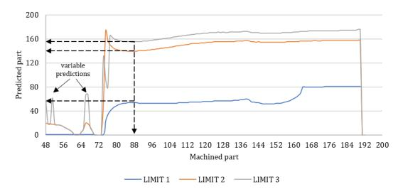
Figure 5.39. CE response plot for PEC e-fit predictions of cutting tool condition
