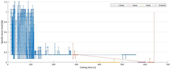
Figure 7.17. SML for arbitrary Con-Rod, separating different cutting tools
