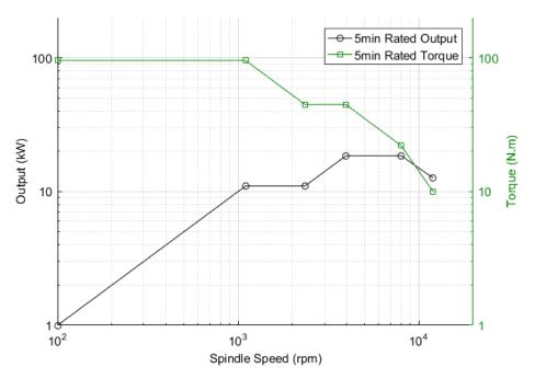
Figure 4.25. Spindle speed-power-torque characteristic, recreated from Yamazaki Mazak (2015b)
