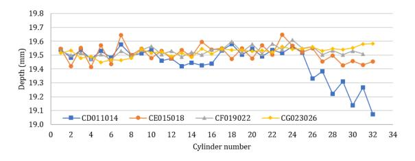
Figure 5.8. Comparison of depth measurements from four tests
