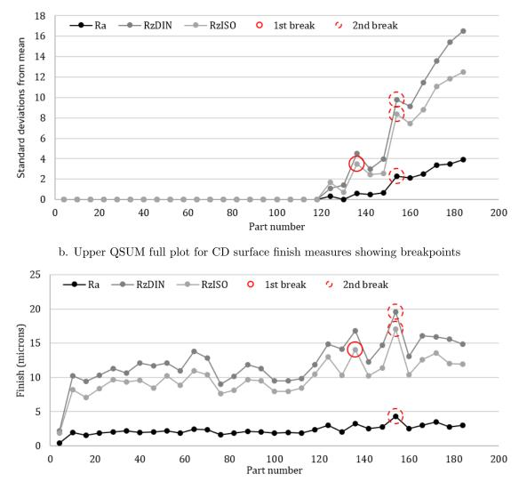
c. Roughness measurements for CD, comparing QSUM breakpoints for Ra, RzDIN, and RzISO Figure 5.19. QSUM investigation for CD surface finish trends
