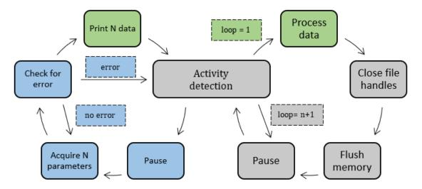
Figure 4.2. Process logic illustrating activity detection (grey), DAQ (blue) and processing (green)
