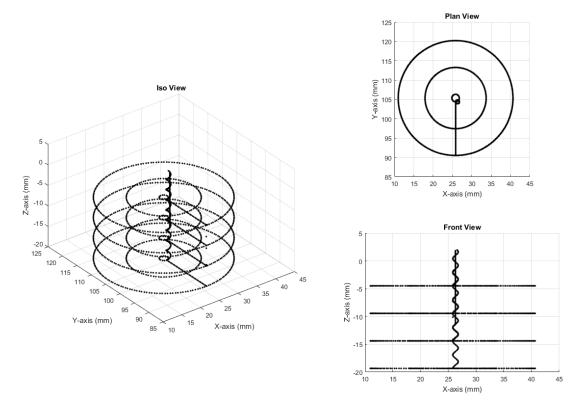
Figure 5.53. 3D process visualisation compiled using in-process axis position data
