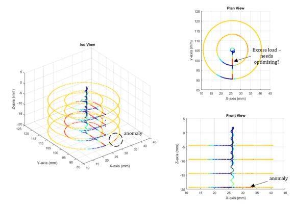
Figure 5.54. 3D process visualisation illustrating feature quality using SML overlay
