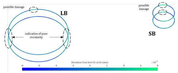
Figure 7.6. Scanned measurements for arbitrary Con-Rod indicating point-to-point variation
