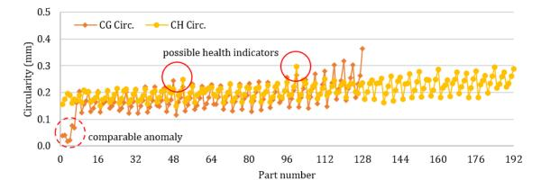
b. Cylinder circularity (target 0.1mm)
