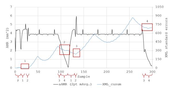
Figure B.19. Cumulative sum for X-axis percentage load compared with material removal during wear test
