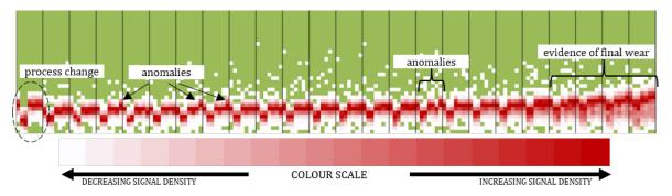
Figure 6.21. YML dispersion heat map for all 12mm Slots
