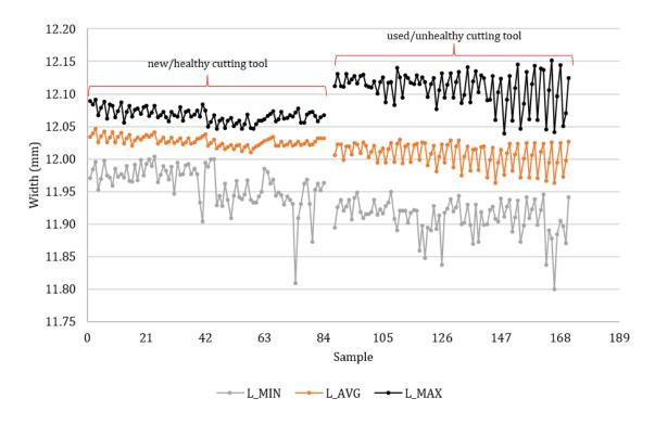
a. Width measurements for top, middle, and bottom scan pairs (concatenated)
