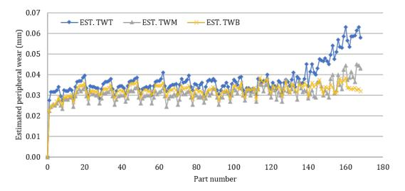
Figure 6.5. Estimated (average) peripheral edge wear based on a 12mm Slot width
