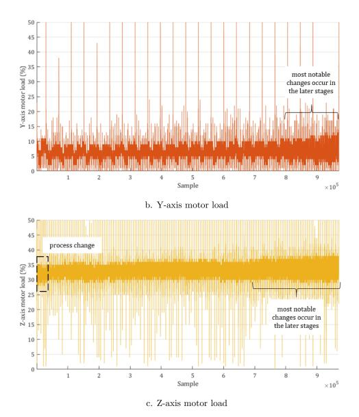
Figure 6.15. Percentage axis motor load signals for SB (including SB003)
