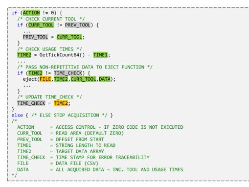
Figure 4.7. Pseudo code illustrating time-specific data filtering
