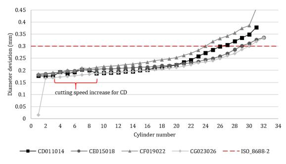
Figure 5.10. Diameter deviation for four tests considering an appropriate upper threshold
