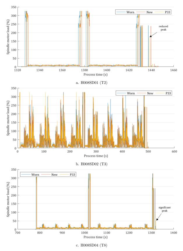
Figure 8.7. SML plot to compare worn and new cutting tools with a potential breakage
