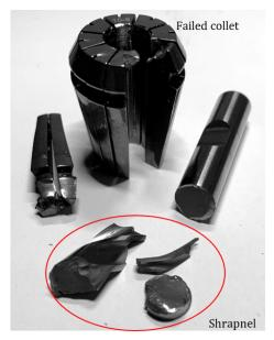
Figure 5.3. Disintegrated tool (catastrophic failure)
