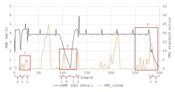
Figure B.20. Cumulative sum for Y-axis percentage load compared with material removal during wear test
