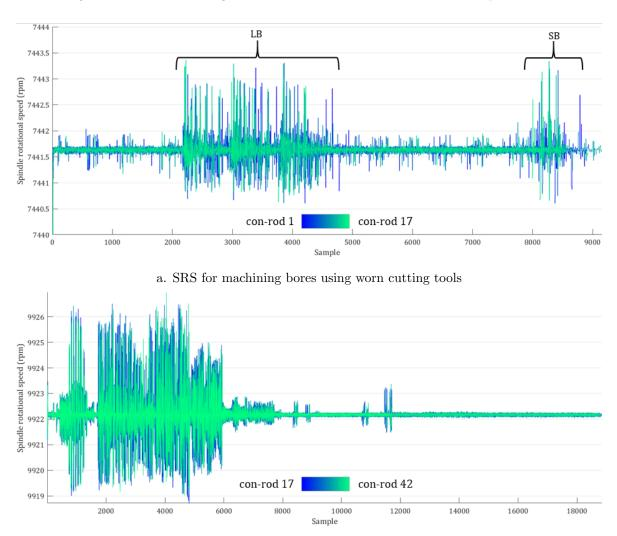
b. SRS for machining [entire] Con-Rod using new cutting tools
