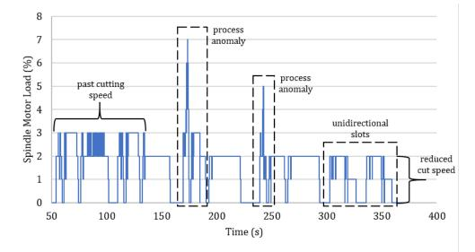
Figure 5.28. Single Cylinder spindle motor load for an arbitrary 10mm cutting tool (no failure)
