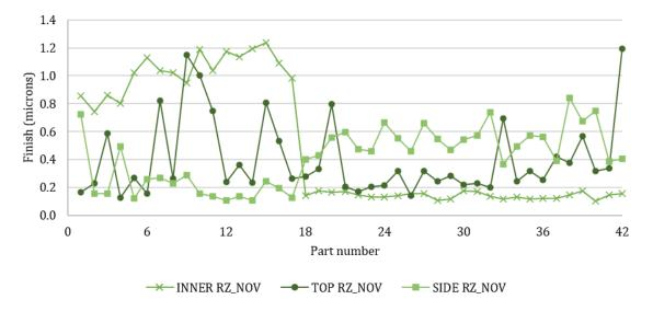
Figure 7.5. RzNOV surface finish measurements for the inner, top, and side of all 42 Con-Rods
