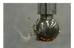
Figure 3.14. Collected probe debris after scanning measurement
