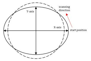
Figure 7.8. Exaggerated geometry of the Con-Rod large bore
