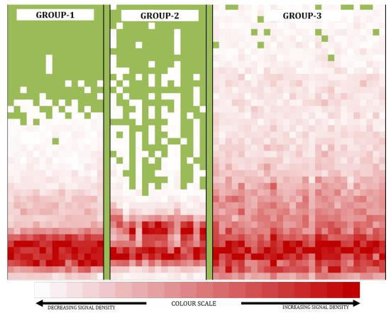
Figure 7.23. YML dispersion heat map for all 42 Con-Rods (R021EM12 only)
