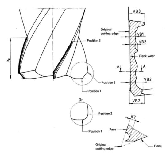
Figure 2.5. Indications of flank wear, reproduced from ISO 8688-2:1989
