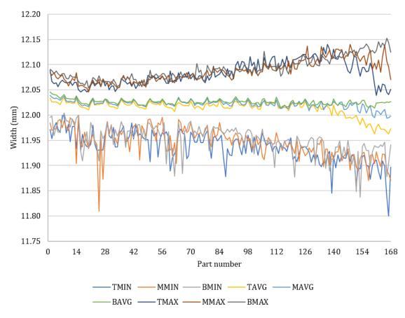
b. Width measurements for top, middle, and bottom scan pairs (separated)Figure 6.4. Min, avg, and max scanned width measurements for SB (inc. SB003)
