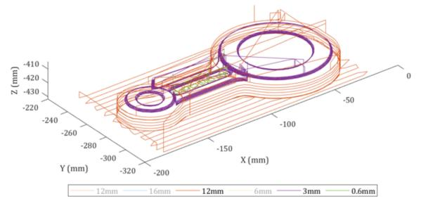
b. Finishing cuts for example Con-Rod
