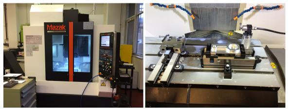
b. Mazak front exterior c. Mazak table area Figure 3.2. Mazak Vertical Centre Smart 430A VMC
