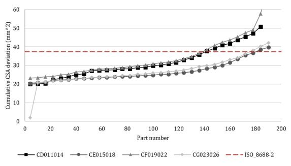
b. Accumulative variation in part cross-section relative to previous parts
