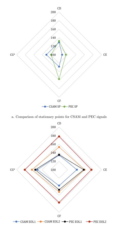
b. Comparison of EOL estimates for CSAM and PEC signals Figure 5.43. CSAM and PEC inflection comparison using radar plot for CD, CE, CF, and CG
