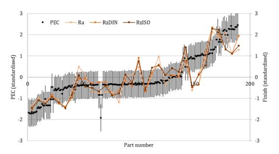
Figure 5.42. Standardised comparison of CE PEC (with uncertainty) and surface finish trends
