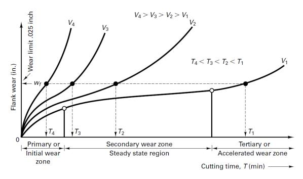
Figure 2.6. Cutting tool flank wear curves, reproduced from Black and Kohser (2012 p594)
