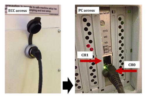
Figure 3.5. MT and PC backend connections
