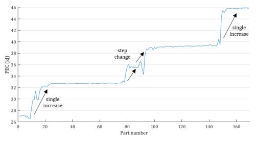
Figure 6.10. PEC trend for all completed 12mm Slots
