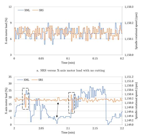
b. SRS versus X-axis motor load during cutting
