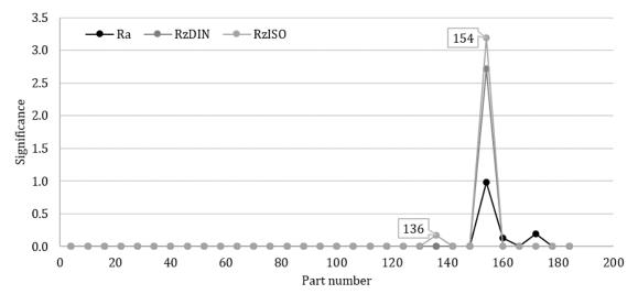
a. Upper QSUM breakpoints for CD surface finish measures with  $3\sigma$  threshold
