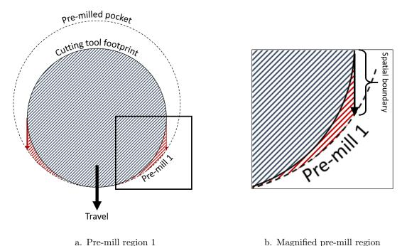
Figure B.4. Pre-mill overlap during first slotting cut
