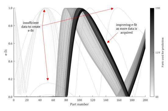
Figure 5.38. CE PEC predicted e-fit curves from 48-190 parts
