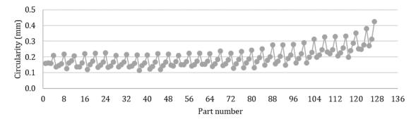
c. Cylinder circularity (tolerance 0.1mm) Figure 5.7. Trends in form measurements for CD
