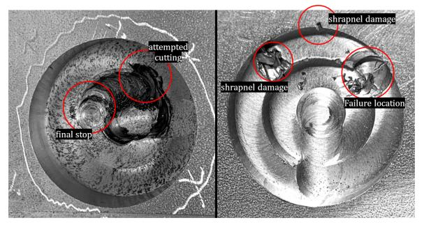
Figure 5.4. Irreparably damaged Cylinders due to catastrophic cutting tool failures
