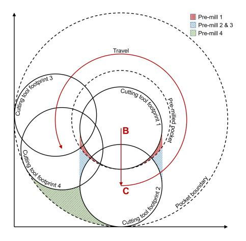
Figure B.3. Pre-mill occurrences for 10mm Cylinder wear tests (inner pocket)
