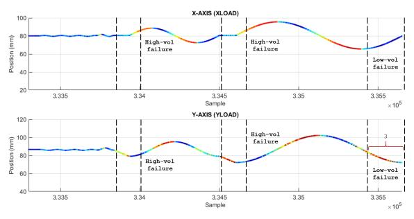
b. X and Y position plot indicating specific axis load
