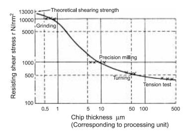
Figure 2.8. Chip thickness versus shear stress - reproduced from Taniguchi (1994), from Shaw (2003)
