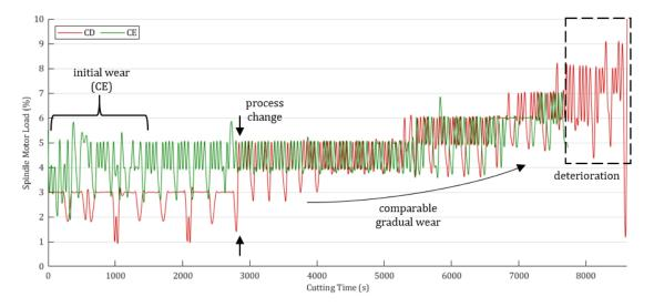
Figure 5.31. SML upper peak envelope with 900pt separation for CD and CE
