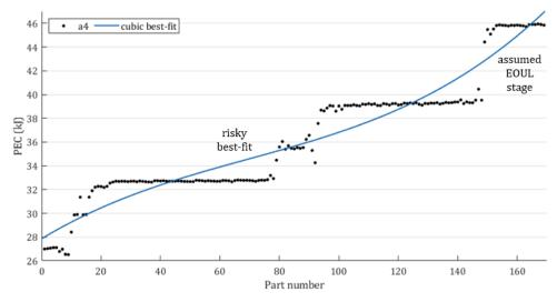
Figure 6.11. PEC trend with cubic best-fit for 12mm Slots (SB)
