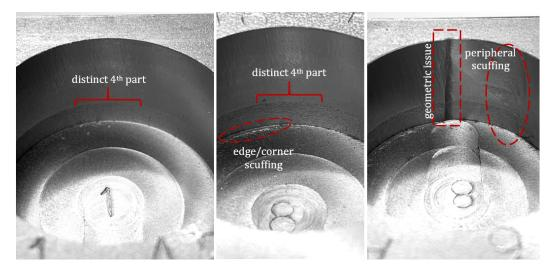
Figure 5.6. Qualitative analysis of Cylinder condition at stages in the cutting process
