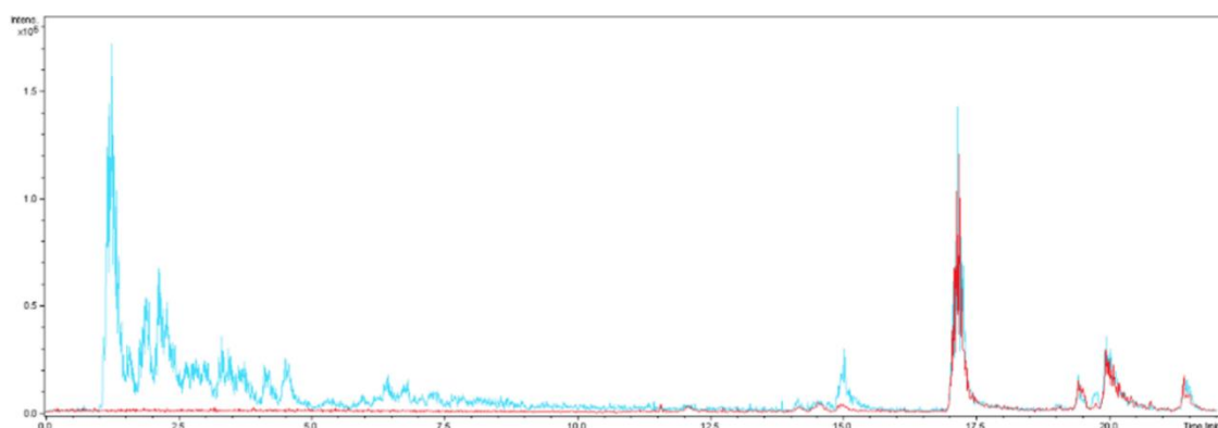
Figure 14. LC-MS chromatogram corresponding to the post reaction solution of a reaction run over MgO for 6 h. Detection parameters are fixed at 100 - 1000 m/z. Reaction conditions; 400 °C, glycerol flow (0.016 mL min -1 ), 0.5 g MgO, 50 mL min -1 Ar, 3 hours. Blue line – chromatogram of the post reaction solution. Red line – chromatogram of a H 2 O blank solution.
