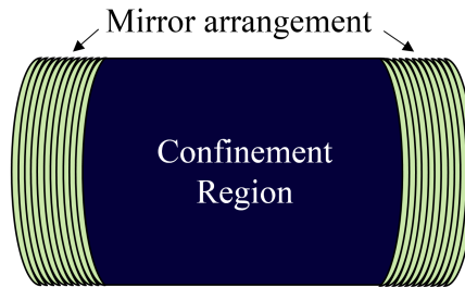
Figure 1.2: Optical cavity diagram. mirrors (green) confine light into a small region (blue).
