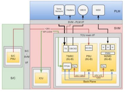
Figure 4-22: TCU block diagram and electrical I/F
