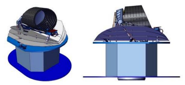
Figure 5-4: Illustrative representation of the Ariel S/C from two angles, composed of the Consortium provided PLM, and a generic dummy SVM. An upwards tilt (5°) can be seen on the right picture between the telescope pointing axis and the SVM "horizontal" XY plane. This means the accessible sky described in Figure 3-19 is a 50° wide annulus region near orthogonal to the ecliptic plane ( $-20^{\circ}/+30^{\circ}$ )
