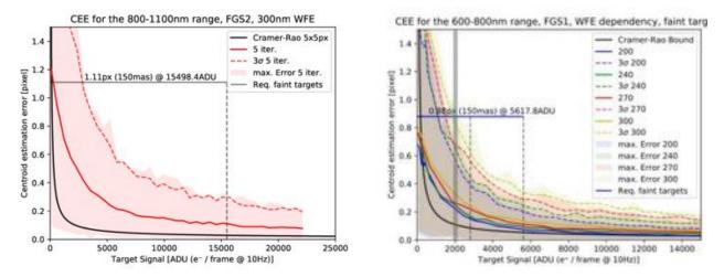
Figure 4-15: Centroiding accuracy estimates for faintest target in nominal FGS2 channel (left) and back-up FGS1 channel (right). Note the simulations shown in different colours for the FGS1 case are for different WFE levels showing that even with 300nm WFE (vs derived requirement of 270nm on the combined TA, CO & FGS systems) the centroiding requirement is met.
