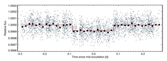
Figure 7-7: Corrected and phase-folded CHEOPS occultation light curve of WASP-189 b. Black points show the light curve binned into 20-minute intervals and the red line shows the final occultation model (Lendl et al. 2020).
