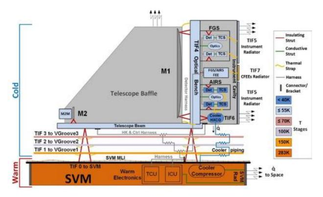
Figure 4-18: PLM Thermal Architecture Scheme
