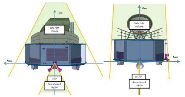
Figure 5-1: Ariel nominal cut angles and PLM shading (illustrative, not to scale). Left:  $\pm 30^{\circ}$  around Y. Right:  $\pm 6.75^{\circ}$  around X. In addition to the 360° slew capability around Z, this provides access to over 40% of the sky at any given time (requirement  $\geq 30\%$ ). Note that these cut angles include margin to accommodate for FDIR aspects. The resulting angular range that can be used for science observations is therefore a bit smaller.
