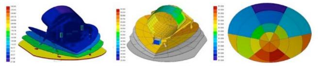
Figure 4-19: Thermal map of hot case temperatures of (from left to right) the whole PLM, the coldest part of the telescope assembly, the M1 mirror surface – note that the colour scales are different in each view.
