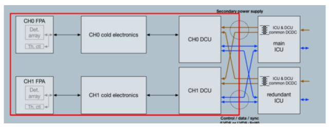
Figure 4-8: Overview of AIRS electrical system. Red line delineates AIRS instrument boundaries.
