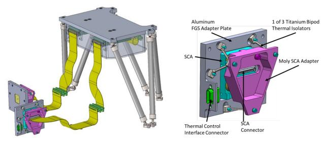
*Figure 4-13: Conceptual design of the FGS detector system. Right – FPE (housing CFEE SIDECAR ASICs operating at ~130K, with cryo-flex harnesses running to detector modules. Right – Focal Plane Module (FPM) design*
