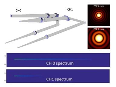
Figure 4-6: Detailed Optimized folded Zemax implementation of Channel 0 and Channel 1 spectrometer. The windows on the detector needed for the spectra are  $325 \times 64$  pixels in Ch0 and 120 x 64 pixels in Ch1 where the spatial direct size is set by the need to monitor the background and dark current of the detector. The PSFs are shown for Ch0 for a region of 10x10 pixels.
