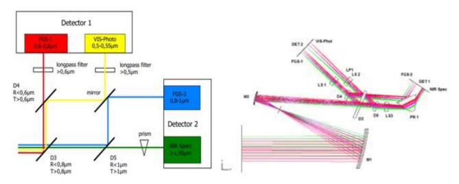
Figure 4-10: Left: Dichroic schematic showing how channels are split. Right: Baseline optical layout for FGS.
