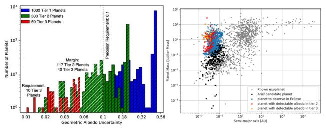
Figure 3-7: Left: Simulations from Zellem et al. (2019): Ariel could measure exoplanetary geometric albedos with high precision. Right: simulations done with Ariel Rad (Mugnai et al 2020) showing the fraction of planets observed in Tier 2 and Tier 3 mode for which the albedo is detectable very precisely, assuming the albedo is = 0.5. This fraction reduces to one half and one quarter if the albedo is = 0.3 and 0.1 respectively.
