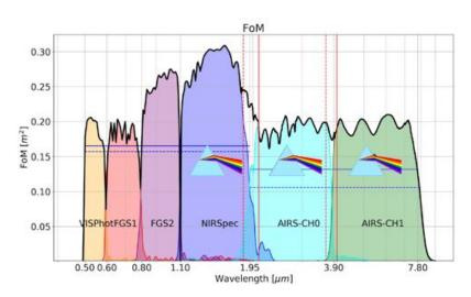
Figure 4-2: End-to-end Figure of Merit for the payload channels. The derived requirement from the PRD is also shown, the solid line is the required band average and the dotted line is the minimum allowable at any point in the band.
