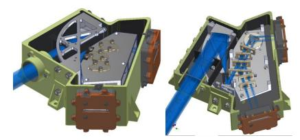
Figure 4-12: FGS Optical Module mechanical design with lid removed (left) and in cross section view (right)
