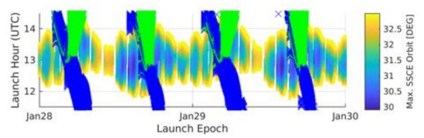
Figure 5-2: Example launch window for a direct transfer to L2 provided by ESOC (to be confirmed by Arianespace). Similar results are valid for any launch year. The colour scale indicates the resulting Sun-S/C-Earth (SSCE) angle in L2 as a function of the launch time. Launches resulting in eclipses during the transfer to L2 and during the nominal operations phase are crossed-out.
