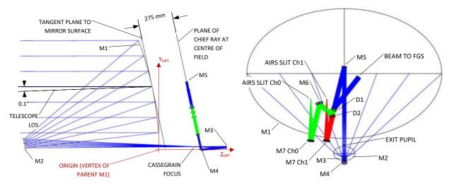
Figure 4-3: Scale drawings of the telescope and common optics. (Left): view in YOPT-ZOPT plane. The 0.1° offset is exaggerated for clarity. (Right) view in XOPT-YOPT plane.
