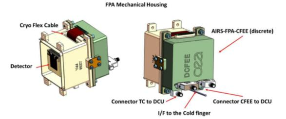
Figure 4-9: Design of the AIRS Focal Plane Assembly with the detailed units (one FPA per channel). Note that the green box housing the CFEE is only installed in the case of the Discrete CFEE solution; in case of the SIDECAR ASIC option these are housed in a separate enclosure outside the payload instrument cavity (as shown in Figure 4-20).
