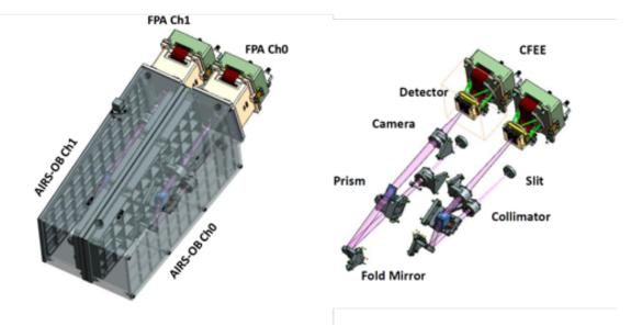
Figure 4-7: Implementation of AIRS optical design within the allocated volume. The size of the AIRS OB volume is 482  $\times$  206  $\times$  184 mm; the optical interface is at the slits which are 40 mm above the mounting plane and separated by ~108 mm for the two channels.
