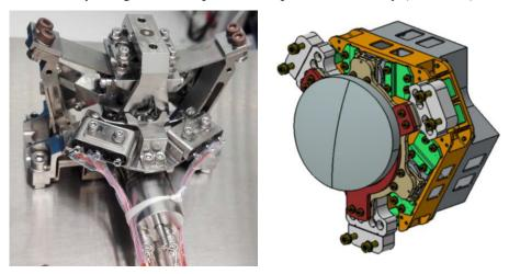
Figure 4-4: (Left) M2M actuator developed for Ariel TDA. (Right) Ariel M2M preliminary design from phase B1.
