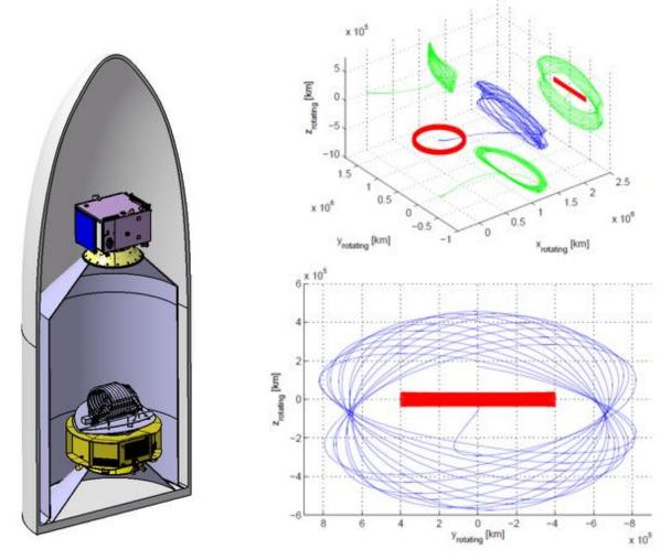
Figure 5-3: Left: illustration of the Ariel S/C in the lower position inside the A62 dual launch fairing (Comet-Interceptor sits in the top position). Right: example of the Ariel quasi-halo orbit around L2 and how eclipses are avoided. Blue shows the 3D trajectory, while green shows the projections in the rotating frame. Red indicates the Moon and its projection in the YZ plane of the rotating frame.
