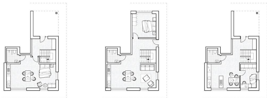
Figure 4.5b: a series of iterations (ground floor above, first floor below) demonstrate the adaptability of the plan, in particular with regard to the provision of lifetime homes.
