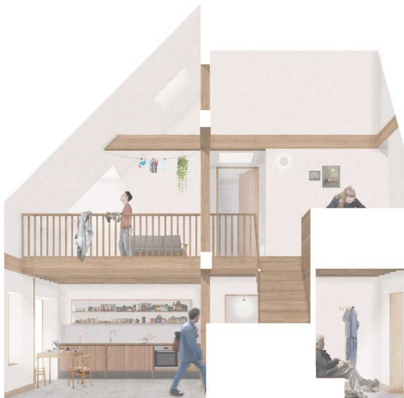
Figure 4.5d: an interior section looking towards the kitchen and service core. A double height space connects living spaces with central circulation.
