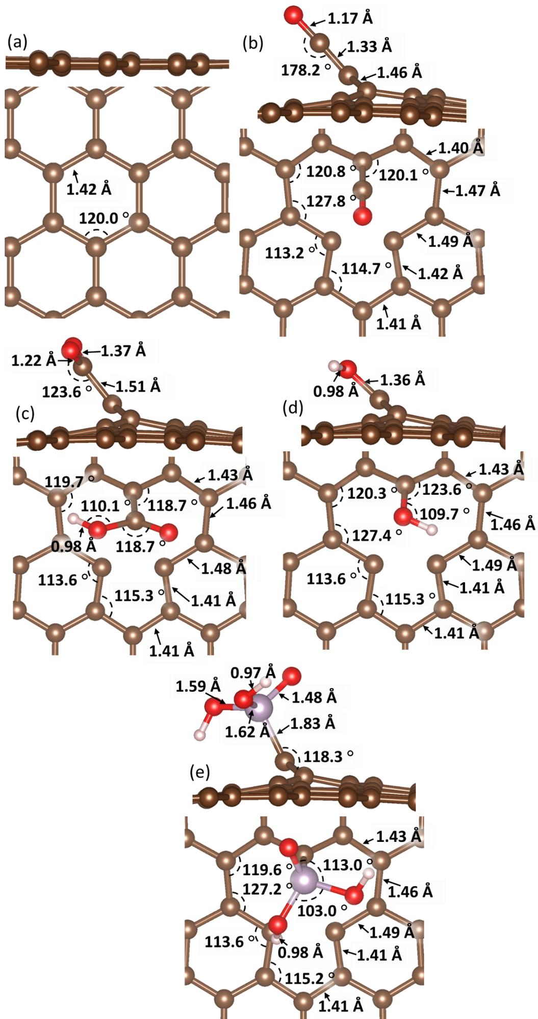
Figure 5: Side and top views of the optimized surfaces a) pristine graphene (PG), b) carbonyl doped SV graphene (G\_CO), c) carboxyl doped SV graphene (G\_COOH), d) hydroxyl doped SV graphene (G\_OH) and e) phosphate doped SV graphene (G\_PO<sub>3</sub>H). Inset shows the distances (Å) and angles (°) of interest. Carbon atoms are represented in brown, oxygen in red, hydrogen in white and phosphorous in violet.
