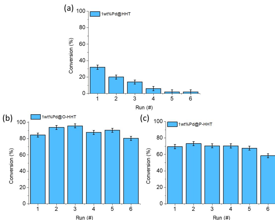
Figure 4: recycling tests of a) Pd@HHT, b) Pd@O-HHT and c) Pd@P-HHT for formic acid dehydrogenation
