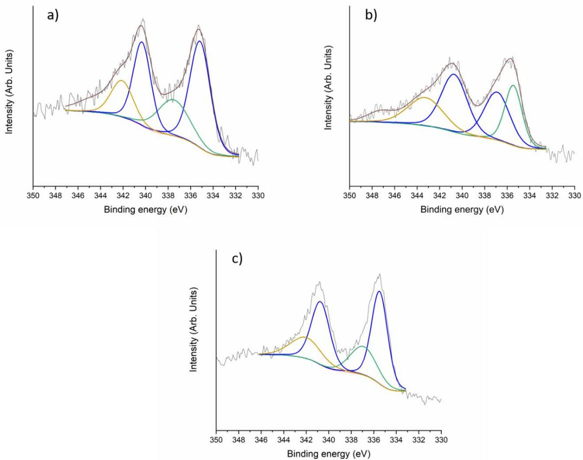
Figure S1: XPS Pd 3d spectra for a) Pd-HHT, b) Pd@O-HHT and c) Pd@P-HHT
