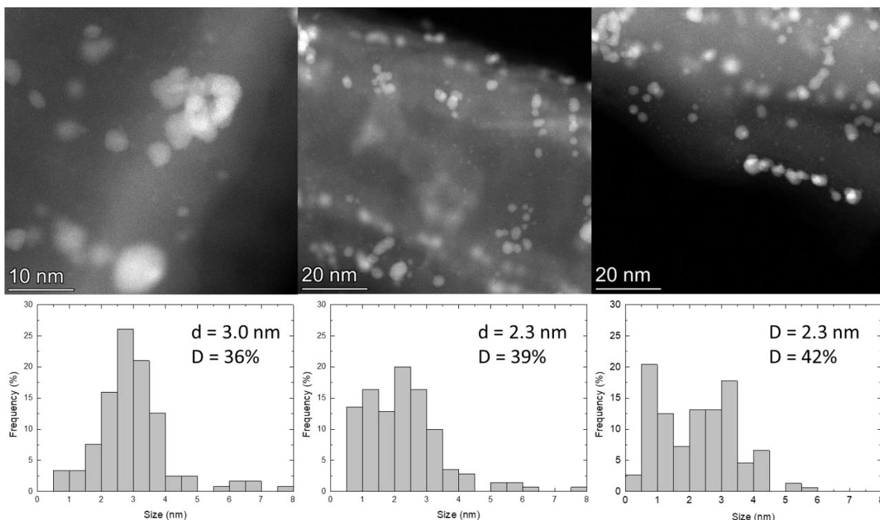
Figure 1: Representative HR-STEM images (top) and particle size distribution (bottom) of 1wt%Pd@HHT (left) 1wt%Pd@O-HHT (middle) and 1wt%Pd@P-HHT (right).
