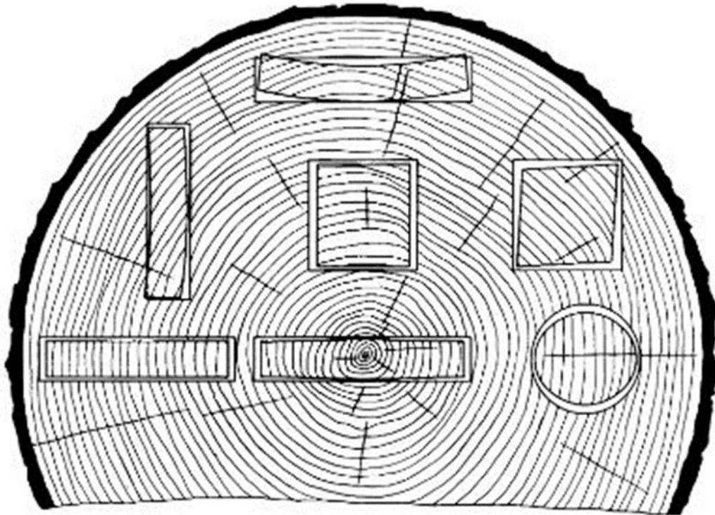
**Figure 54: Results caused by differences in tangential and radial shrinkage (Simpson 2001).**
