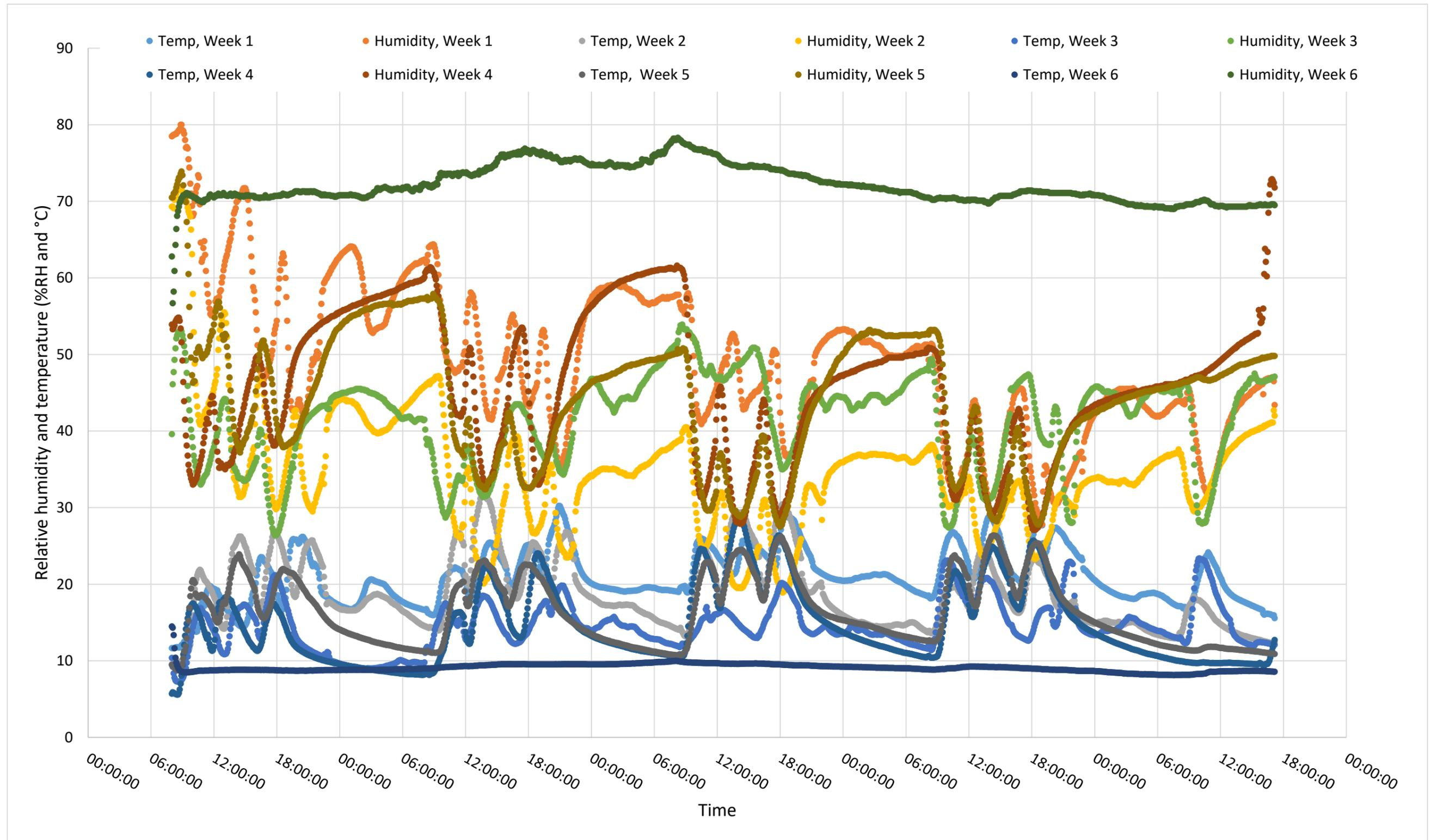
Figure 138: Data from logger E2 (room centre) for heating experiments. Week 1-3 banked in, week 4-5 daily fires, Experiment 6 unheated.
