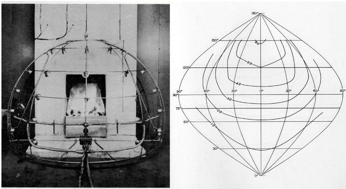
**Figure 132: Distribution of radiation from inset open-fire (Venables 1957a; Venables 1957b).**
