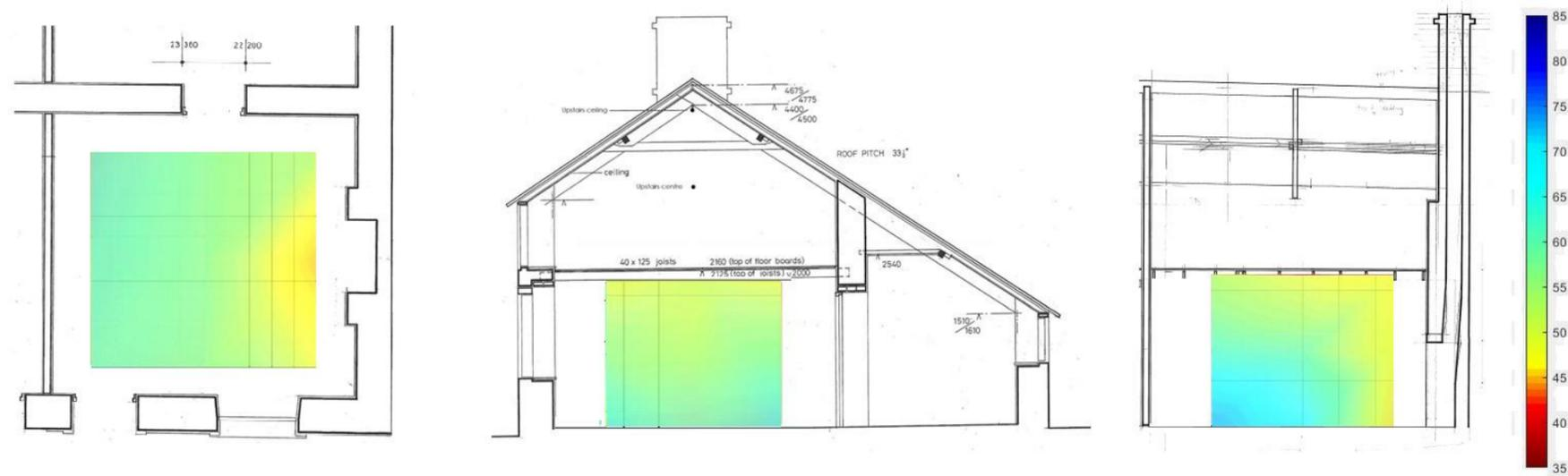
Figure 97: Cross-sectional image of RH distribution at 02:00 21/11/17 Experiment 1 Banked fire.
