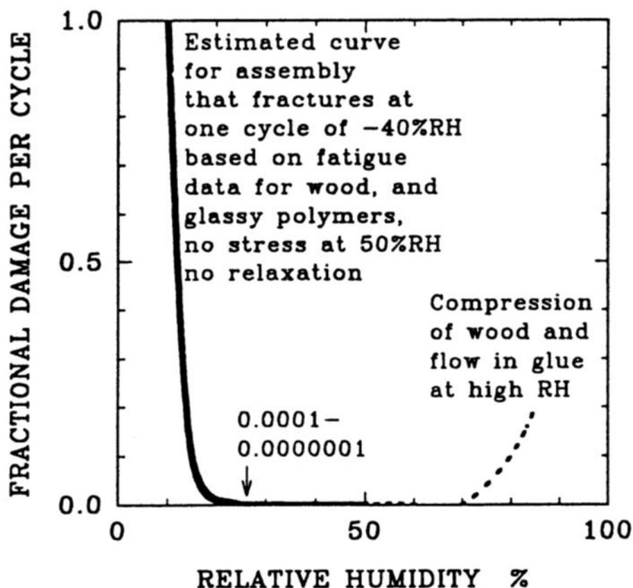
Figure 55: Estimated shape of a curve for mechanical damage function of RH fluctuation from some middle value. The solid line for shrinkage fracture assumes a linear rise in tension from 50% RH to some critical value at 10% RH. (Michalski 1993a, 626).
