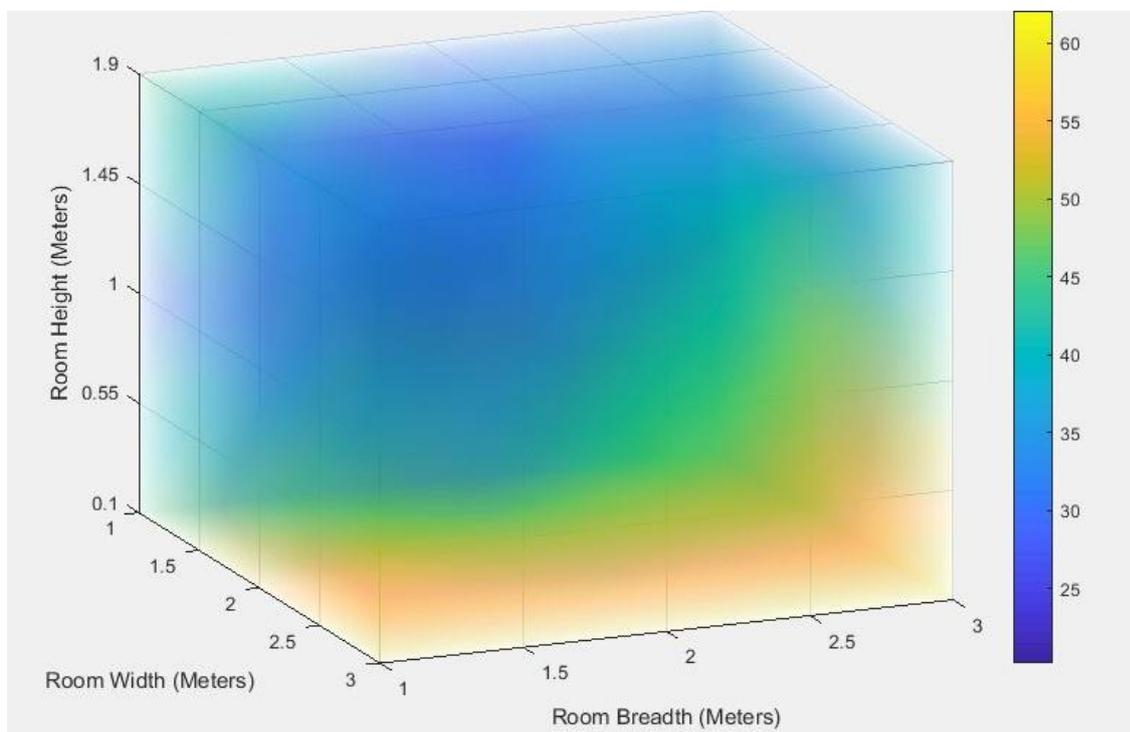
**Figure 87: 3D interpretation of RH in Rhyd-y-Car No.6 at 22:00 21/11/2017, Experiment 1 (scale is different to later graphs)**
