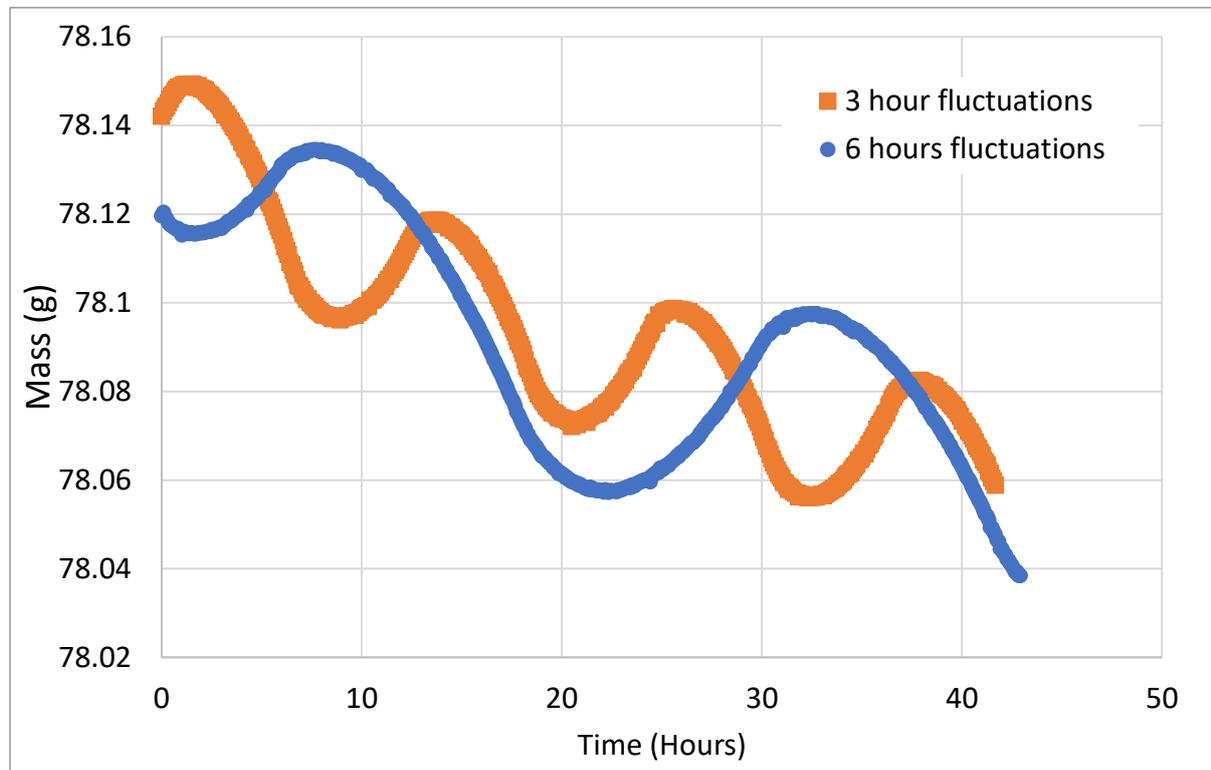
**Figure 170: Response of timber sample to RH fluctuations for sample 2D.**
