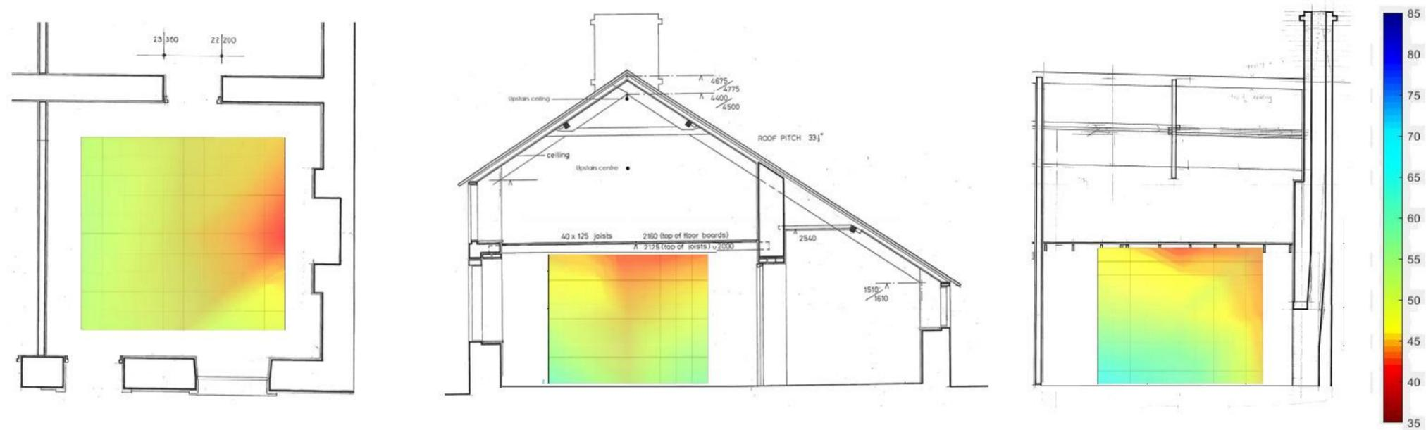
Figure 95: Cross-sectional image of RH distribution at 22:00 20/11/17 Experiment 1 Banked fire.
