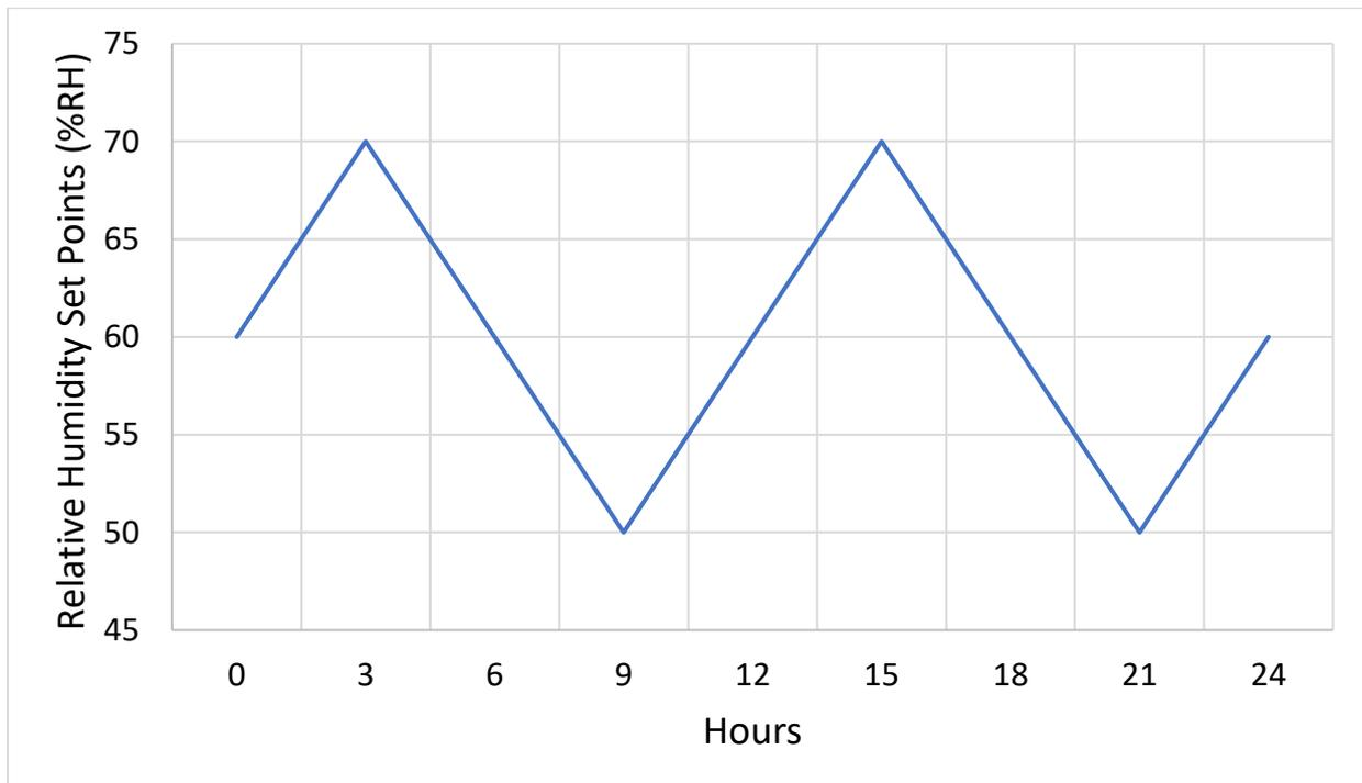
**Figure 165: Climatic chamber set points for three house tests.**
