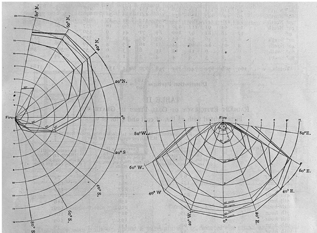
**Figure 135: Intensity of radiation from open fire recorded by thermopile (Fishenden 1920, 7).**
