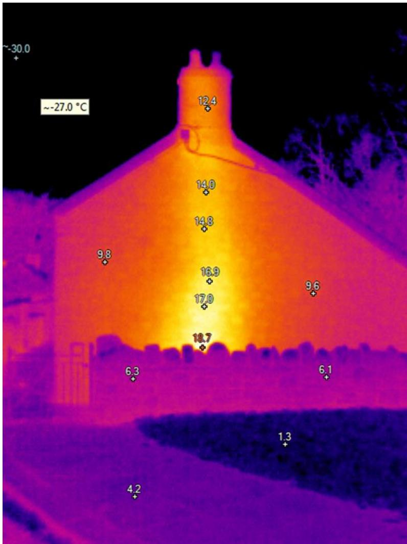
**Figure 143: Infrared image of the pine end of Rhyd-Y-Car No.6, showing the heat from chimney.**
