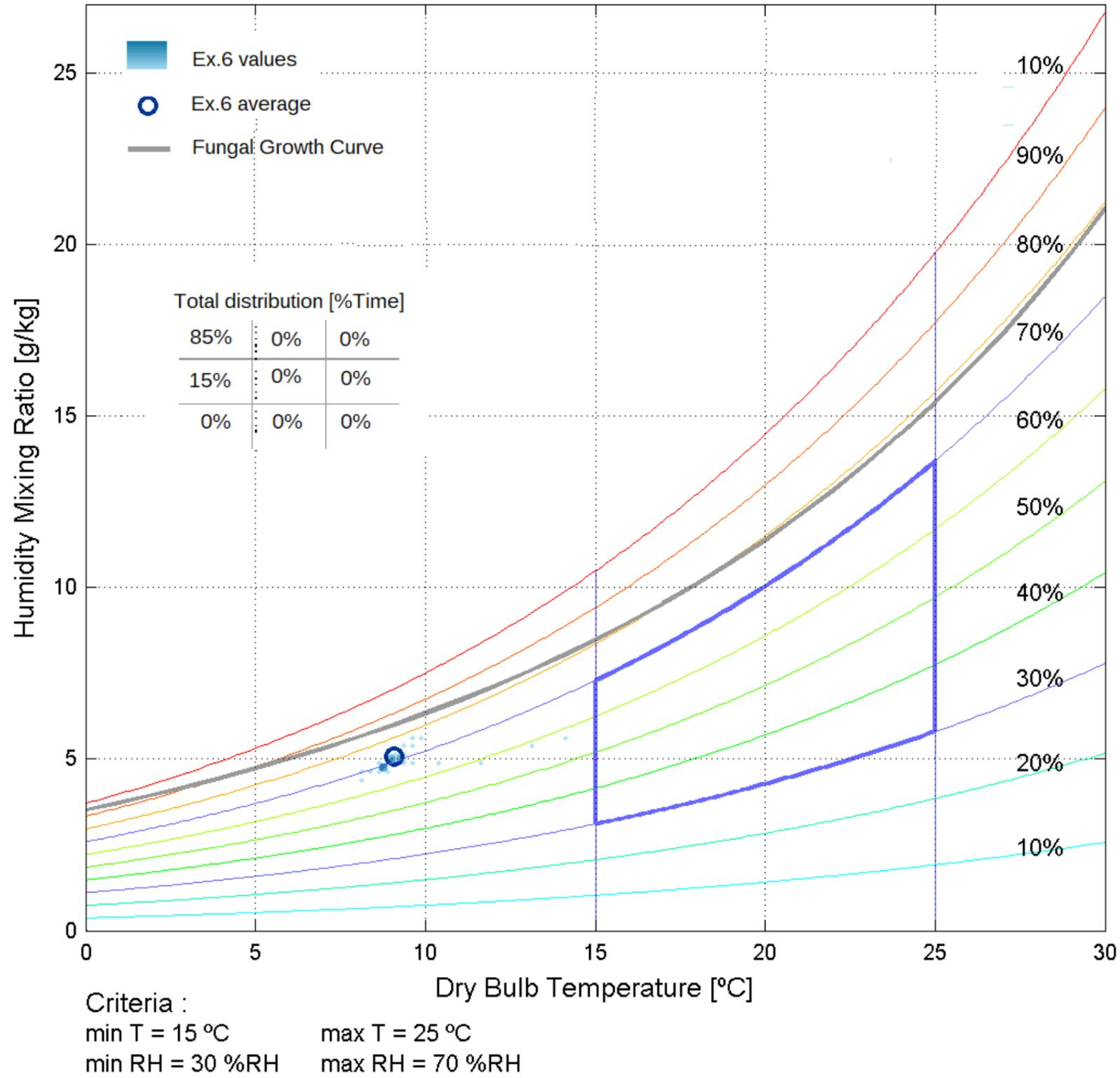
Figure 83: Climate Evaluation Chart showing that RH and temperature measured during Week 6 (circled in pale blue) fall outside the defined RH and temperature goal values (darker blue outlined region).
