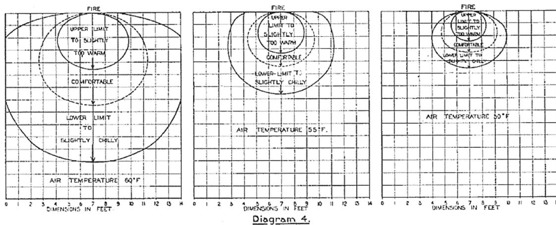
ZONES OF COMFORT WHICH WOULD BE PRODUCED BY THE RADIATION FROM A FIRE BURNING 2 LBS. OF COAL PER HOUR WHEN THE AIR TEMPERATURES HAD REACHED 60°F, 55°F, 50°F.
