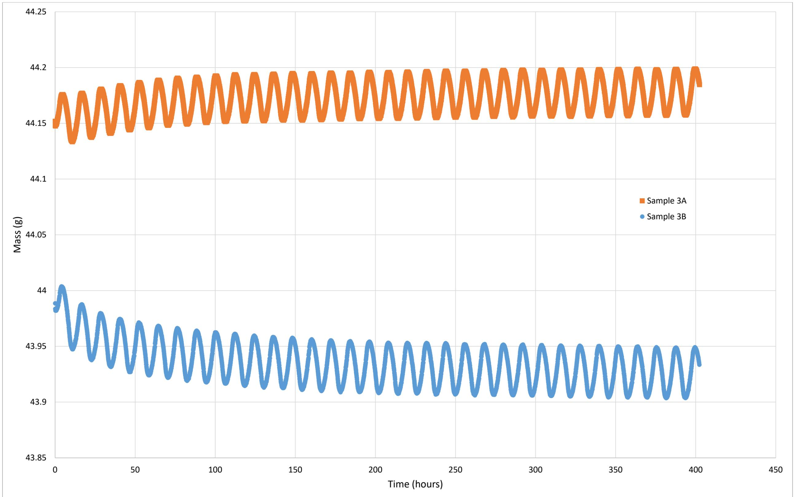
Figure 168: Timber sample RH% fluctuation response showing mass for samples 3A and 3B.
