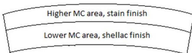
**Figure 176:** End grain view of timber board with shellac and stain finish exposed to high RH levels for 30 days.
