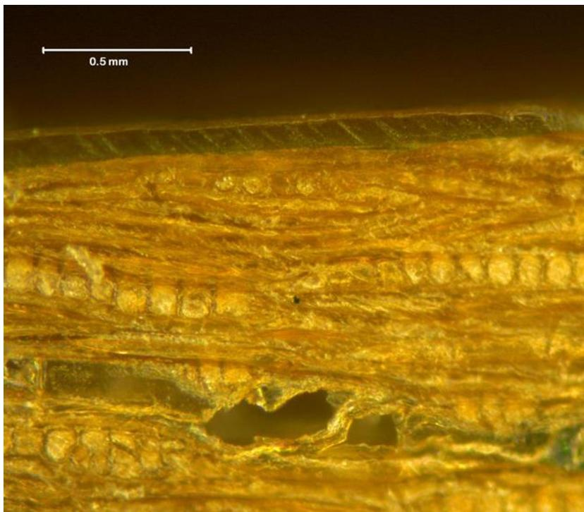
**Figure 153: Microscope image of sample cross section from sample 2, showing the shellac layer**
