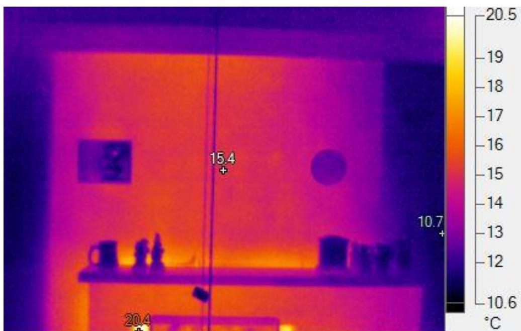
**Figure 149: Experiment 4 day 4, 20 hours after the fire is out. Room centre temperature 9.6°C**
