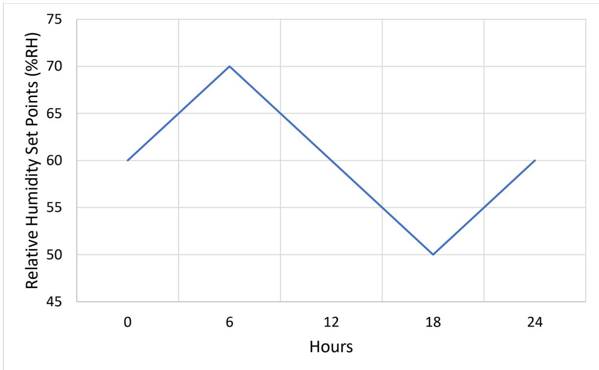
**Figure 166: Climatic chamber set points for six hour fluctuation tests.**
