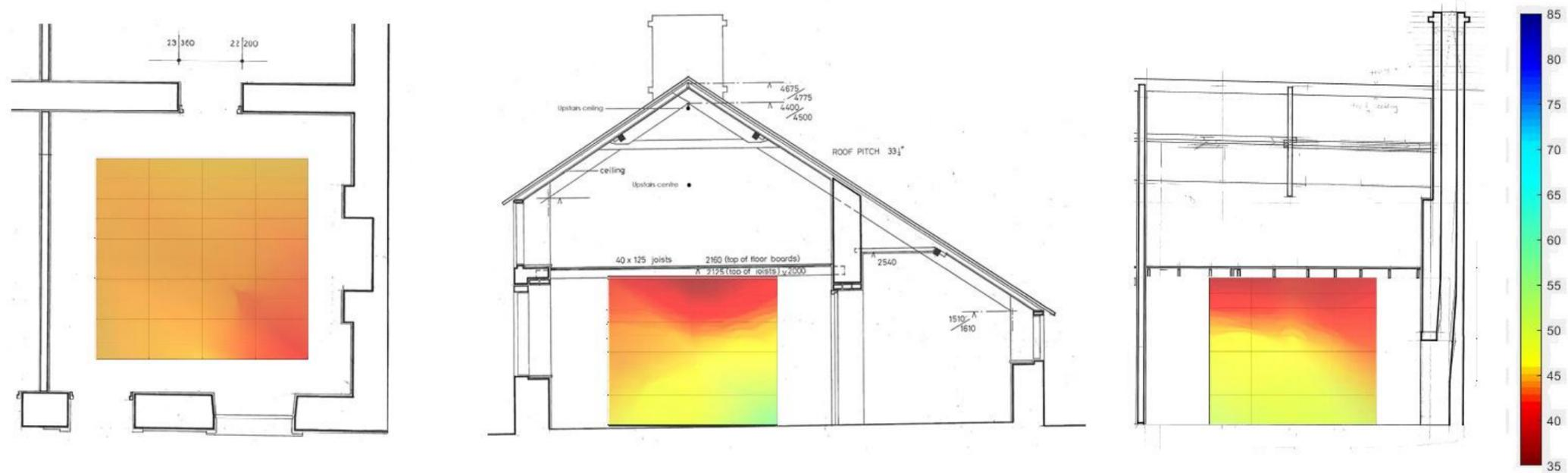
Figure 107: Cross-sectional image of RH distribution at 22:00 15/1/18 Experiment 5 Daily fire.
