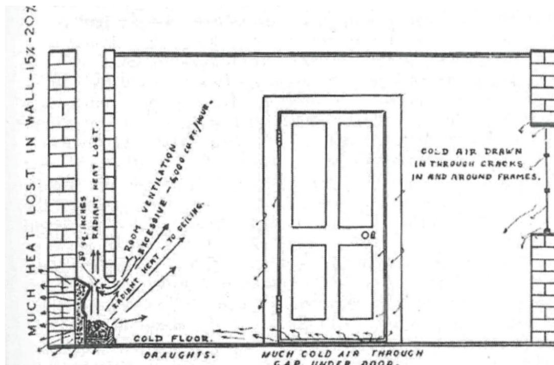
Figure 136: Warming and ventilation from open fire (Angus 1956, 135).
