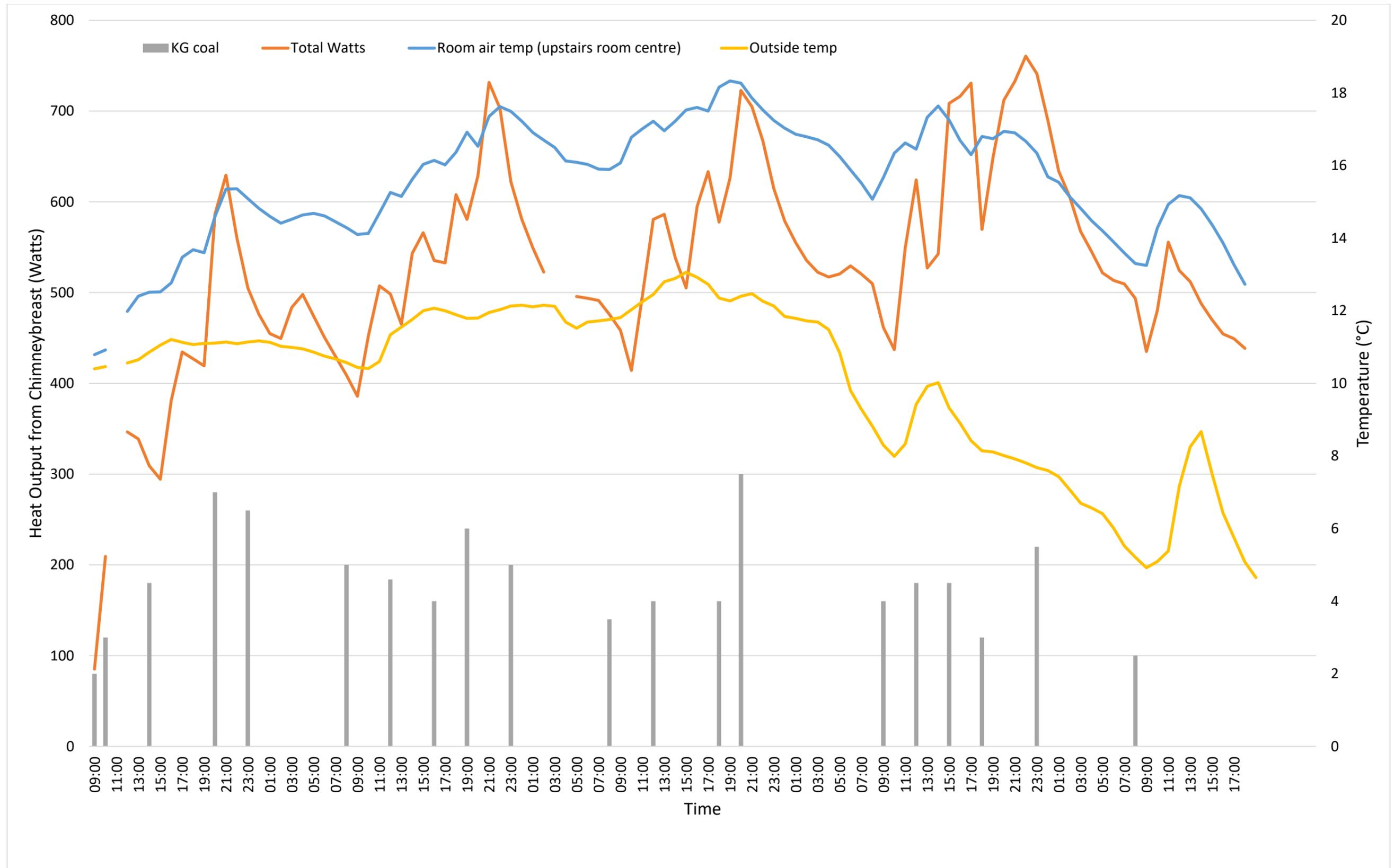
Figure 126: Watts output from chimney breast against room air temperature, outside temperature and coal consumption for Experiment 1, banked in fire.
