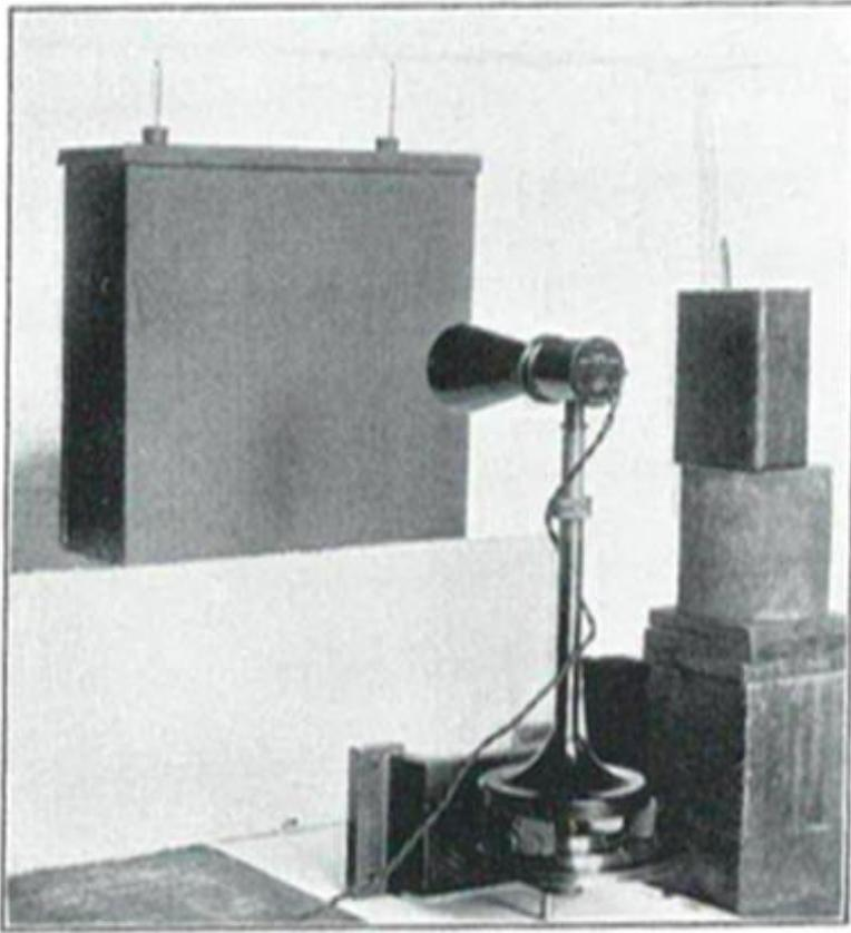
**Figure 28: A thermopile being calibrated against a known emitter (copper box coated in lampblack, filled with water of known temperature).**
