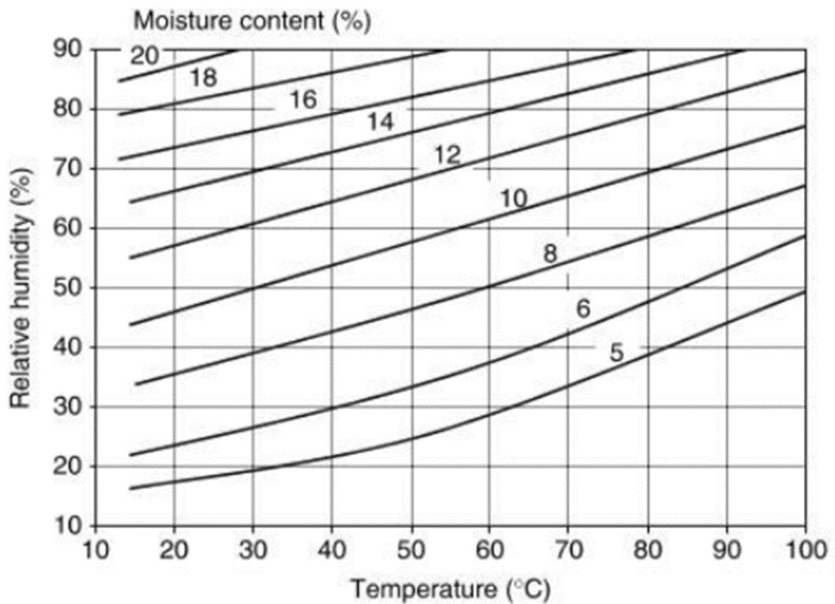
Figure 49: Relationship between moisture content and temperature and humidity in timber (Domone et al. 2010, 423).
