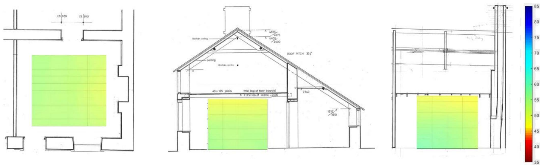
Figure 111: Cross-sectional image of RH distribution at 06:00 16/1/18 Experiment 5 Daily fire.
