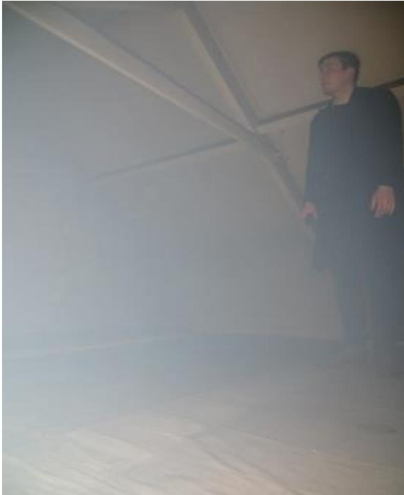
**Figure 64: Upstairs in Rhyd-Y-Car No.4 Following insertion of the fire hood downstairs, it was discovered smoke was syphoning down the bedroom fireplace chimney.**
