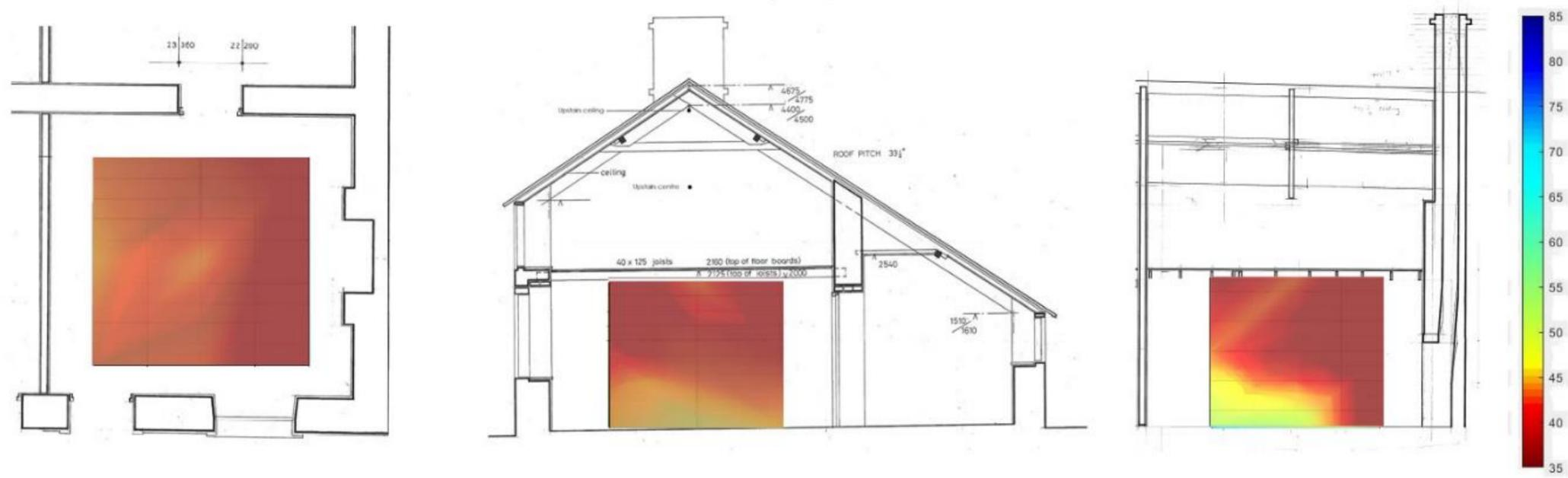
Figure 103: Cross-sectional image of RH distribution at 14:00 15/1/18 Experiment 5 Daily fire.
