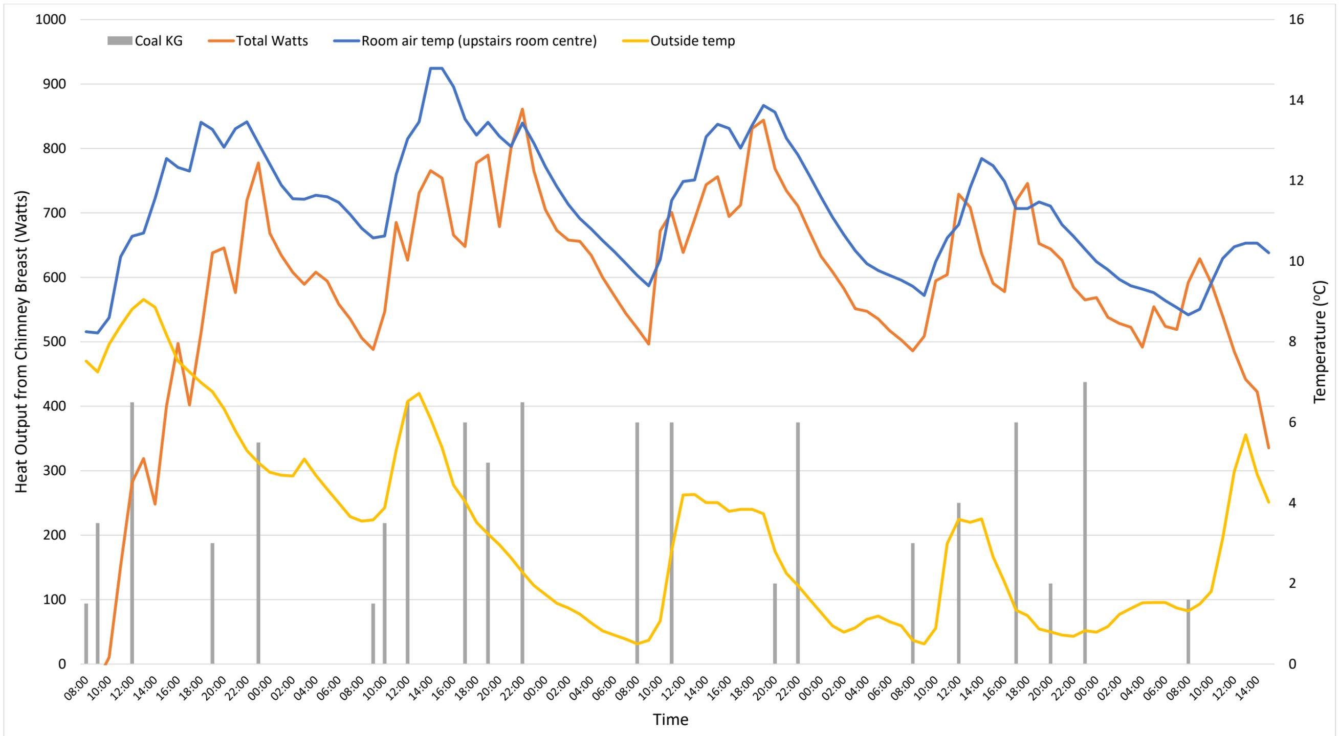
Figure 127: Watts output from chimney breast against room air temperature, outside temperature and coal consumption. Experiment 2, banked in fire.
