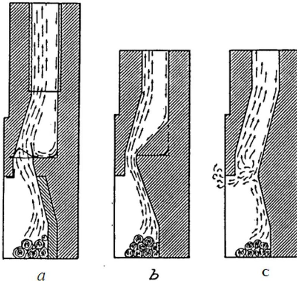
Figure 31: Cross section of fireplaces and different throat openings (Rosin 1939, 16).
