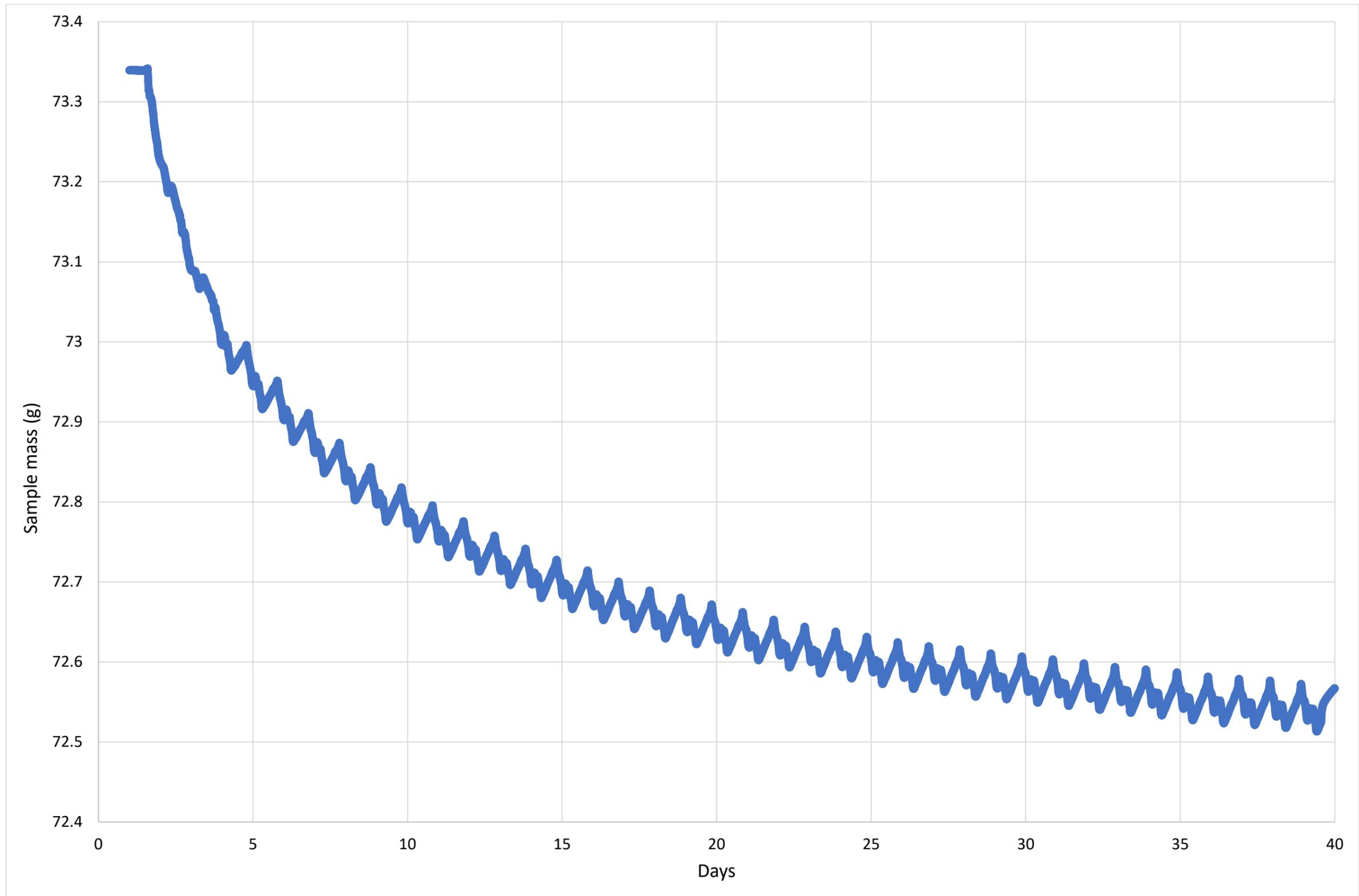
Figure 164: Sample 2A, mass of sample responding to daily RH fluctuations.
