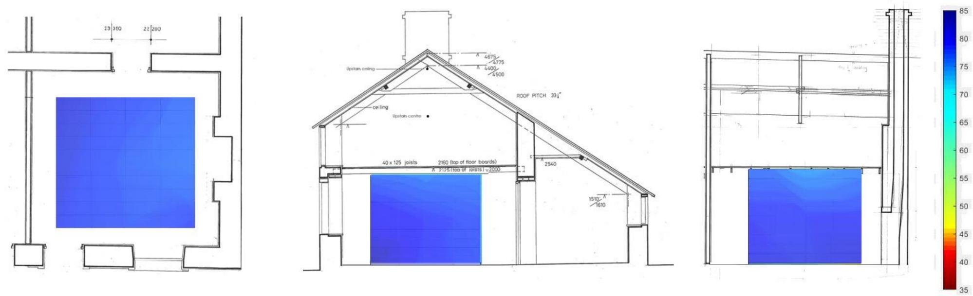
Figure 88: Cross-sectional image of RH distribution at 8AM 20/11/17 Experiment 1 Banked fire.
