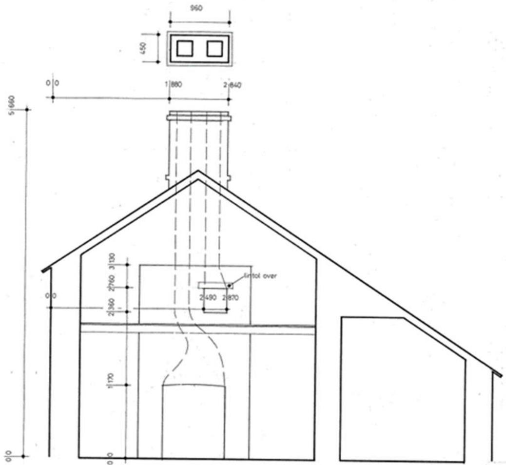
**Figure 72: Cross section of fireplaces and chimneys, Rhyd-y-Car Cottages**
