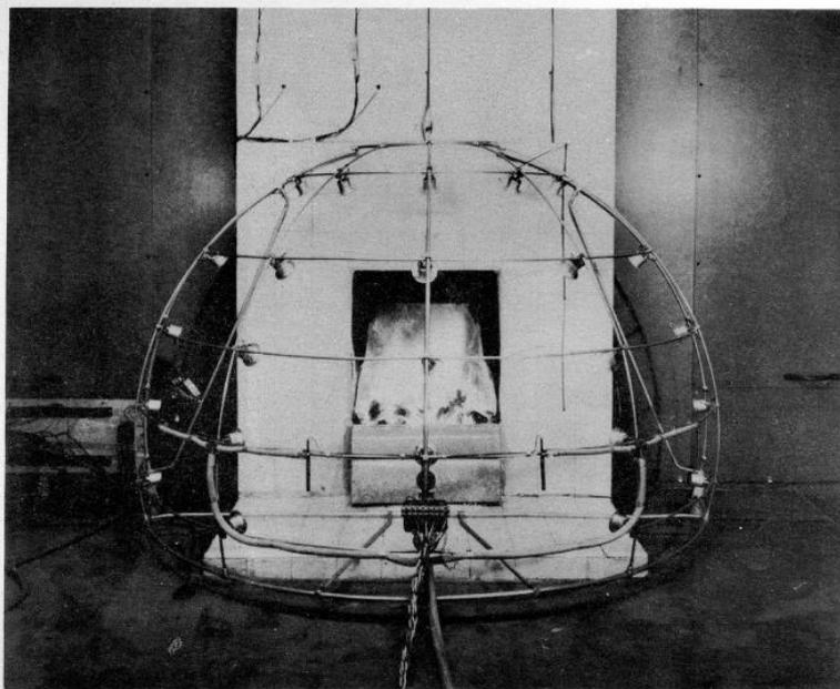
**Figure 36: A BCURA cage radiometer in use (Venables 1957a, 8).**
