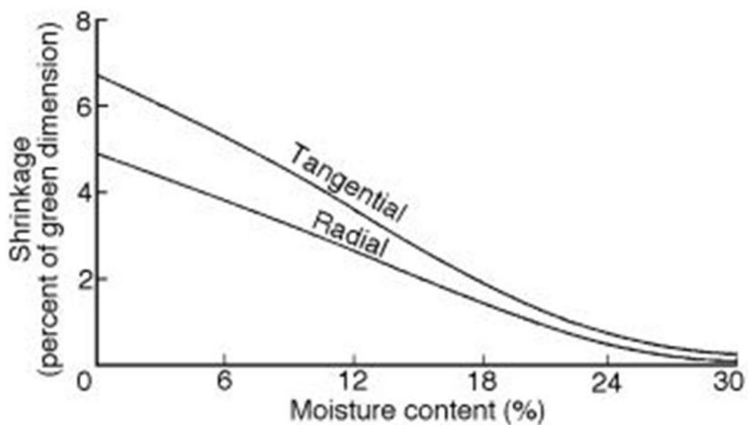
Figure 50: Typical moisture content shrinkage curves (Simpson 2001, 13).
