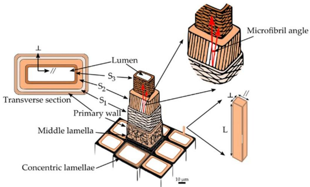
**Figure 47: Diagram showing makeup of cell walls and patterns of primary, S1, S2 and S3 show microfibril orientation. Directions in cell wall are shown in the parallel ( $\parallel$ ) and perpendicular ( $\perp$ ) and defined in the transverse plane in relation to the lumen surface (Arzola-Villegas et al. 2019, 4).**
