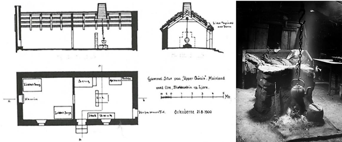
Figure 13: Orkney house with central fireplace 1906, showing clearly the roof vent (louvre) for the removal of smoke (Fenton 1978, 198; <https://photos.orkneycommunities.co.uk/picture/number28451.asp>).
