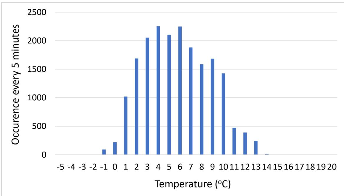
Figure 78: External temperature frequency calculated as whole numbers for Experiments 1-6.
