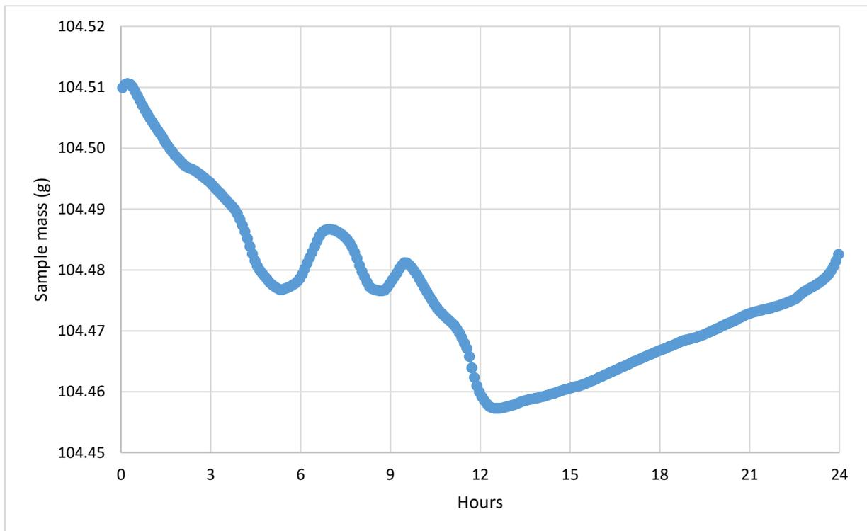
**Figure 162:** A close up of a section from Figure 163, sample 1A weight during one of the 24 hour fluctuation RH cycles, showing how closely it follows the RH pattern in Figure 161.
