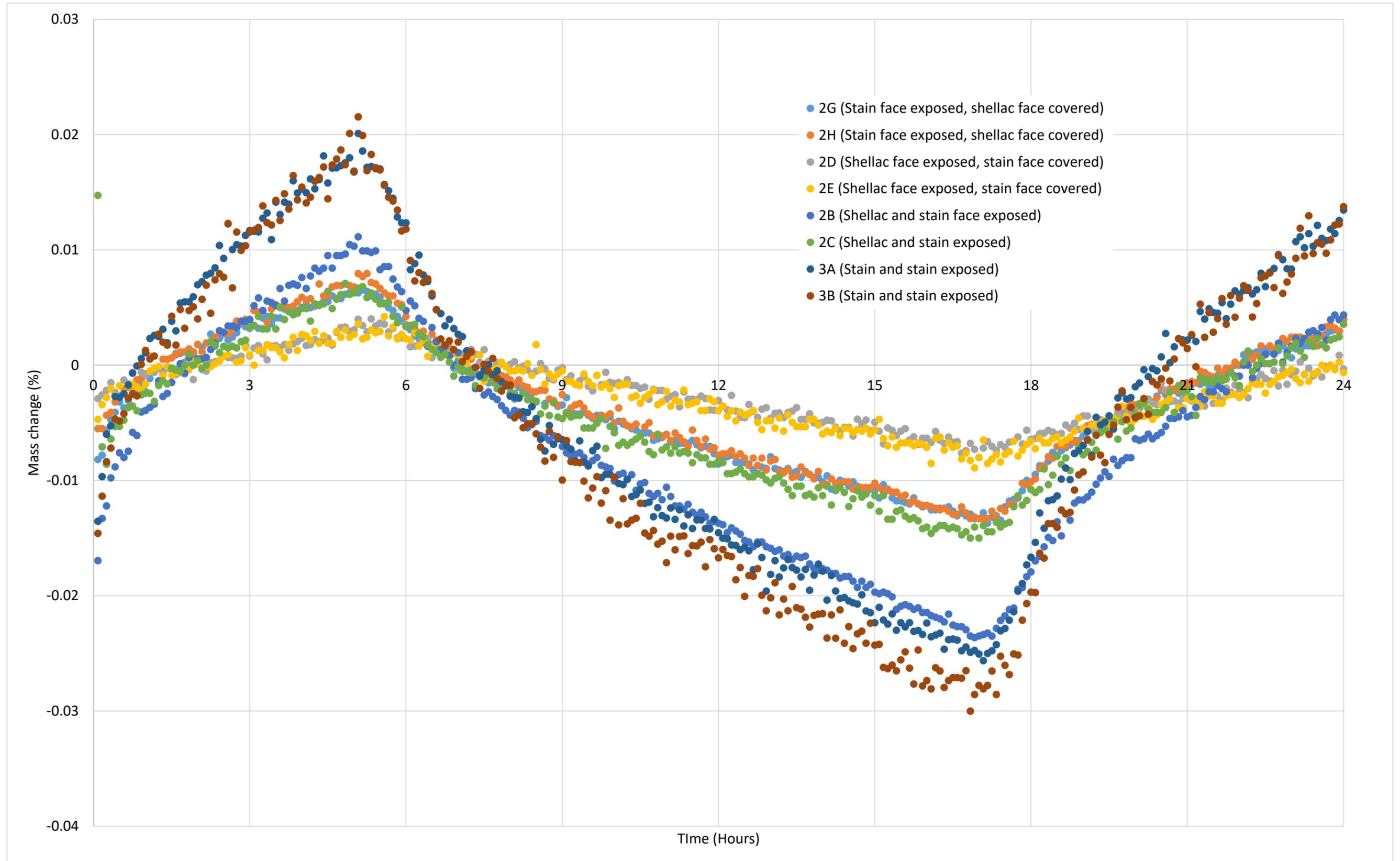
Figure 172: Hourly percentage mass gain/loss of sample over 6 hour fluctuations over 24 hours.
