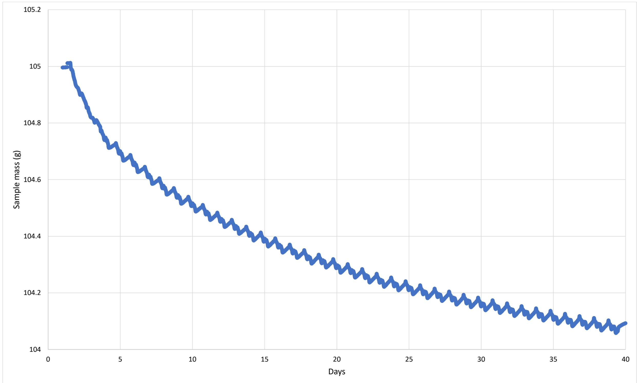
Figure 163: Sample 1A, mass of sample responding to daily RH fluctuations.
