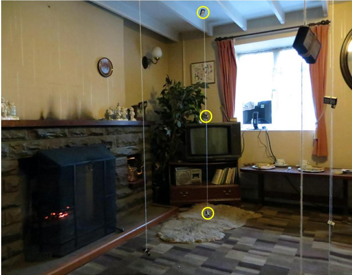
**Figure 70: Loggers on string, fireplace and chimney breast. Yellow circles indicate the locations of three loggers on one string from ceiling to floor.**
