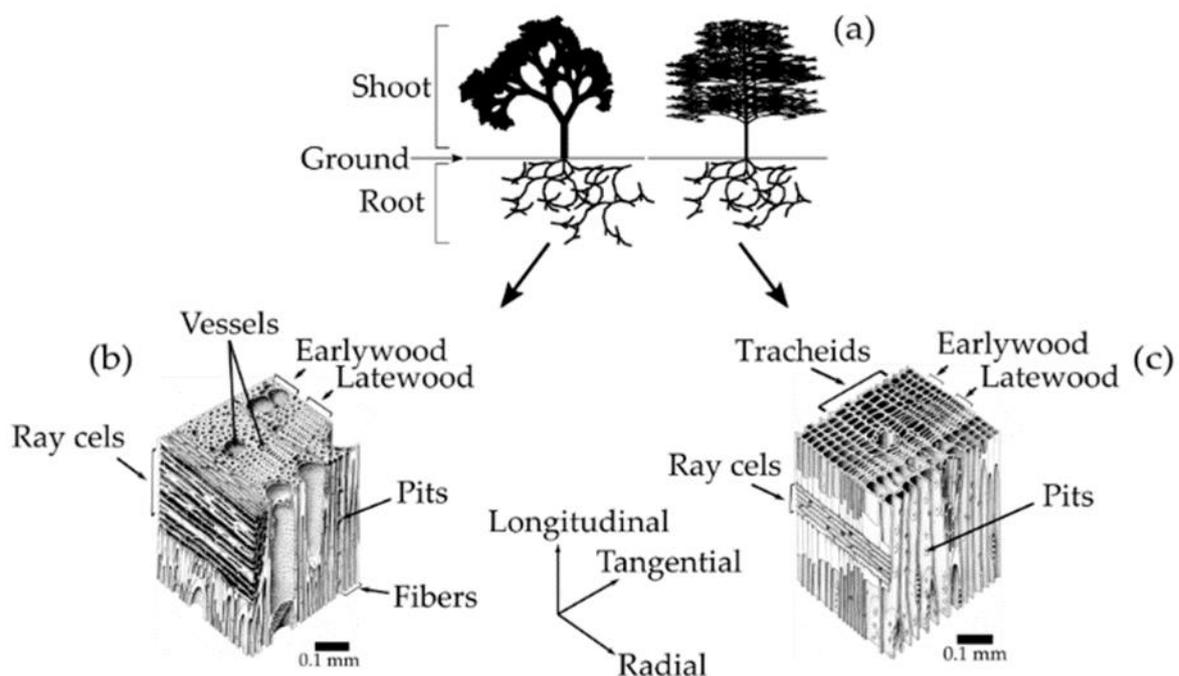
**Figure 40: Representation of structure of hardwood (b) and softwood (c), giving an overview of cellular structure in all three directions with various elements, such as the earlywood and latewood forming rings, the pits between vessels, vessels, and ray cells (Arzola-Villegas et al. 2019, 3).**
