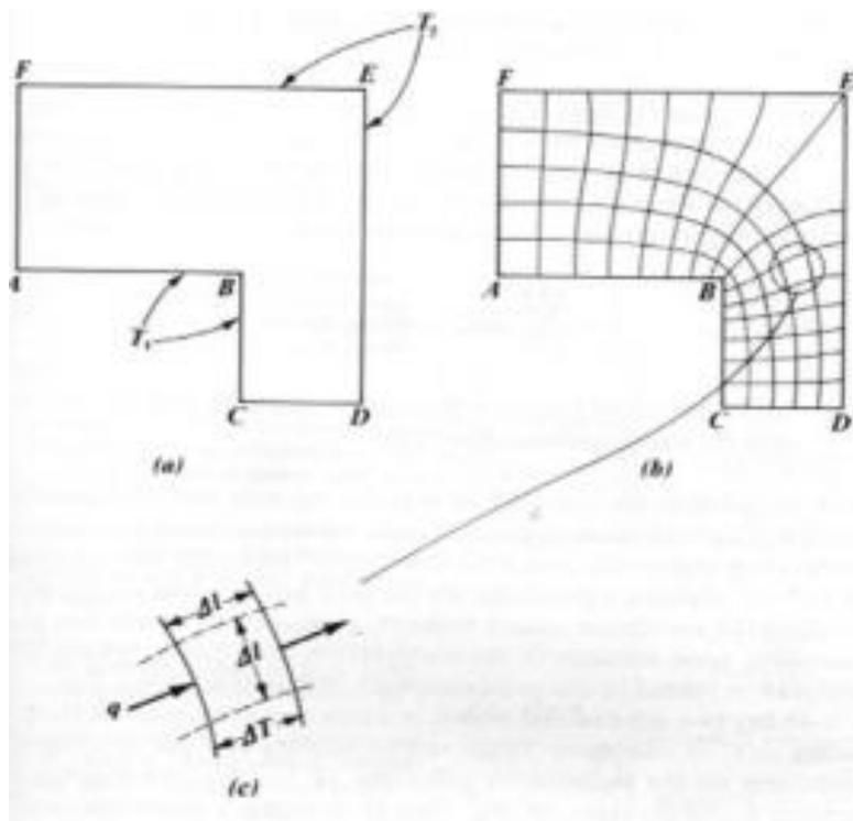
**Figure 147: Diagram showing heat transfer of a corner, how the external surface area is larger than the internal surface area (Kreith 1973).**
