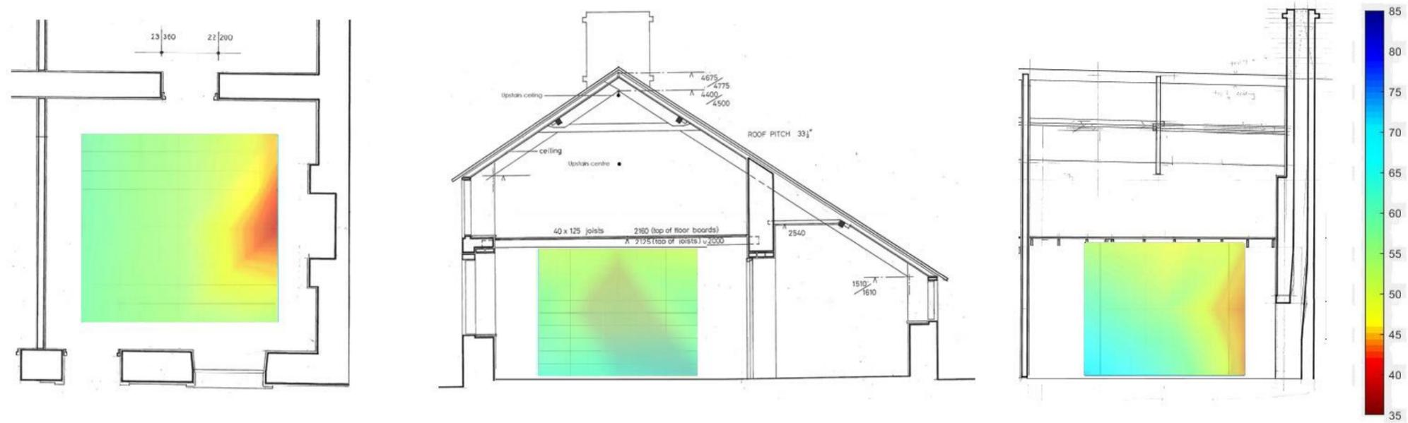
Figure 92: Cross-sectional image of RH distribution at 16:00 20/11/17 Experiment 1 Banked fire.
