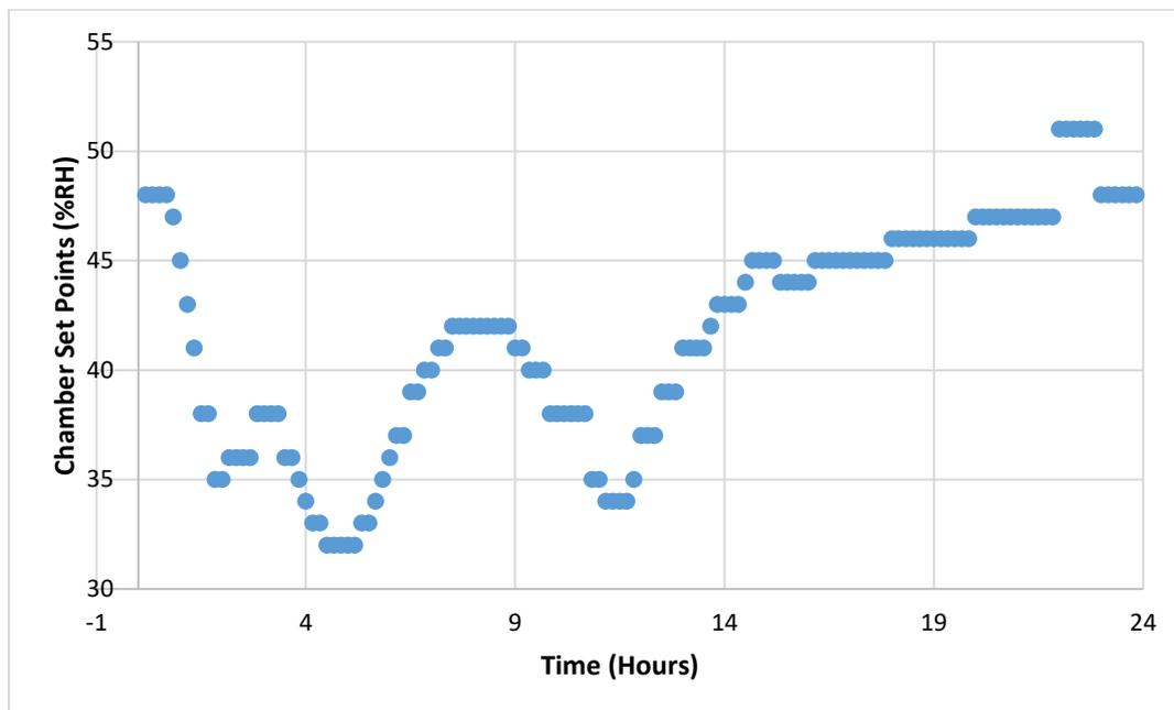
**Figure 161: Climatic chamber set points for banked in fires model run over 24 hours and repeated thereafter.**
