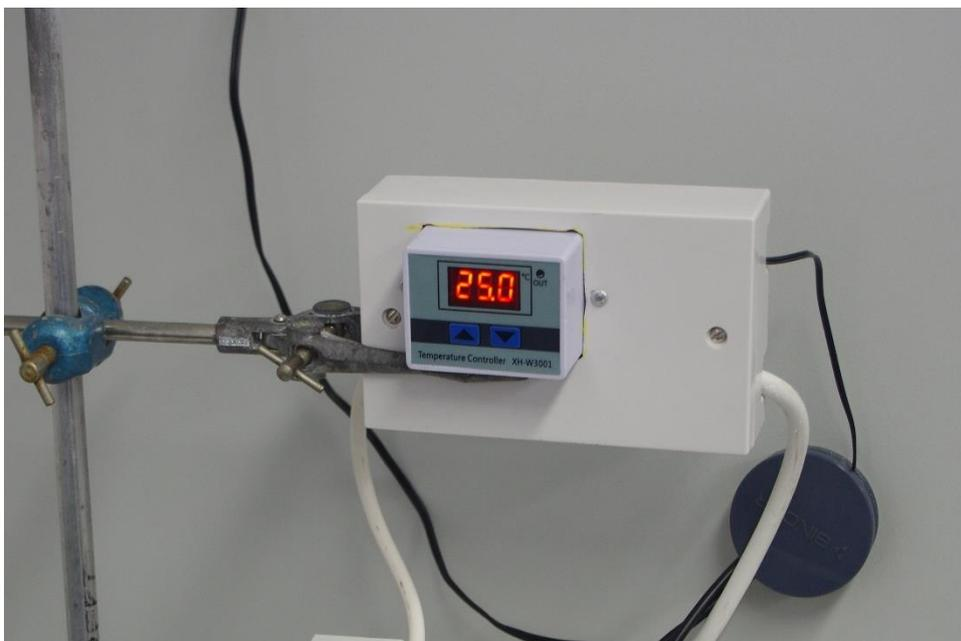
**Figure 178: Thermostat microcontroller for switching the element on and off.**
