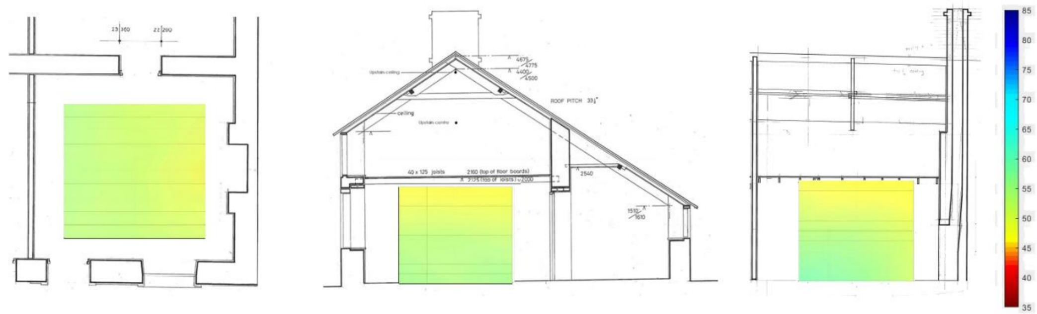
Figure 109: Cross-sectional image of RH distribution at 02:00 16/1/18 Experiment 5 Daily fire .
