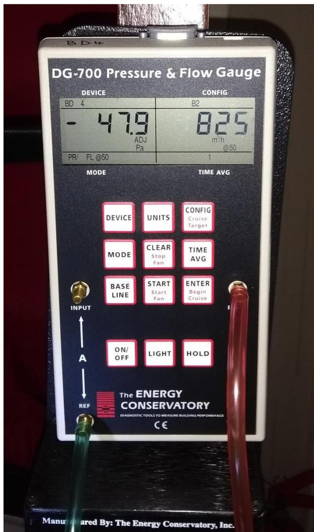
Figure 75: Pressure flow gauge from air exchange test.
