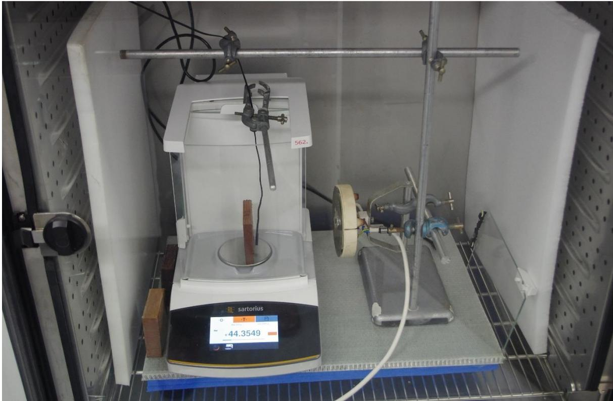
**Figure 177: Radiant heat experimental setup. Showing sample on balance in climatic chamber, with heating element and thermostat sensor in front of sample.**
