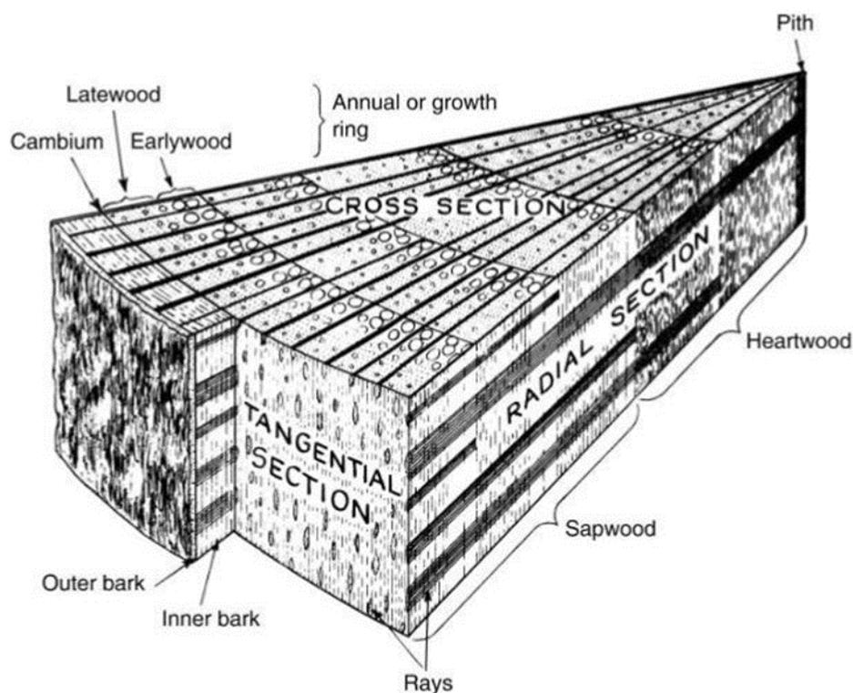
**Figure 42: Five year old wedge of timber showing makeup of the wood (Desch et al. 1996, 11).**
