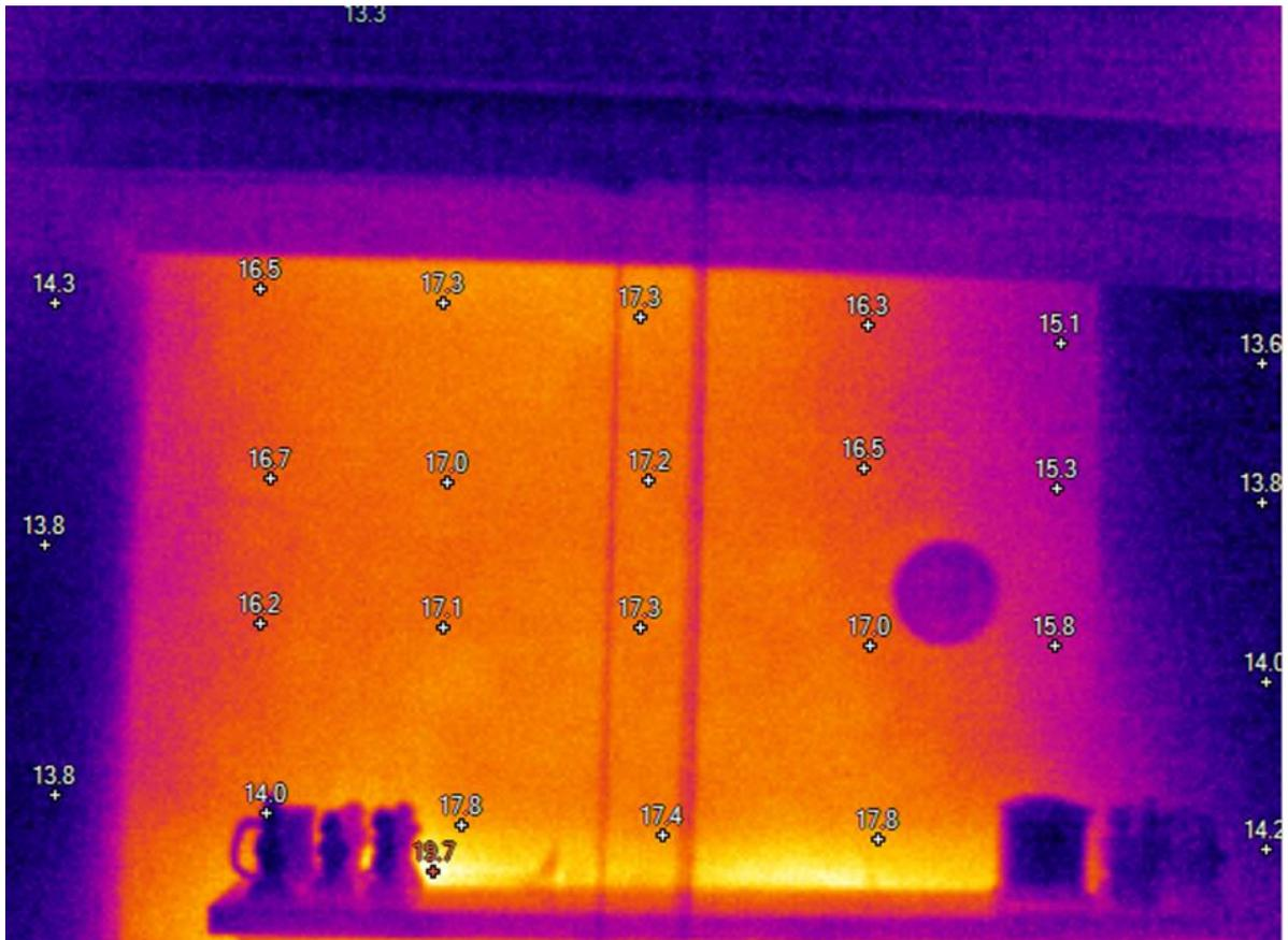
**Figure 145: Chimney breast temperature 20 hours after the fire has gone out.**
