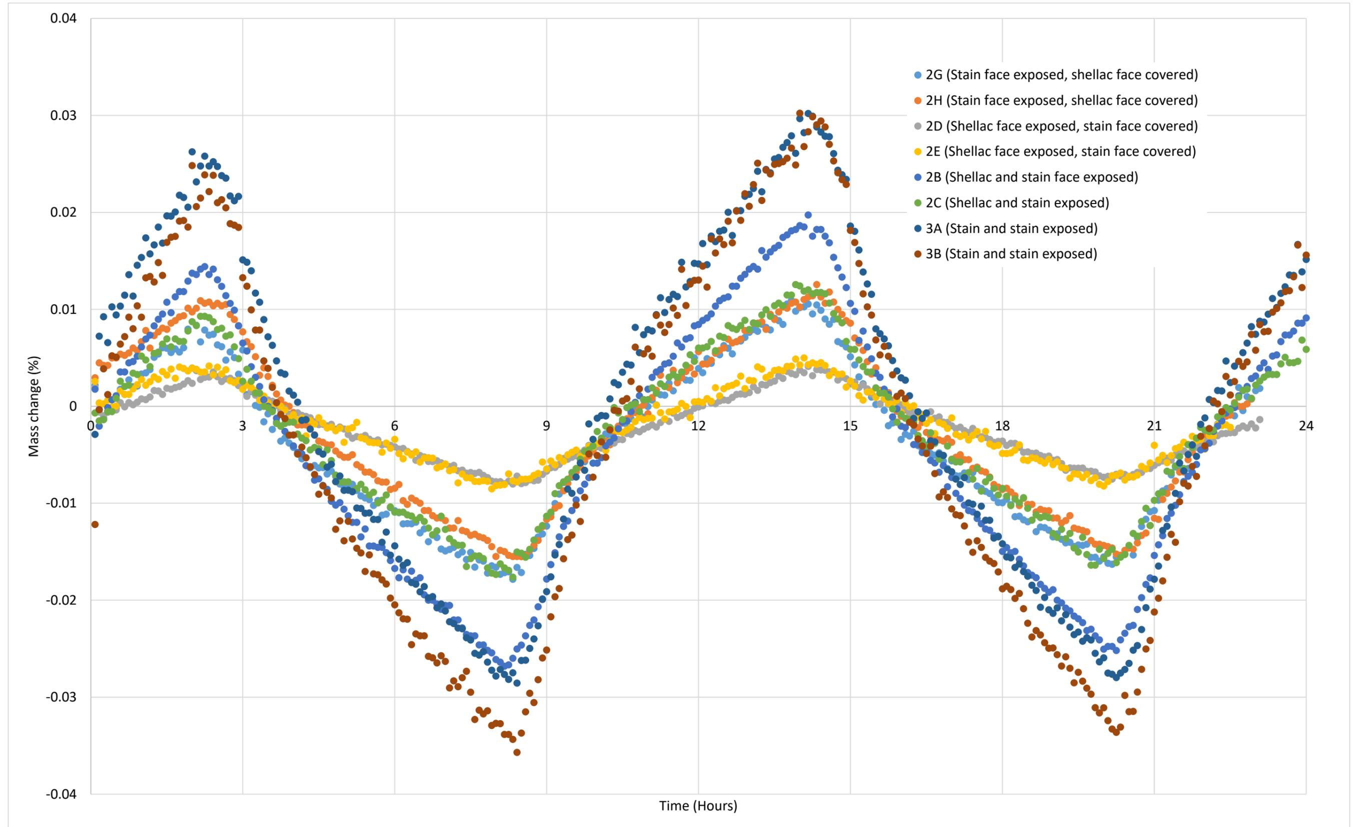
Figure 171: Hourly percentage mass gain/loss of samples over three hour fluctuations over 24 hours.
