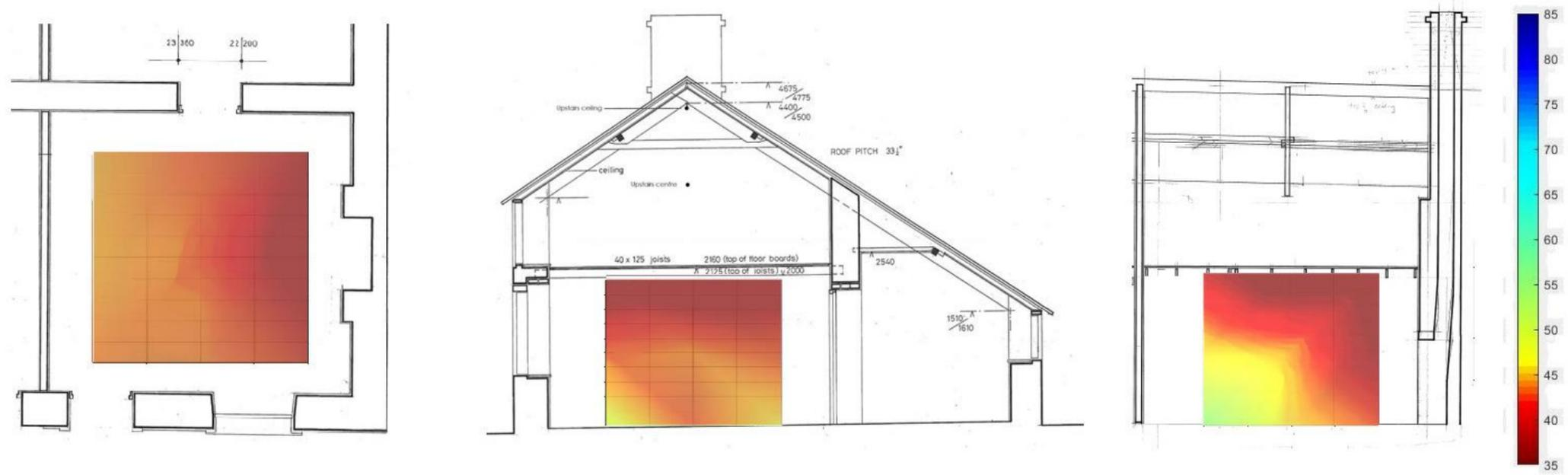
Figure 104: Cross-sectional image of RH distribution at 16:00 15/1/18 Experiment 5 Daily fire.
