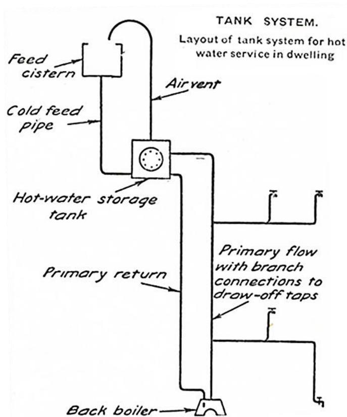
**Figure 38: How a back boiler heats domestic hot water (Stubbs 1949, 1039).**
