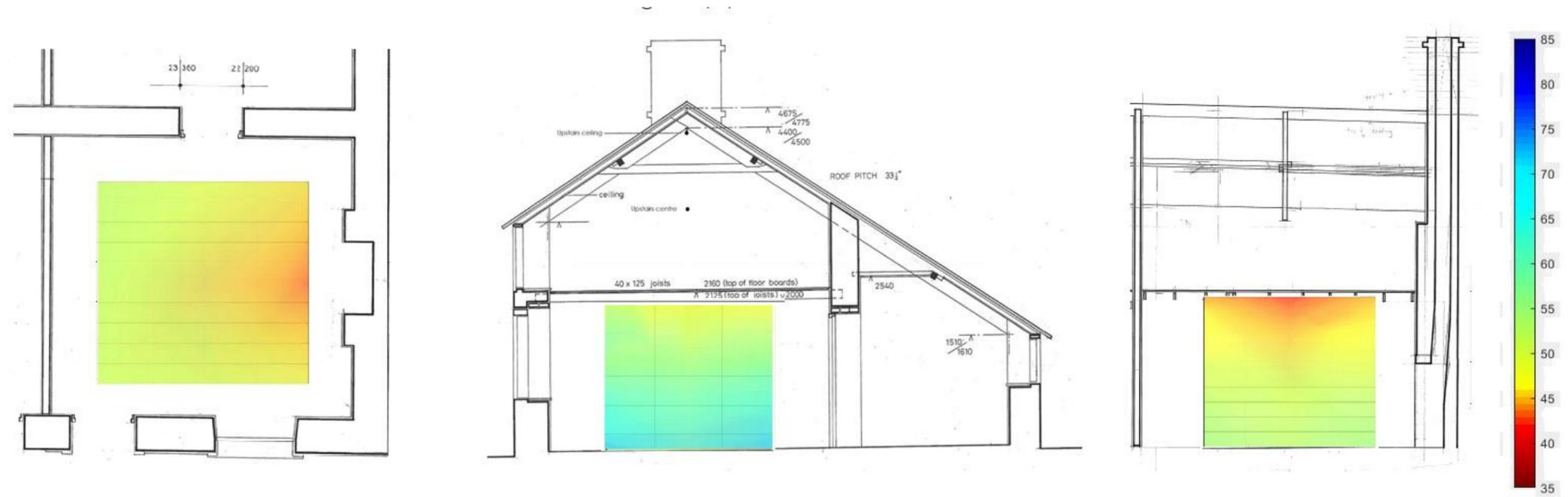
Figure 108: Cross-sectional image of RH distribution at 24:00 15/1/18 Experiment 5 Daily fire.
