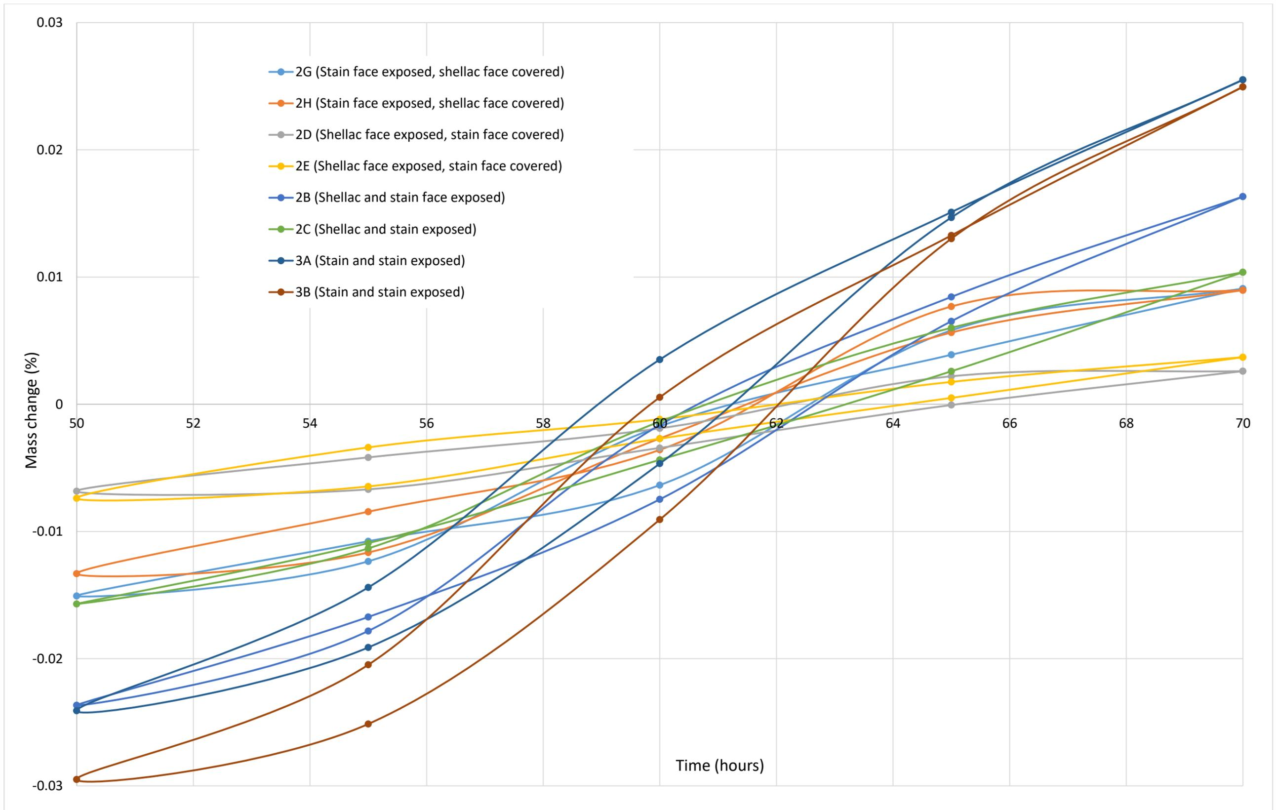
Figure 173: Hysteresis loop for three hour fluctuations, showing hourly percentage mass gain/loss at different RH points for samples..
