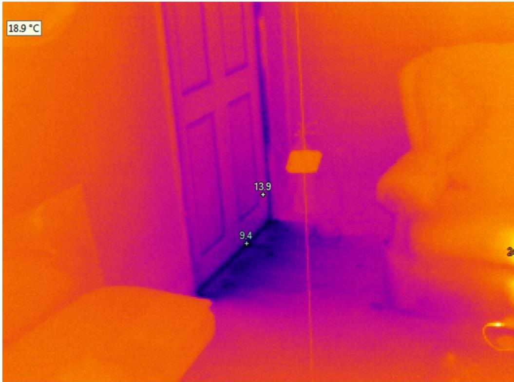
**Figure 137: Infrared image showing low temperature external air ingress into the room.**
