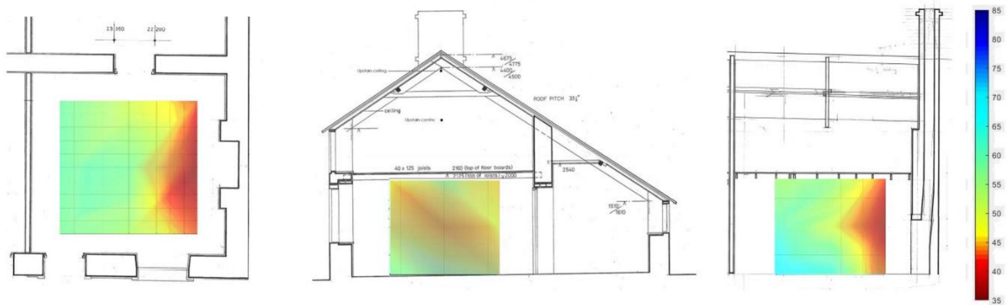
Figure 101: Cross-sectional image of RH distribution at 10:00 15/01/18 Experiment 5 Daily fire.
