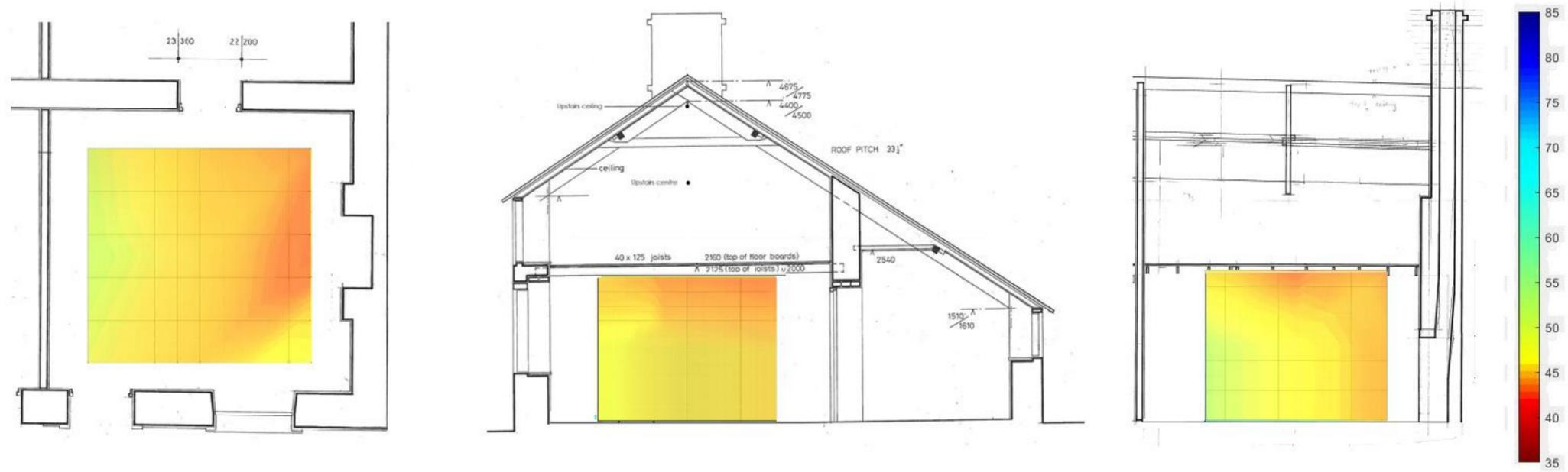
Figure 98: Cross-sectional image of RH distribution at 04:00 21/11/17 Experiment 1 Banked fire.
