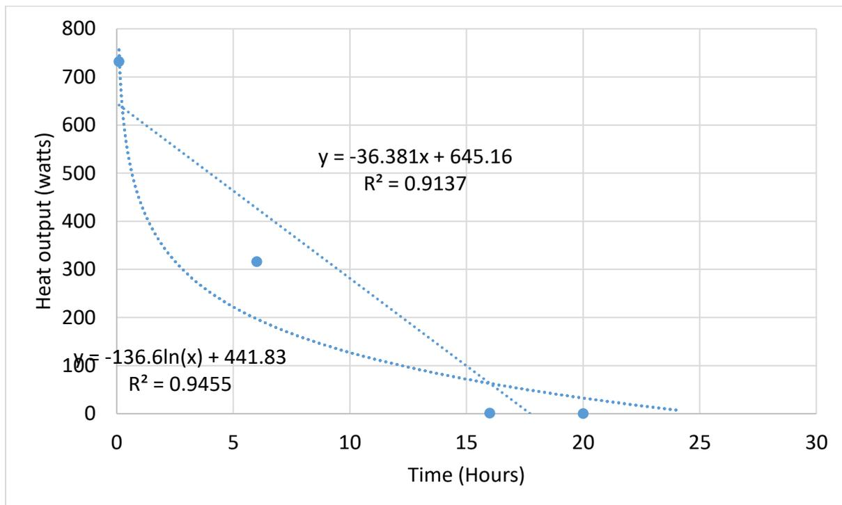
**Figure 146: Heat decay from chimney breast to room. Clear that half-life of first 6 hours is of most benefit. Logarithmic line showing best  $R^2$ . Maximum watts taken from theoretical calculations on heat output later in chapter (which are in line with observed readings for Experiment 1 day 2).**
