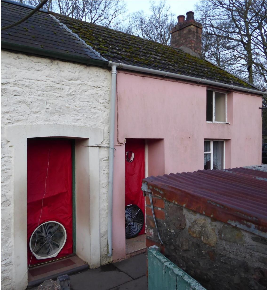
**Figure 74: Blowers inserted into doorways for Rhyd-y-Car No.5 and 6.**
