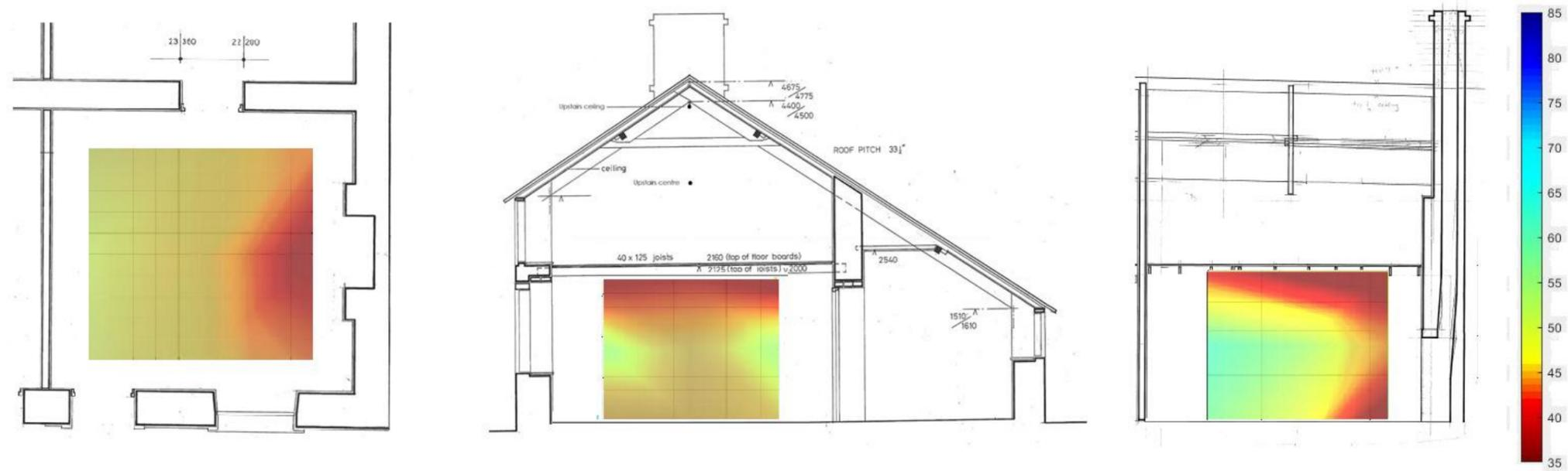
Figure 94: Cross-sectional image of RH distribution at 20:00 20/11/17 Experiment 1 Banked fire.
