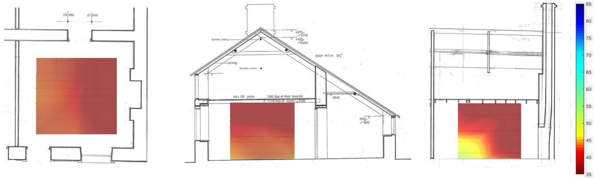
Figure 106: Cross-sectional image of RH distribution at 20:00 15/1/18 Experiment 5 Daily fire.
