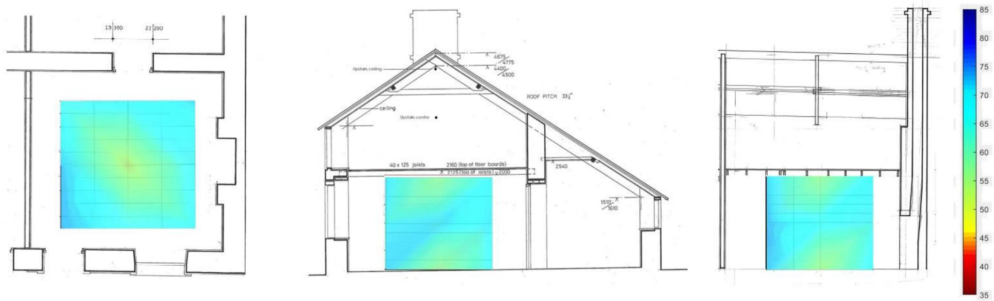
Figure 100: Cross-sectional image of RH distribution at 08:00 15/01/18 Experiment 5 Daily fire.
