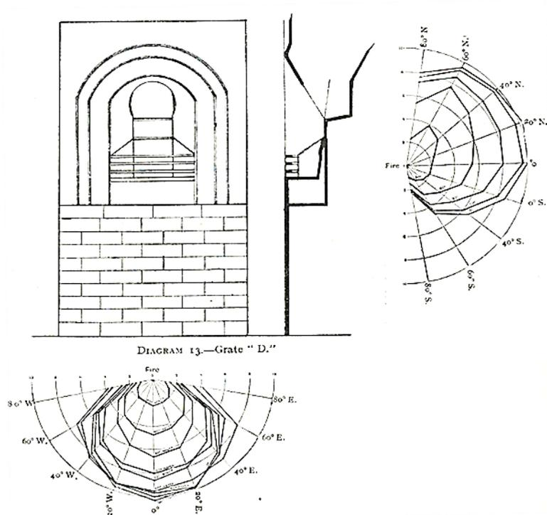
**Figure 29: Results from testing of fireplace showing radiant heat distribution (Fishenden 1920, 18)**
