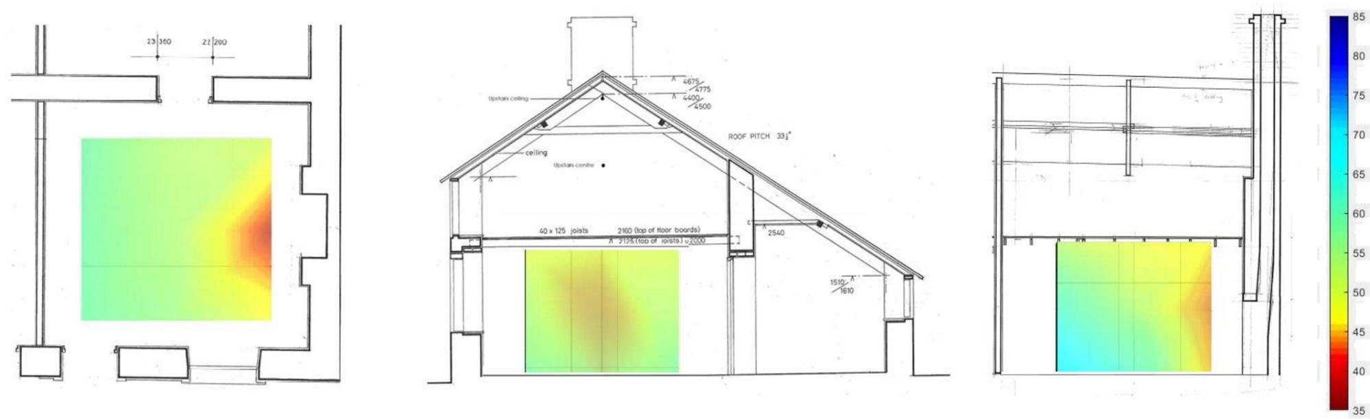
Figure 90: Cross-sectional image of RH distribution at 12:00 20/11/17 Experiment 1 Banked fire.
