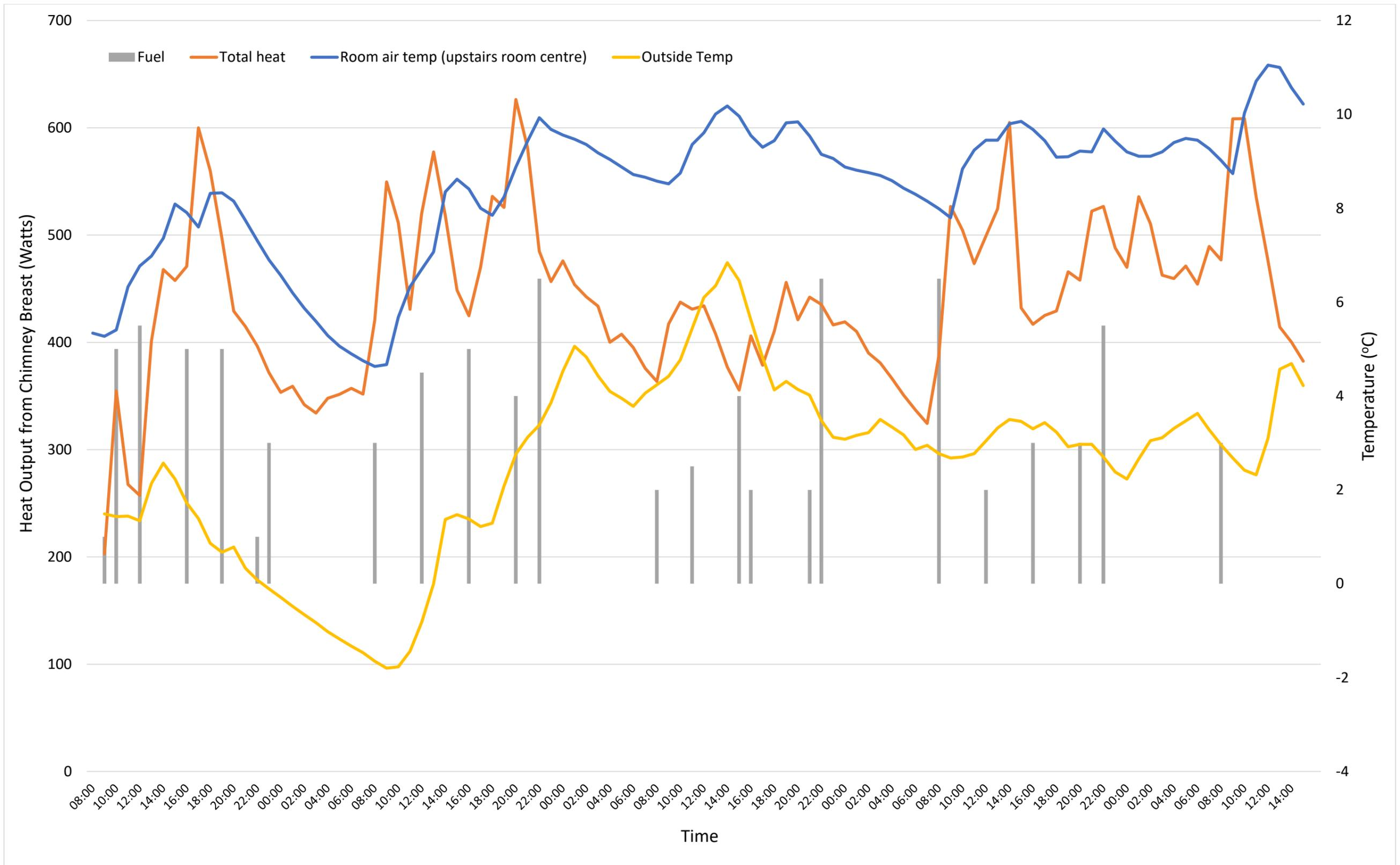
Figure 128: Watts output from chimney breast against room air temperature, outside temperature and coal consumption. Experiment 3, banked in fire.
