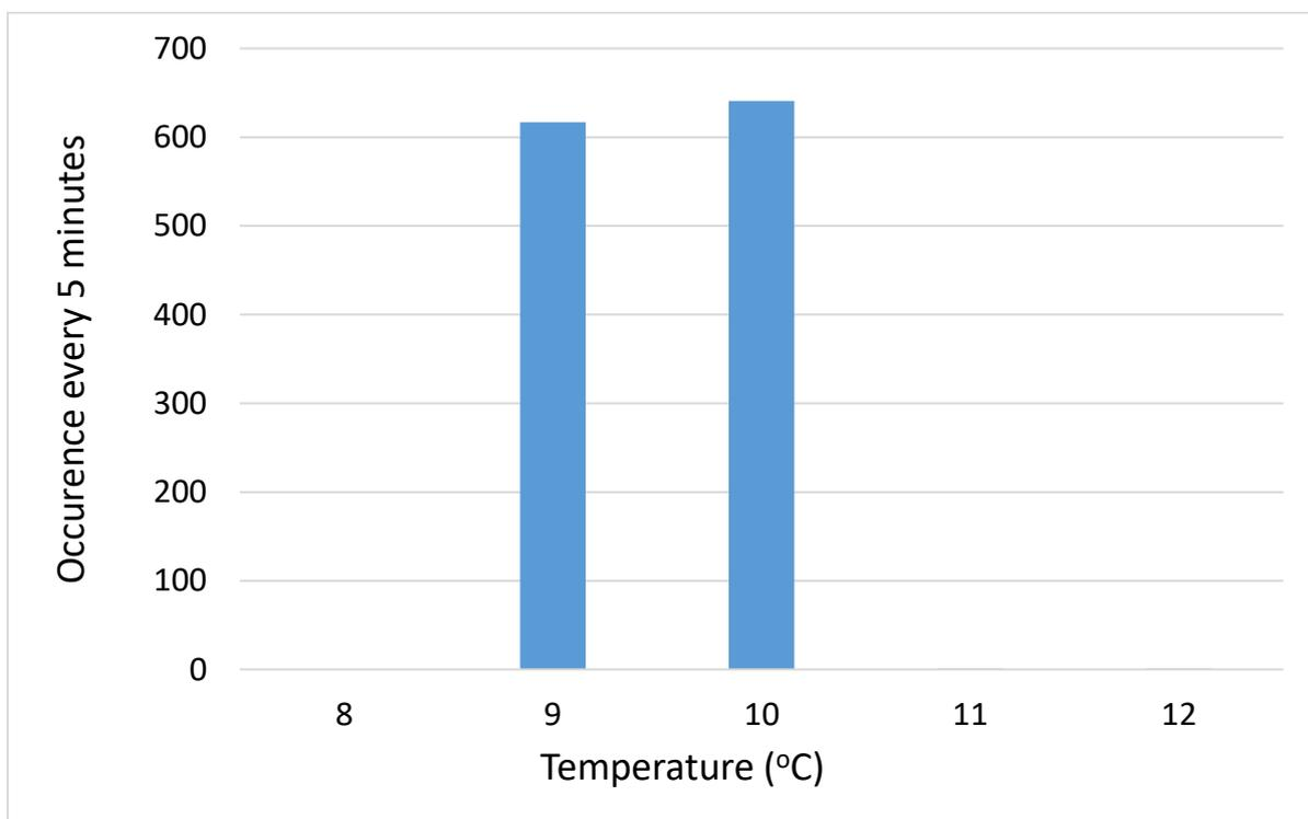
**Figure 81: Temperature frequency for room centre during Experiment 6, 22-26 Jan 2018 unheated room.**
