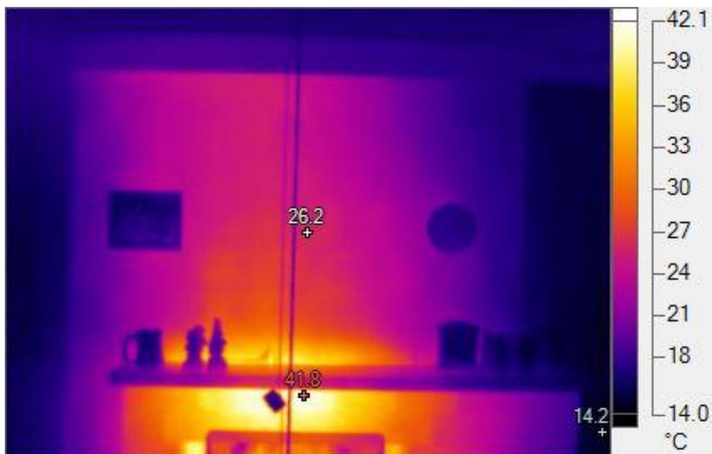
Figure 148: Experiment 4 day 4, 10 hours after the fire is out. Room centre temperature 11°C
