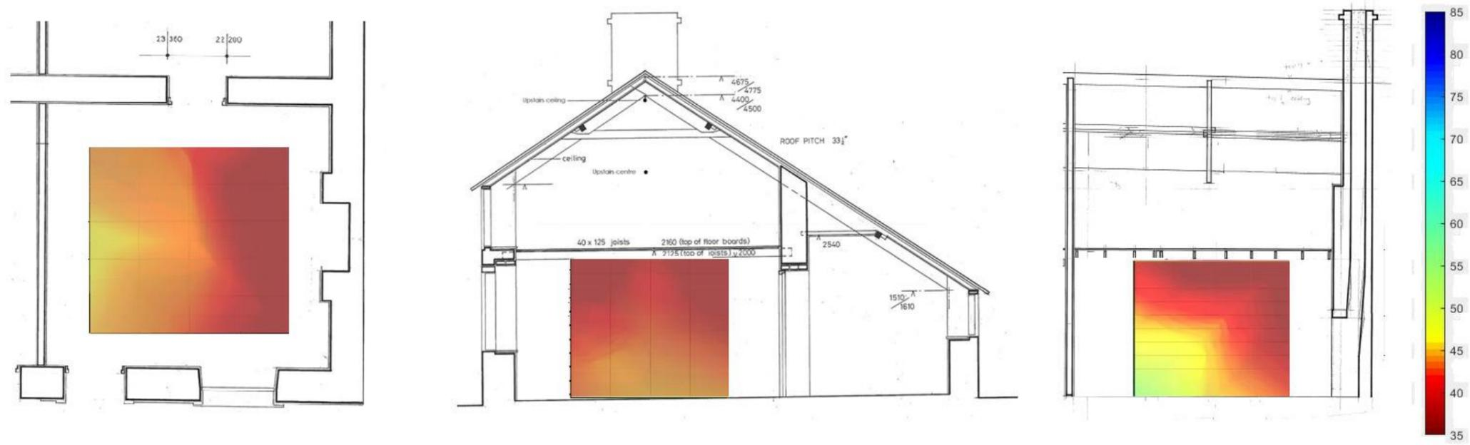
Figure 105: Cross-sectional image of RH distribution at 18:00 15/1/18 Experiment 5 Daily fire.
