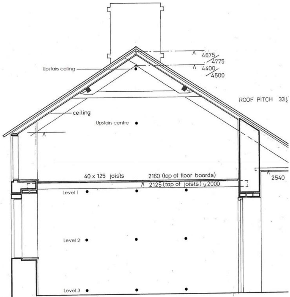
Figure 68: Data logger locations in elevation view.
