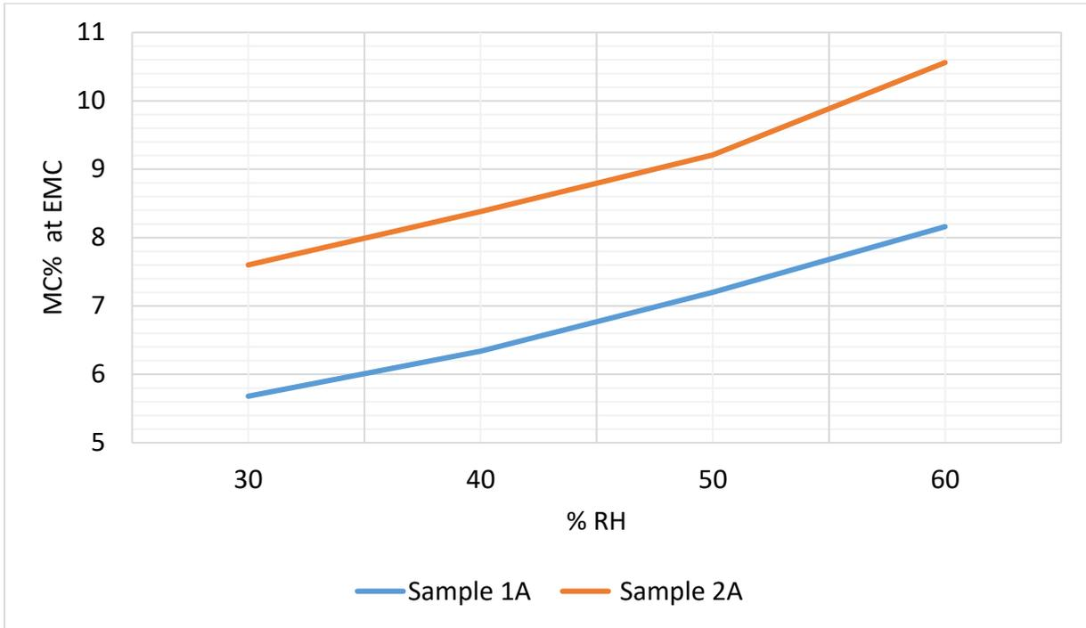
Figure 160: Equilibrium moisture content of timber samples 1A and 2A at 30, 40, 50 and 60% RH.
