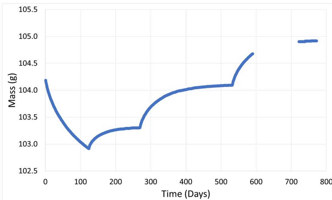
**Figure 156: showing sample 1A mass from the ambient room RH to 30% RH, 40%RH, 50%RH, 60%RH.**
