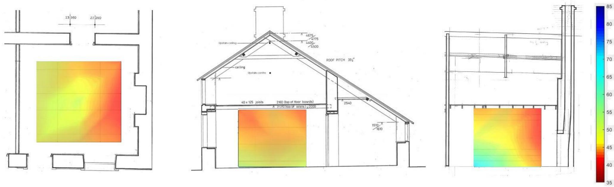
Figure 102: Cross-sectional image of RH distribution at 12:00 15/1/18 Experiment 5 Daily fire.
