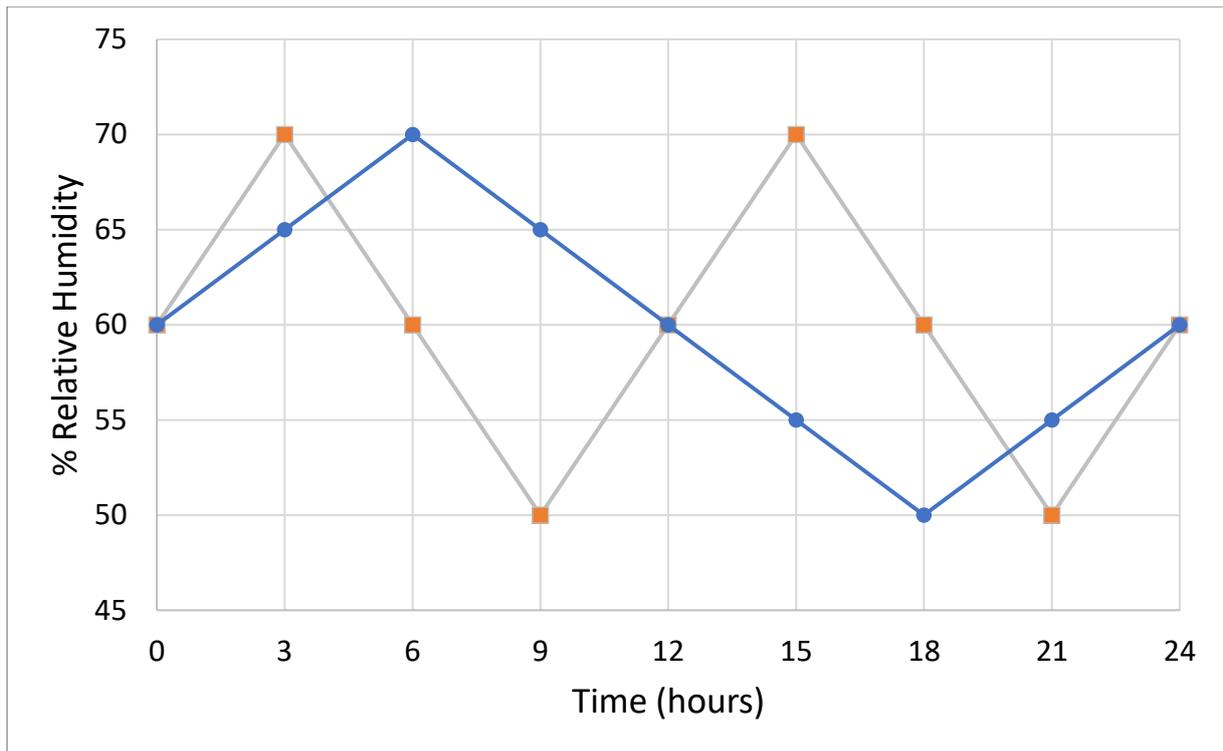
**Figure 167: Climate chamber set points for three (orange) and six (blue) hour fluctuations.**
