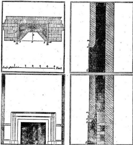
**Figure 22: Rumford's fireplace, top right showing before alterations (Rumford 1796).**
