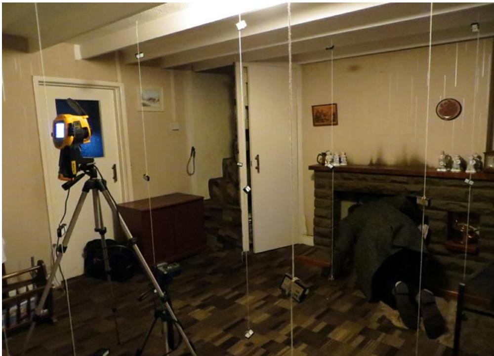
**Figure 73: Loggers on string, infrared camera and fireplace.**
