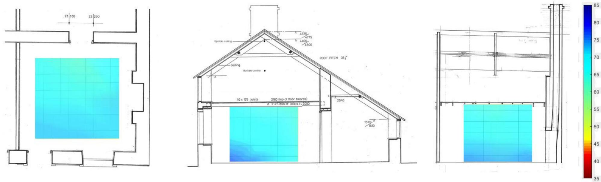
Figure 91: Cross-sectional image of RH distribution at 14:00 20/11/17 Experiment 1 Banked fire.
