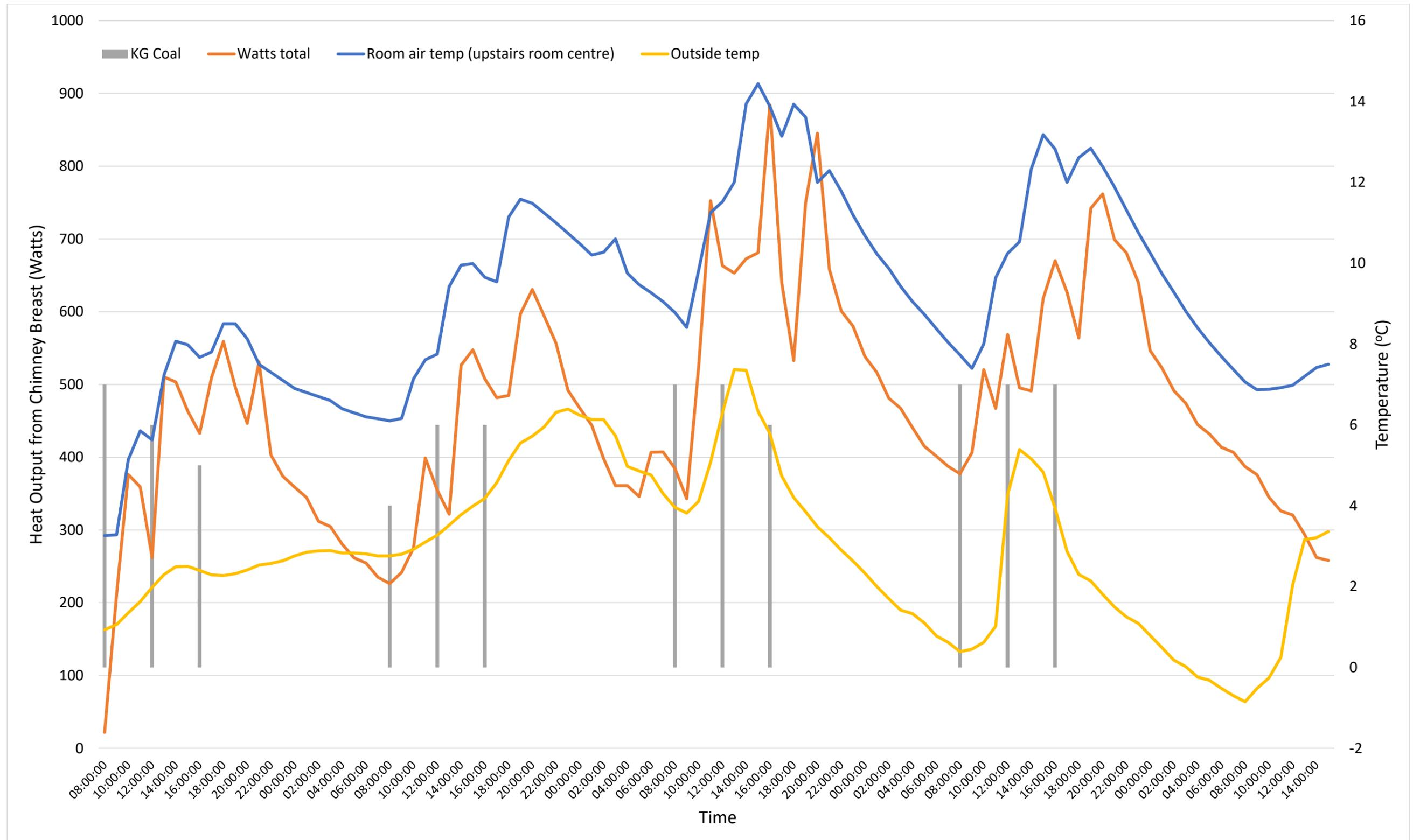
Figure 129: Watts output from chimney breast against room air temperature, outside temperature and coal consumption. Experiment 4, daily fires.
