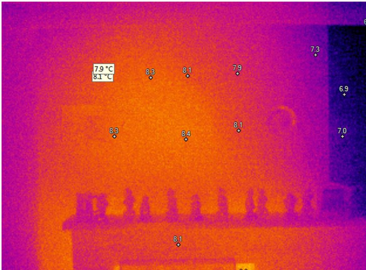
Figure 144: Chimney breast temperature three days after fire has gone out.
