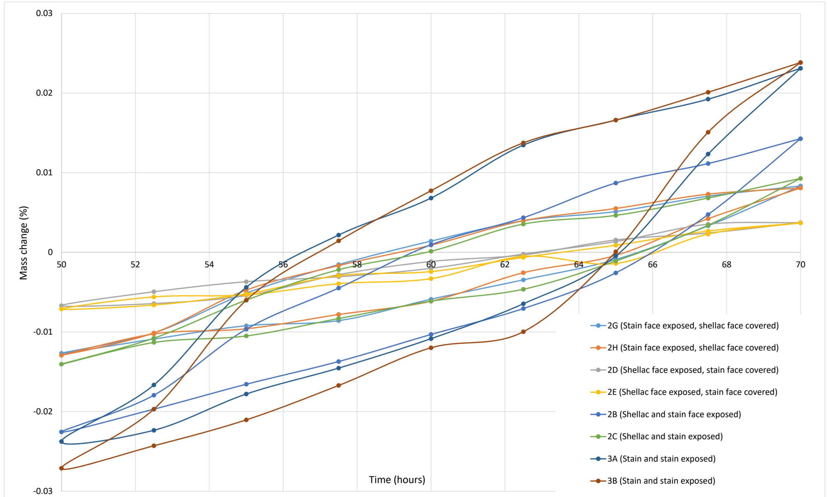
Figure 174: Hysteresis loop for six hour fluctuations, showing hourly percentage mass gain/loss at different RH points for samples.
