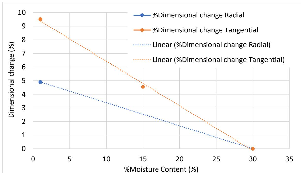
**Figure 52: Shrinkage of European oak, 30% to 12% Moisture Content tangential-7.5% radial-4%. 20% MC at 90%RH, to 12% 60% RH is tangential-2.5% radial-1.5% (Farmer 1972, 147).**
