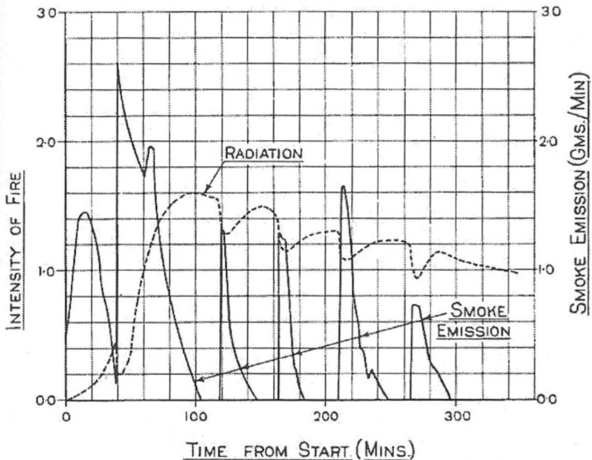
Figure 139: Radiant intensity from open fire against smoke emission (Blackie 1938, 24).
