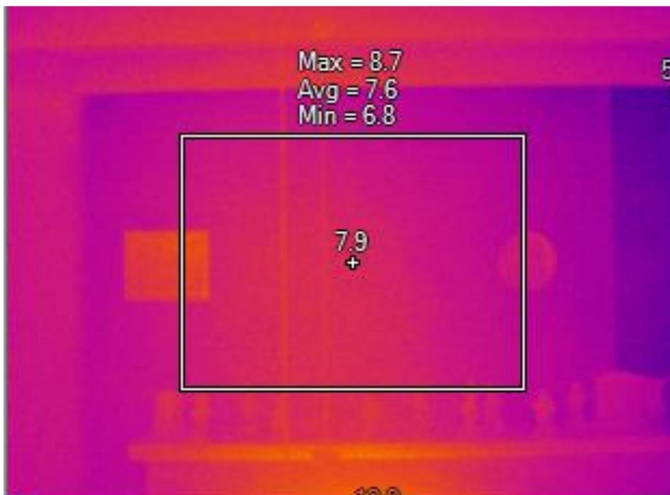
**Figure 79: Infrared image of chimney breast 8:39 1st day of Experiment 2 with the white box showing an average surface temperature of 7.6°C.**
