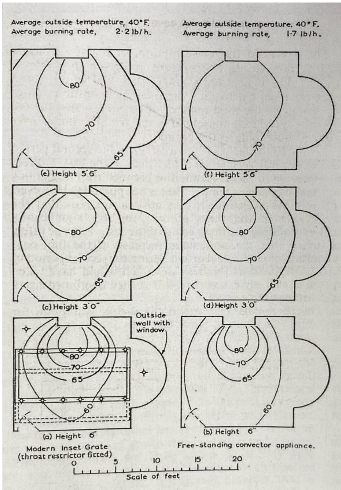
Figure 133: Isotherms of room heated for 10 hours by open fire (left) and convector heater (right) showing patterns of low temperature caused by windows are more stark with radiant heating. (Davidson 1955, 128).
