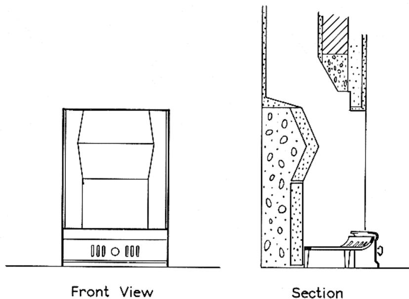
**Figure 6: Cross section of open fire with stool bottom grate, showing the refractory clay fireback with rubble infill behind, throat opening, splayed sides, smoke chamber and flue, (Venables 1957b, 10).**
