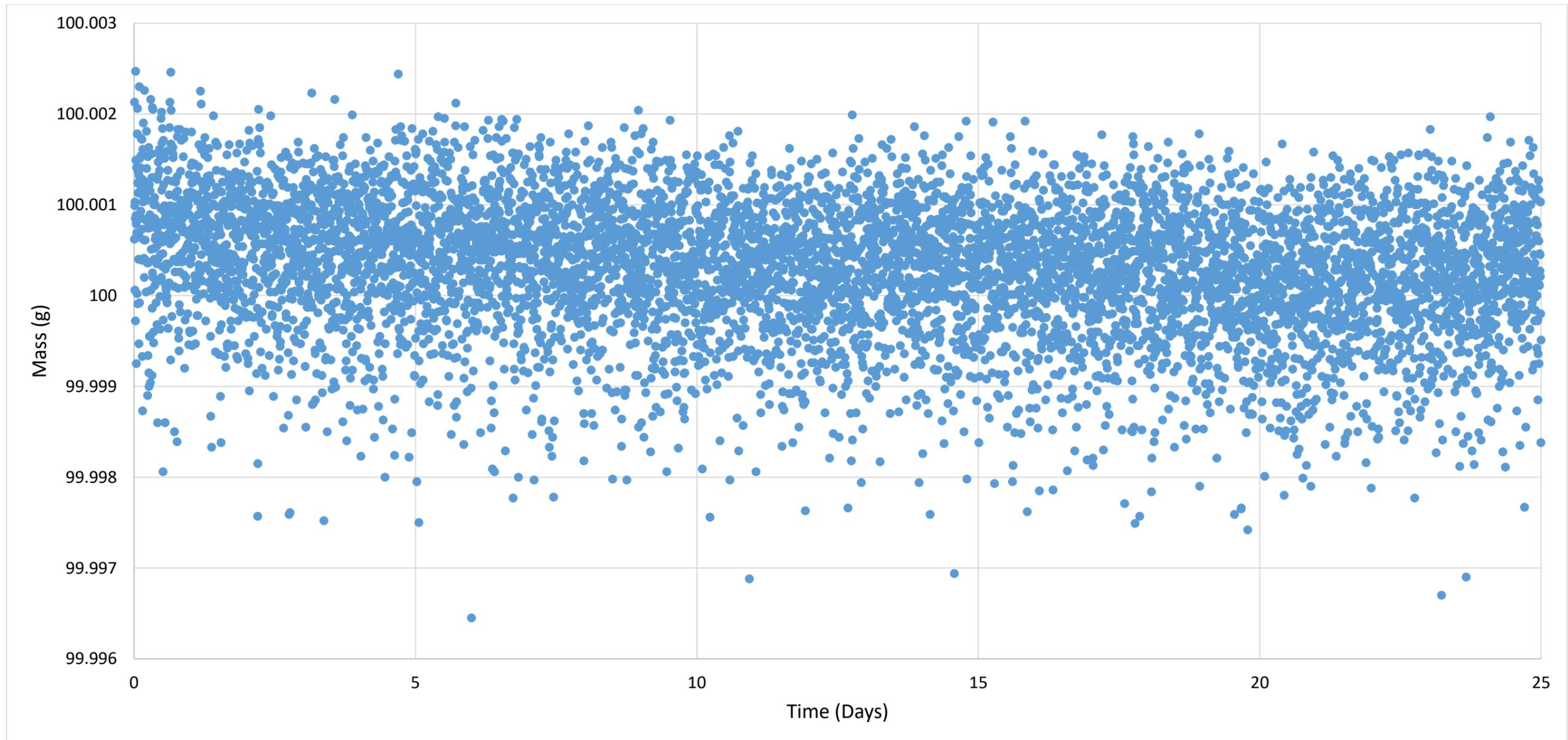
Figure 180: 100gram weight on balance in climatic chamber as experimental set up chapter 8.3. Three-hour fluctuations as described in chapter 8.5.1
