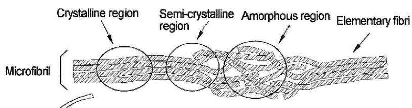
**Figure 44: Structure of microfibril proposed in (Stokke et al. 2006, 134).**
