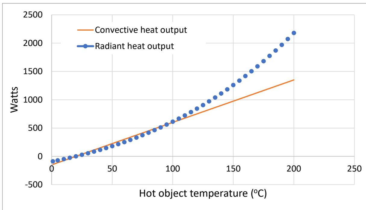
**Figure 141: Convective heat output and radiant heat output showing overview of outputs in watts against temperature 0-200°C, for a hot object with a surface area of 1m<sup>2</sup> and a background temperature of 20°C (convective heat transfer coefficient 7.5, emissivity coefficient 0.9)(CIBSE 2001,Web Reference 1).**
