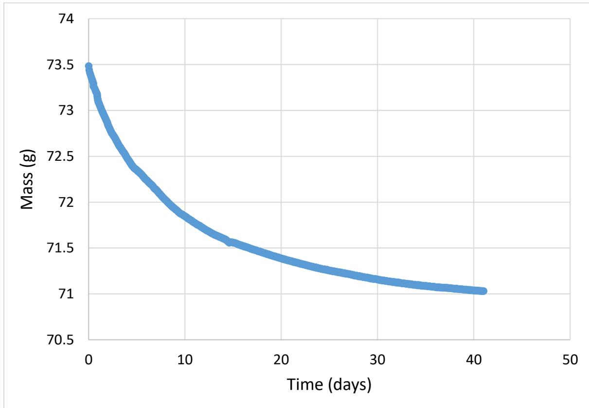
**Figure 179: Mass of timber Sample 2B (*Quercus robus*) when exposed to radiant heat source at background of 60%RH 14°C.**
