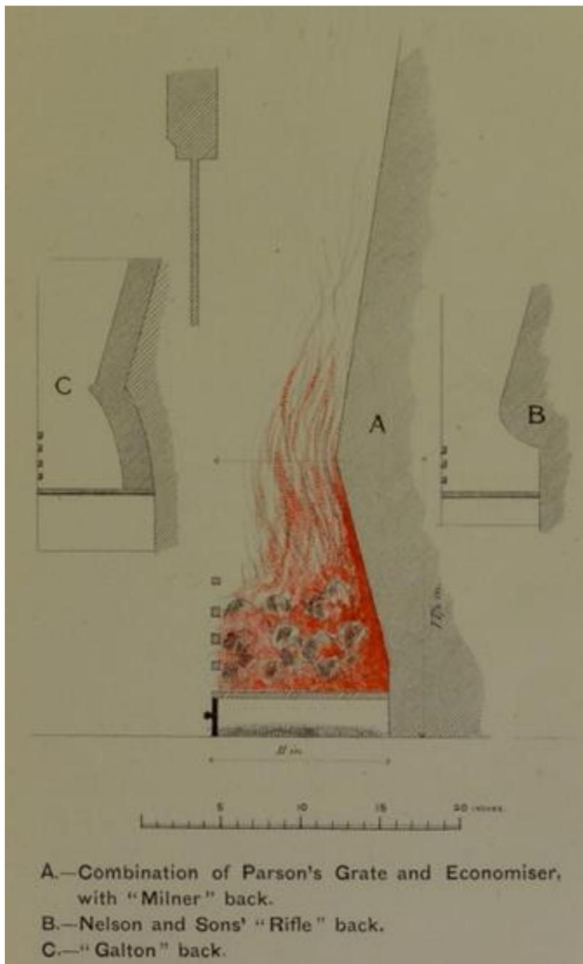
**Figure 24: Cross sections of Teale's improved grates, showing the minimal use of iron and use of fireback angles to minimise heat loss up the flue (Teale 1883, 37).**
