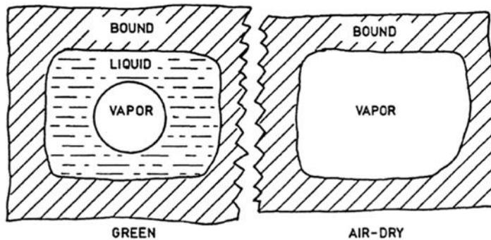
**Figure 48: Diagram showing three kinds of moisture in green wood, and two types in air-dry wood (Skaar 1988, 22).**
