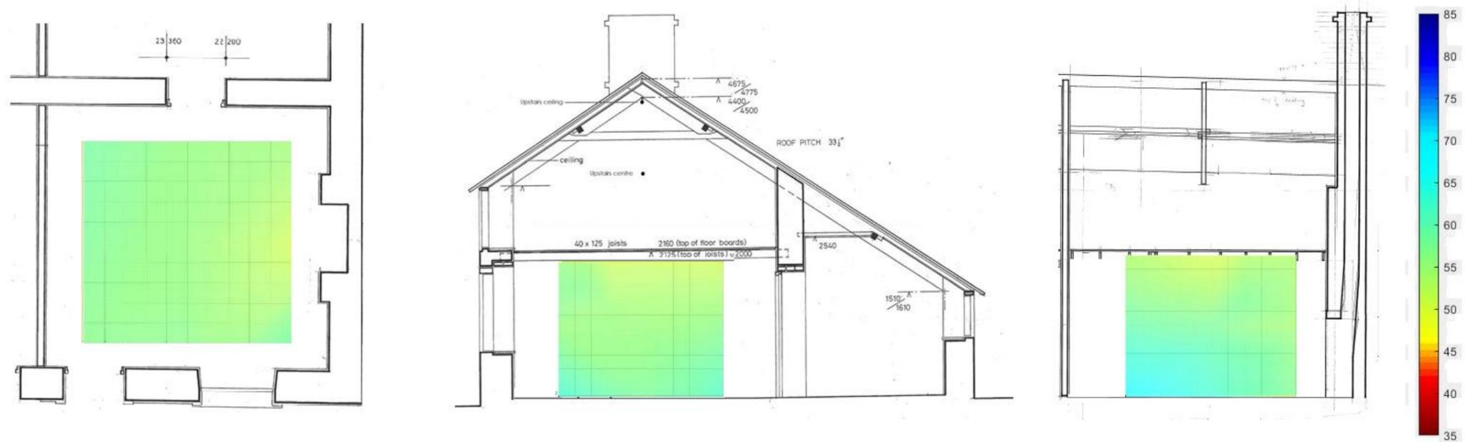
Figure 99: Cross-sectional image of RH distribution at 06:00 21/11/17 Experiment 1 Banked fire.
