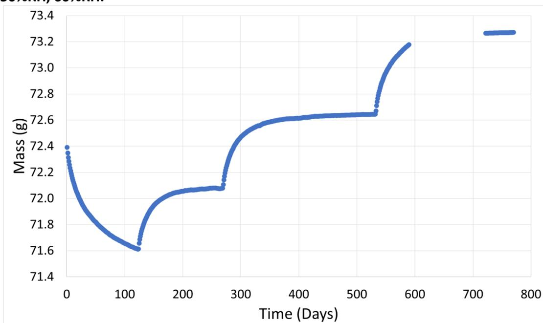
**Figure 157: showing sample 2A mass from the ambient room RH to 30% RH, 40%RH, 50%RH, 60%RH.**
