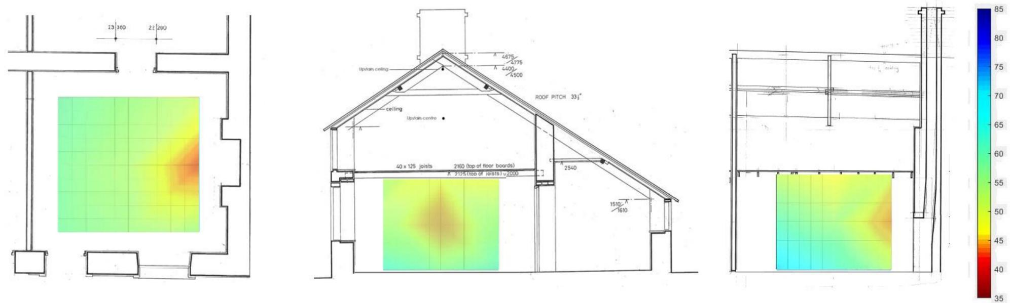
Figure 93: Cross-sectional image of RH distribution at 18:00 20/11/17 Experiment 1 Banked fire.
