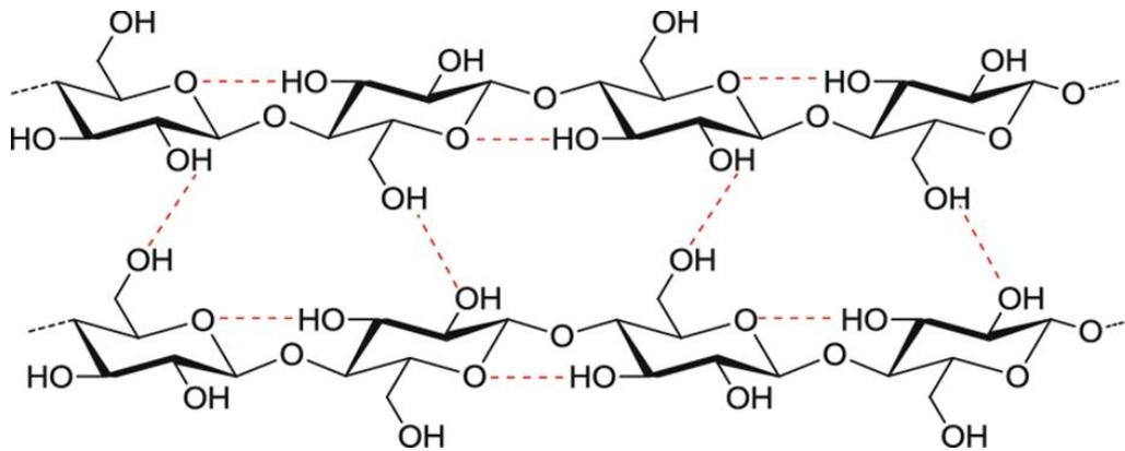
**Figure 45: Intramolecular and intermolecular H-bonding in cellulose (Pingping et al. 2015, 212).**
