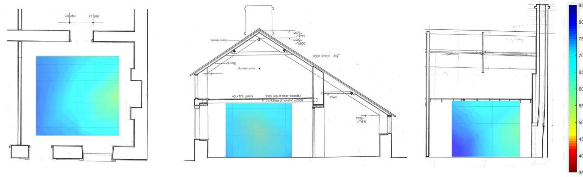
Figure 89: Cross-sectional image of RH distribution at 10AM 20/11/17, Experiment 1 Banked fire.
