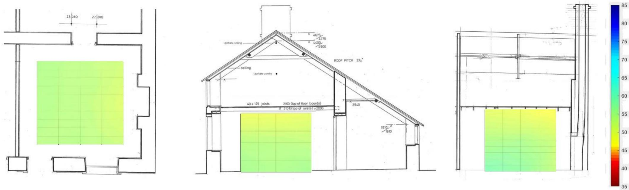
Figure 110: Cross-sectional image of RH distribution at 04:00 16/1/18 Experiment 5 Daily fire.
