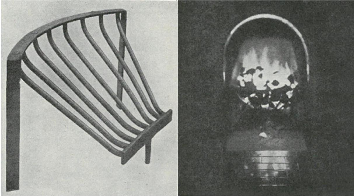
**Figure 65: A grate for burning anthracite in an open fire; note the deep fuel bed and wide firebars ensuring little ash build up and a higher surface area of fuel to air (Bedford 1948, 256-257).**
