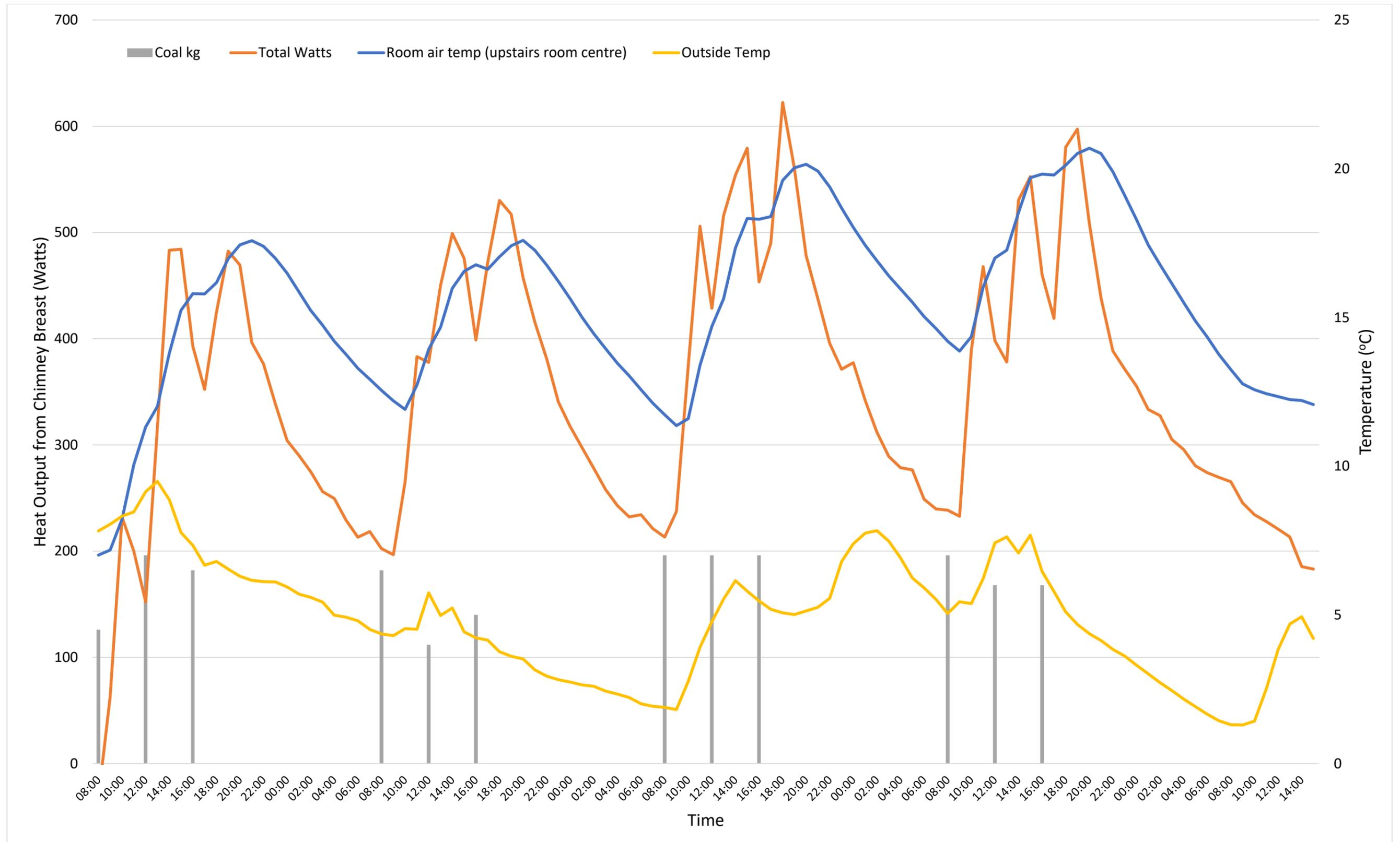
Figure 130: Watts output from chimney breast against room air temperature, outside temperature and coal consumption. Experiment 5, daily fires.
