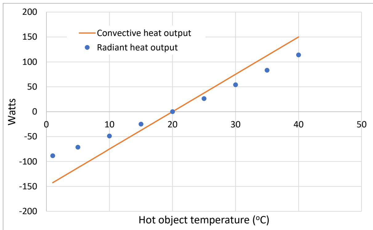
**Figure 142: Convective heat output and radiant heat output showing overview of outputs in watts against temperature 0-40°C, for a hot object with a surface area of 1m<sup>2</sup> and a background temperature of 20°C (convective heat transfer coefficient 7.5, emissivity coefficient 0.9) (CIBSE 2001, Web Reference 1).**
