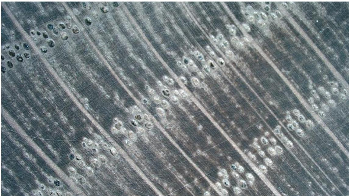
**Figure 43: Cross section of oak sample from St Fagans, showing how lumen size changes seasonally. Also showing medullary rays at near ninety degrees to growth rings.**
