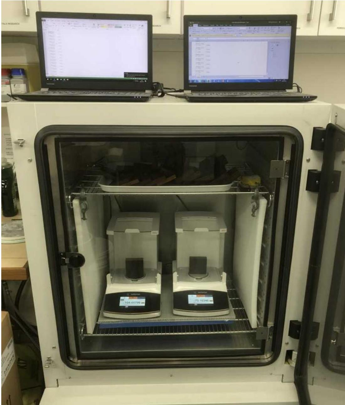
**Figure 155: Experimental set up, Sample 1 and 2A in the climatic chamber on balances, with remaining samples above on tray.**
