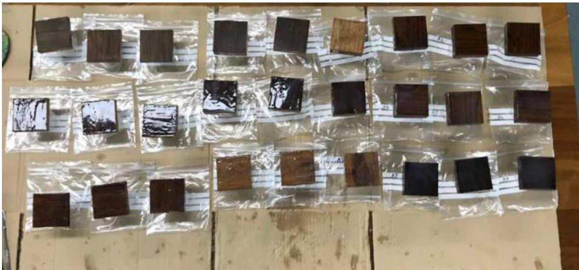
**Figure 154: Samples during coating with two-part silicone.**
