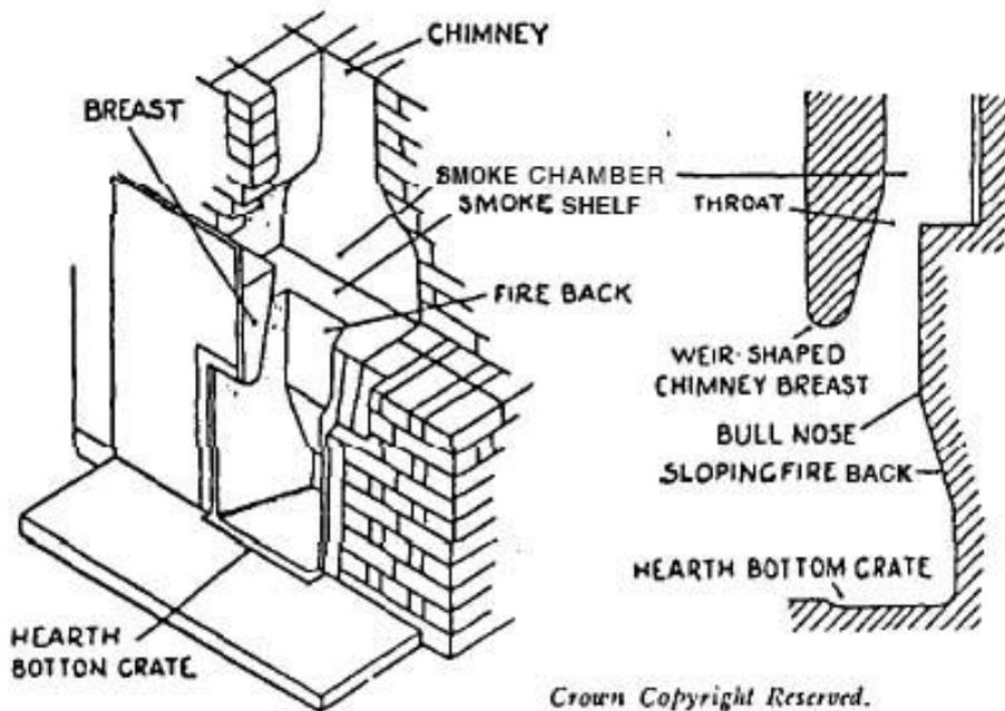
**Figure 7: A detailed overview of the parts of the fireplace, however no grate is shown (Rosin et al. 1939,8).**
