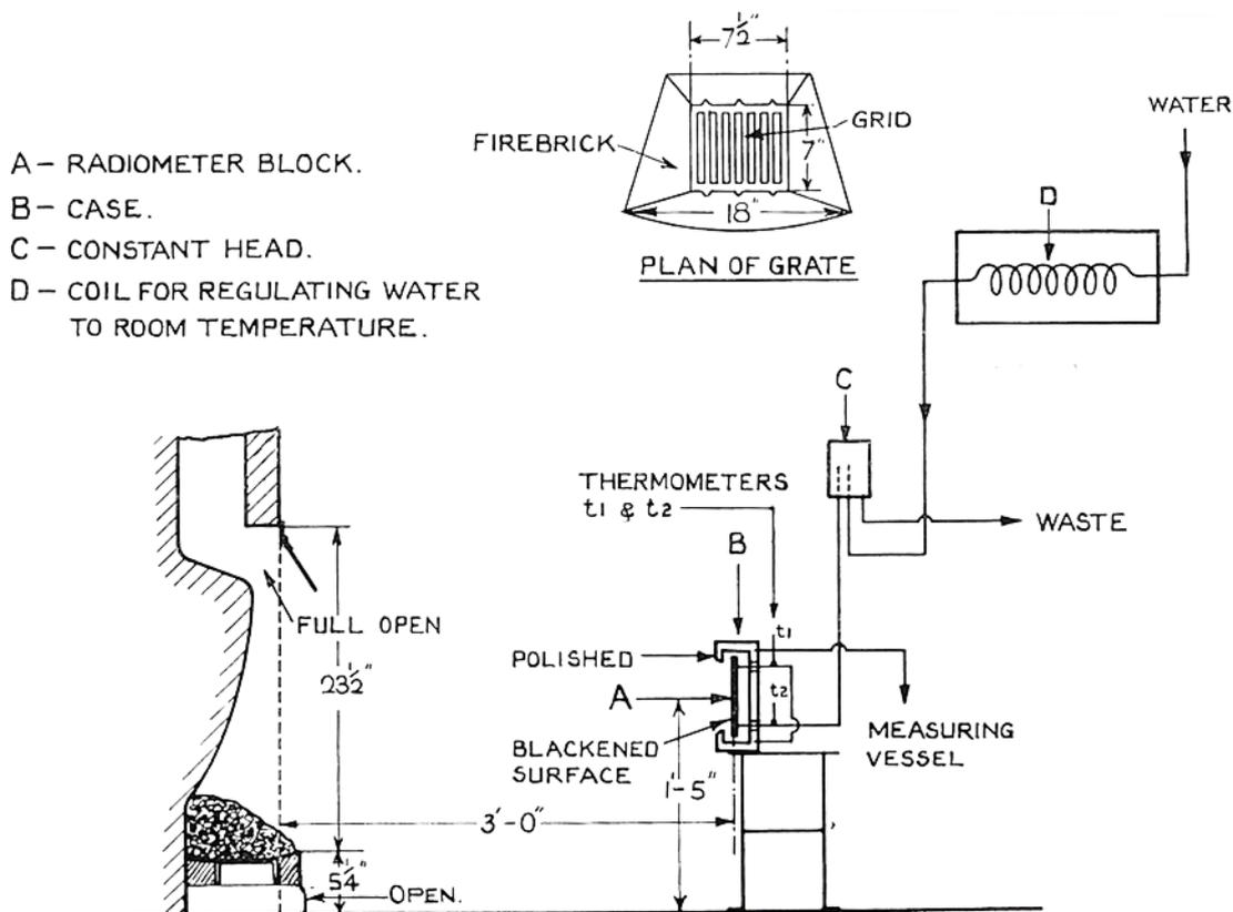
**Figure 32: Fireplace and apparatus for measuring radiant heat output (Blackie 1938, 21).**
