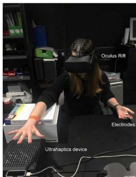
Figure 4. Experimental setup encompassing the UltraLeap device, Oculus Rift and Biopac electrodes
