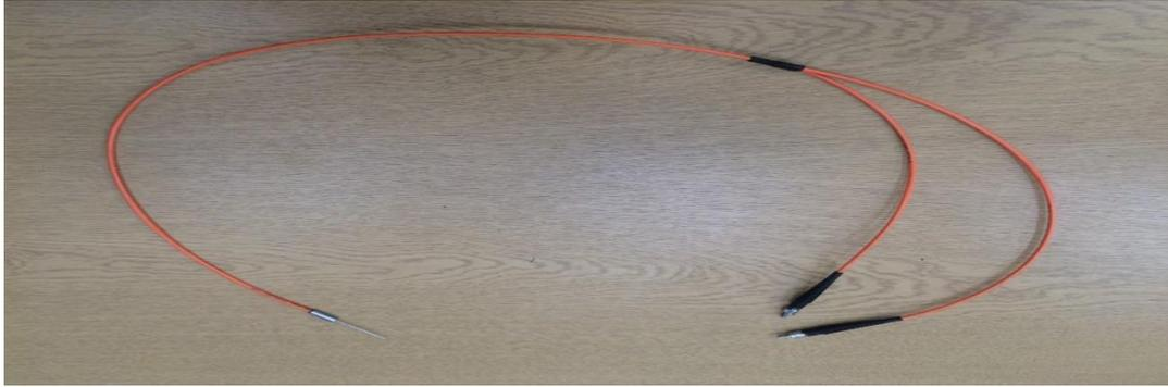
Figure 4-4: The physical optical probe
