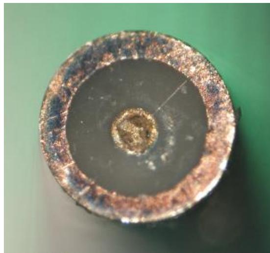
Figure 8-22: Coated flat coaxial cable with Au.
