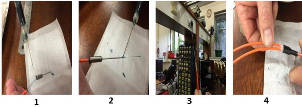
Figure 4-1: Fabrication steps 1-Gluing two fibre optics after adjacent both of them.2- Glue and house the adjacent fibres in a rigid stainless steel needle.3- drying all gluing parts.4- Fix and separate two fibres, one as a source and the second as a receiver.
