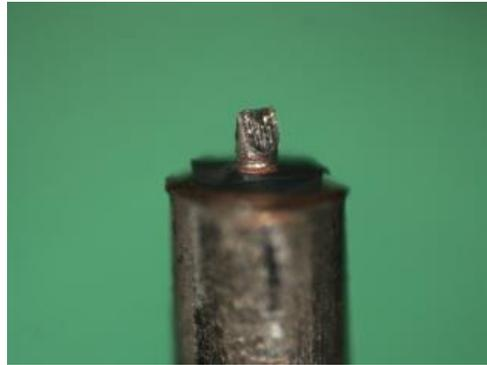
Figure 8-1: Protruding probe 'cut back'
