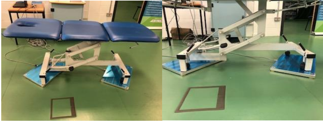
Figure 4. 1 Plinth mounted onto 2 portable force plates to record vertical GRF.
