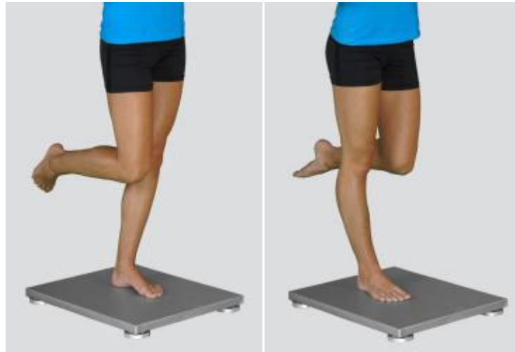
Figure 4. 2 The single leg stance test, on either left or right foot placed in the centre of the plate with normal upright position (image from Kistler MARS Software v2.1 Manual).
