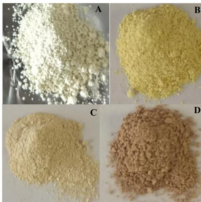
Appendix 6.12. UiO-66(Zr)-NH<sub>2</sub> MOFs before (fresh, A) and after undergoing STS with methanol (B), ethanol (C), and water (D) solvents. Images obtained from post-STs reactions carried out by Justyna Minkiewicz.
