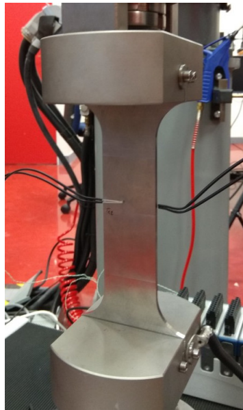
Figure 1. Experimental configuration of a PVR test with two thermocouples.
