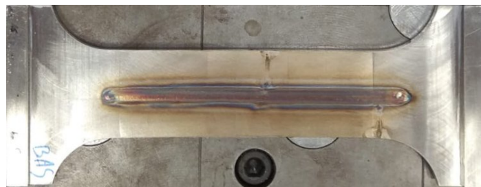
Figure 3. Welded PVR specimen after the experiment.
