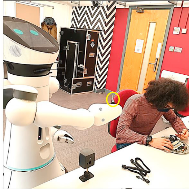
Fig. 6. In a human-robot teaming scenario, Care-O-bot 4 offers using of screwdriver to the human teammate.
