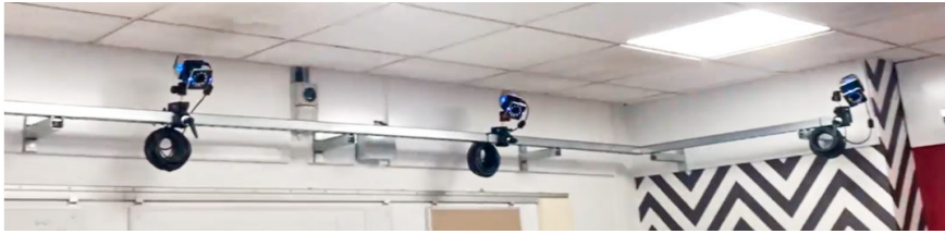
Fig. 3. Vicon motion tracking system mounted all around the laboratory.
