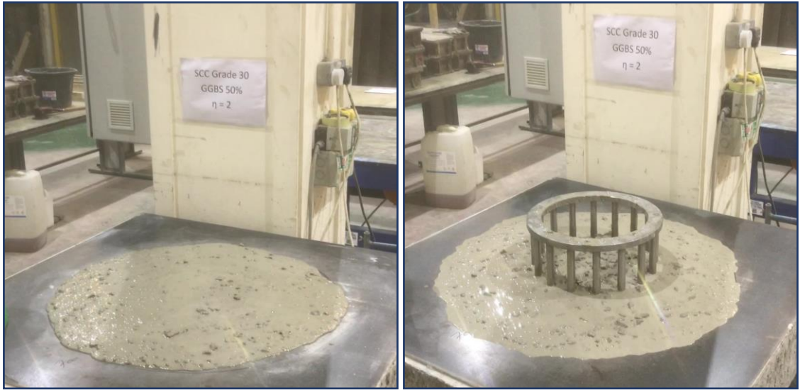
Figure 7.6 Slump and J-Ring final horizontal spreads for mix C1 2
