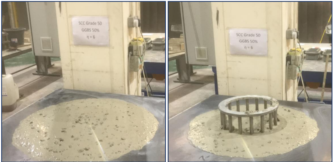
Figure 7.7 Slump and J-Ring final horizontal spreads for mix C3 2
