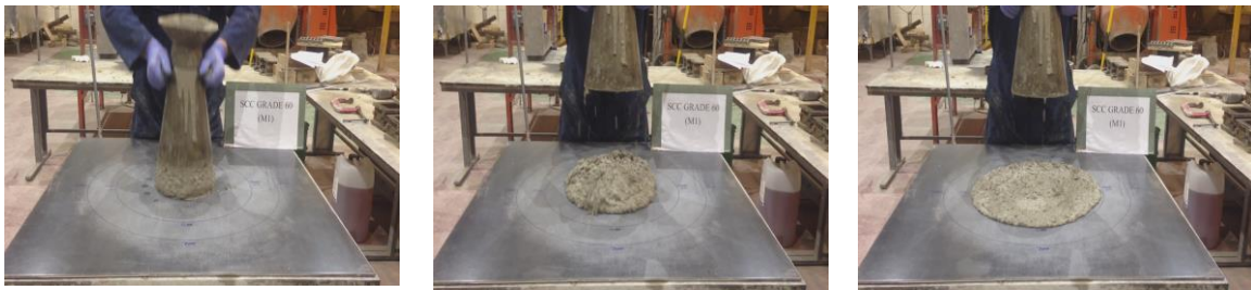
Figure 3.2 Video images of the slump cone test at three flow stages
