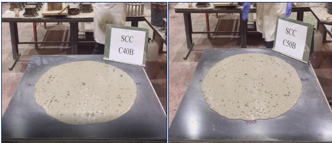
Figure 7.2 Horizontal spread of SCC mix when it stopped to flow
