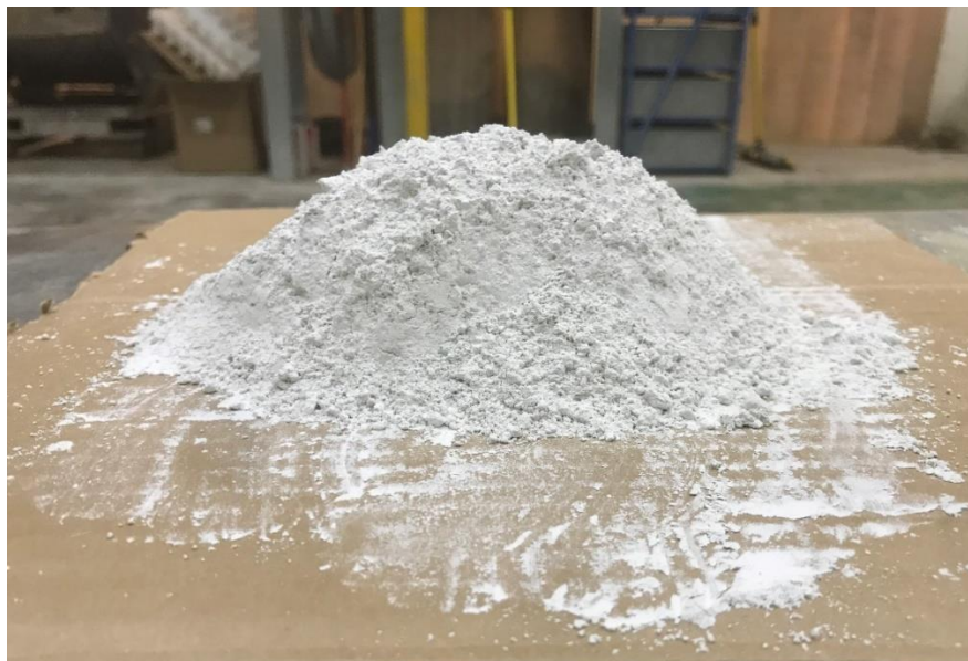
Figure 2.6 Physical appearance of ggbfs used in current study 2021
