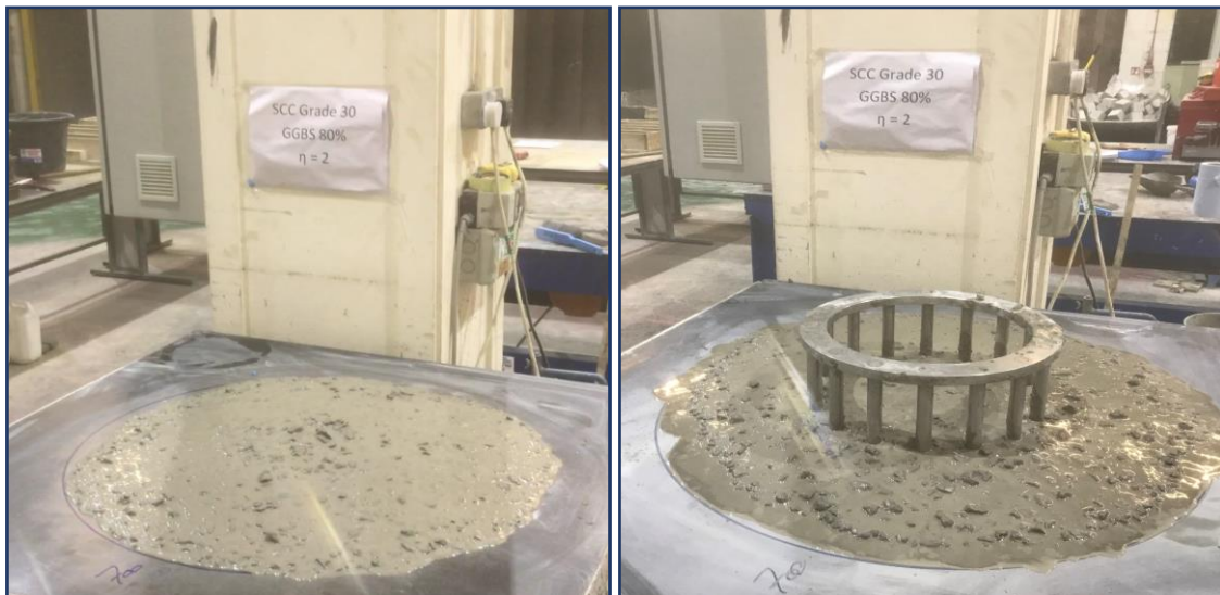
Figure 7.9 Slump and J-Ring final horizontal spreads for mix F
