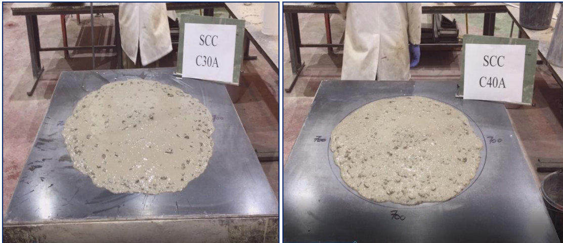
Figure 7.2 Horizontal spread of SCC mix when it stopped to flow
