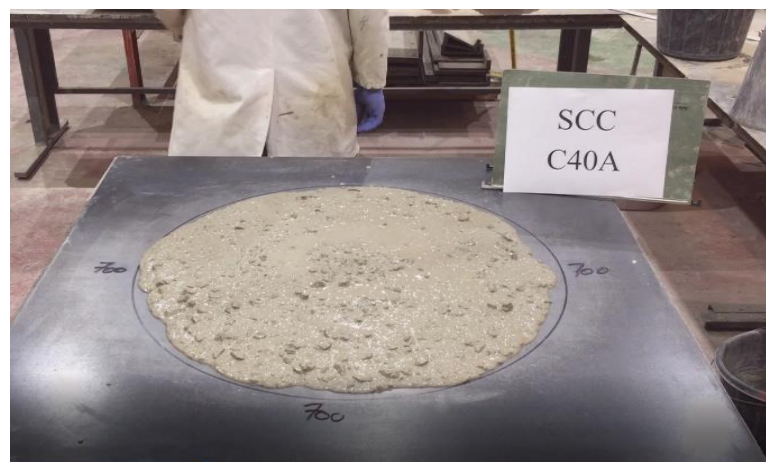
Figure 3.4 Flow-ability test (cone)
