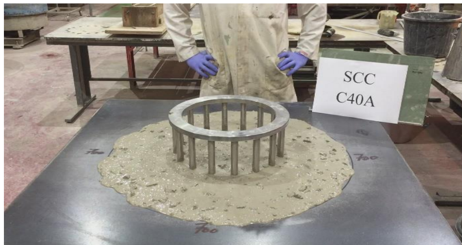
Figure 3.6 Passing-ability test (J-ring)
