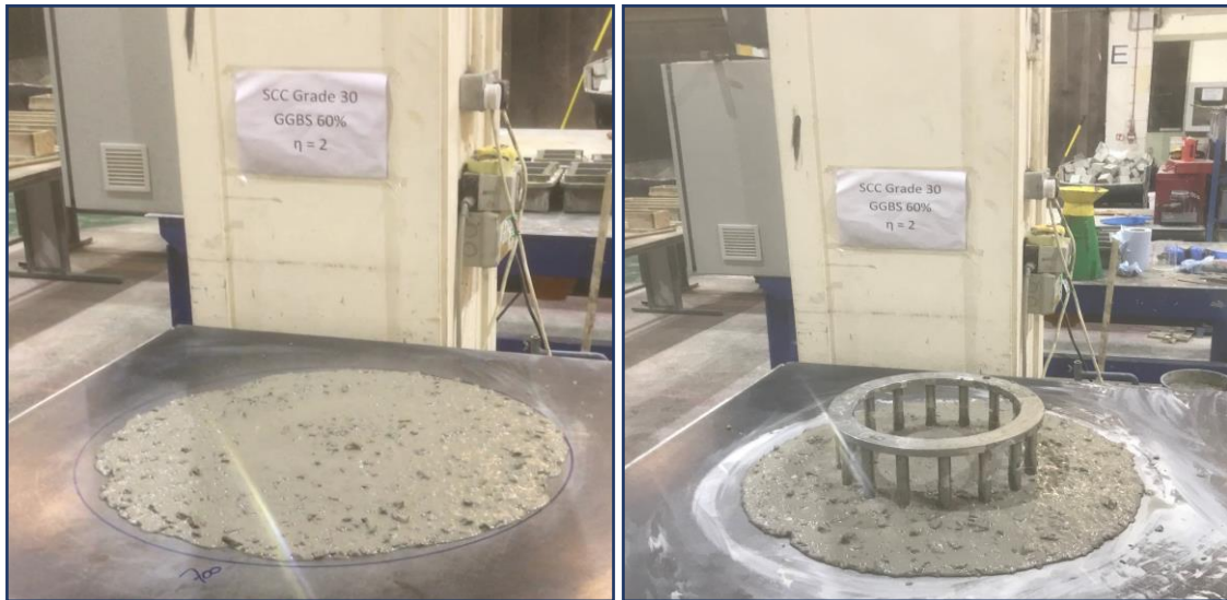
Figure 7.8 Slump and J-Ring final horizontal spreads for mix D1
