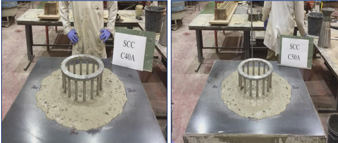
Figure 7.4 J-Ring final horizontal spread of SCC mix
