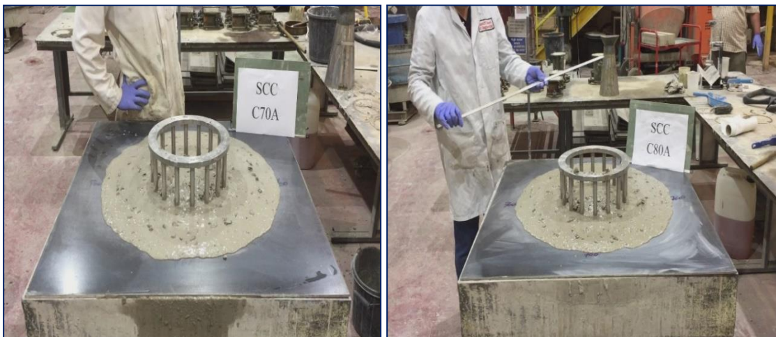
Figure 7.4 J-Ring final horizontal spread of SCC mix
