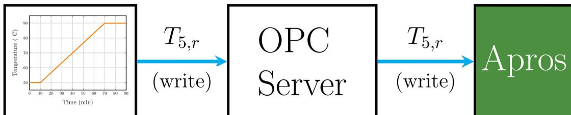
Figure 5.27: Block diagram of the co-simulation between MATLAB/Simulink-Apros.
