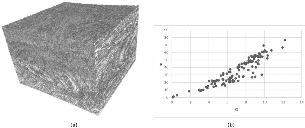
Figure 4.4: Testing on a glass fibre reinforced composite material. (a) 3D image of a glass fibre reinforced composite material. 970 × 1469 × 1217 and  $\kappa$  for each subsample  $\mathcal{X}_1$  voxels, spacing: 4 $\mu$ m.
