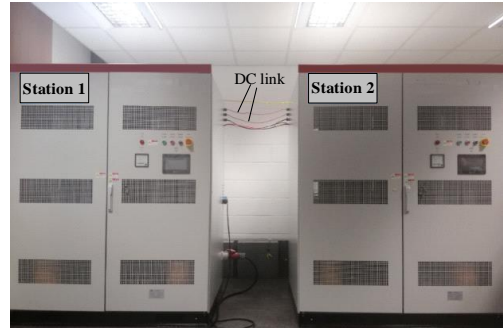
Fig. 20. Lab-scaled MVDC platform.
