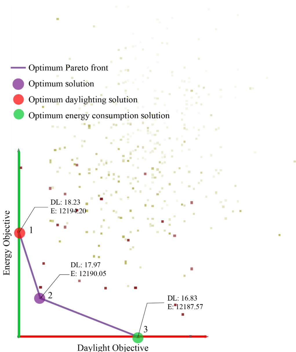
Figure 6.27: Pareto front and genomes generations produced in Octopus for Jeddah
