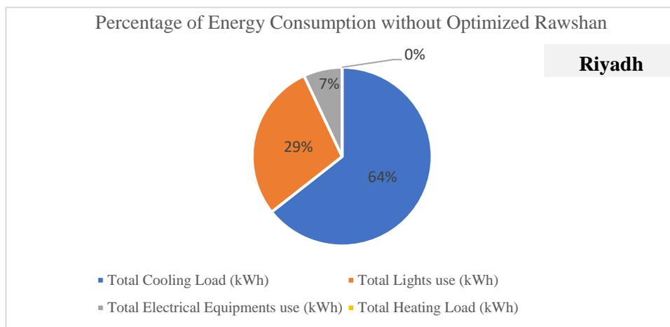
Figure 5.12: Energy Usage Percentages for Riyadh Climate Simulation
