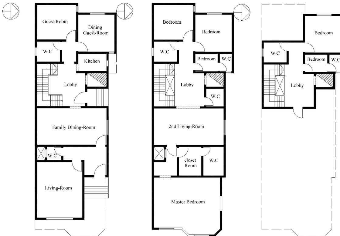
Figure 3.8: Ground floor plan, first floor plan, and second floor plan (from left to right)
