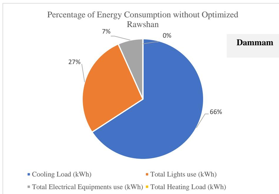
Figure 5.14: Dammam Energy Consumption and UDLI Predictions without a Rawshan
