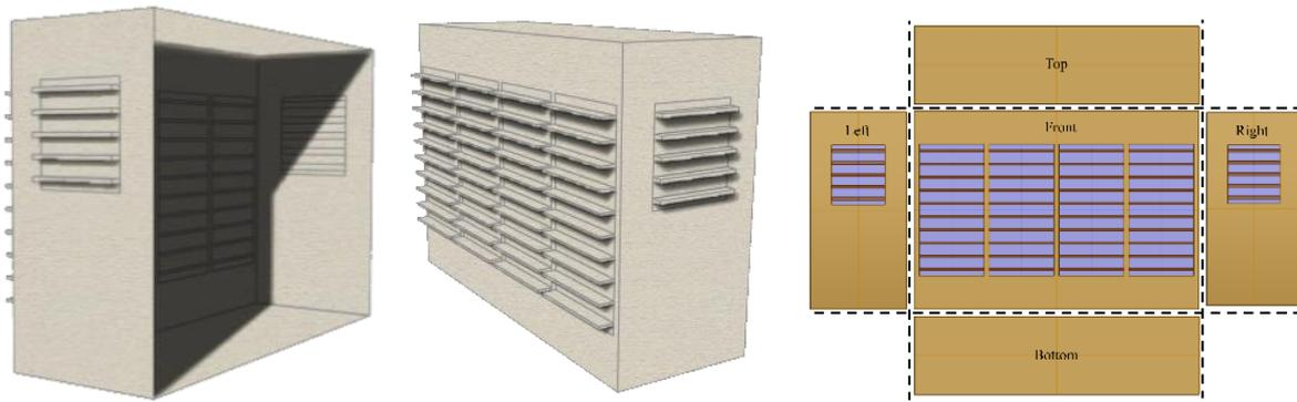
Figure 3.19: Standard Rawshan Element; from the left to right hand figures show the Rawshan from interior, exterior, and the Rawshan's sides
