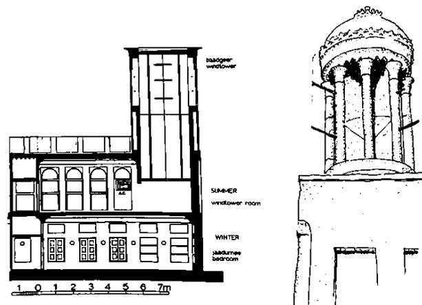
Figure 2.3: A cross-section and perspective diagram of a windcatcher. Source: (Ragette 2003)
