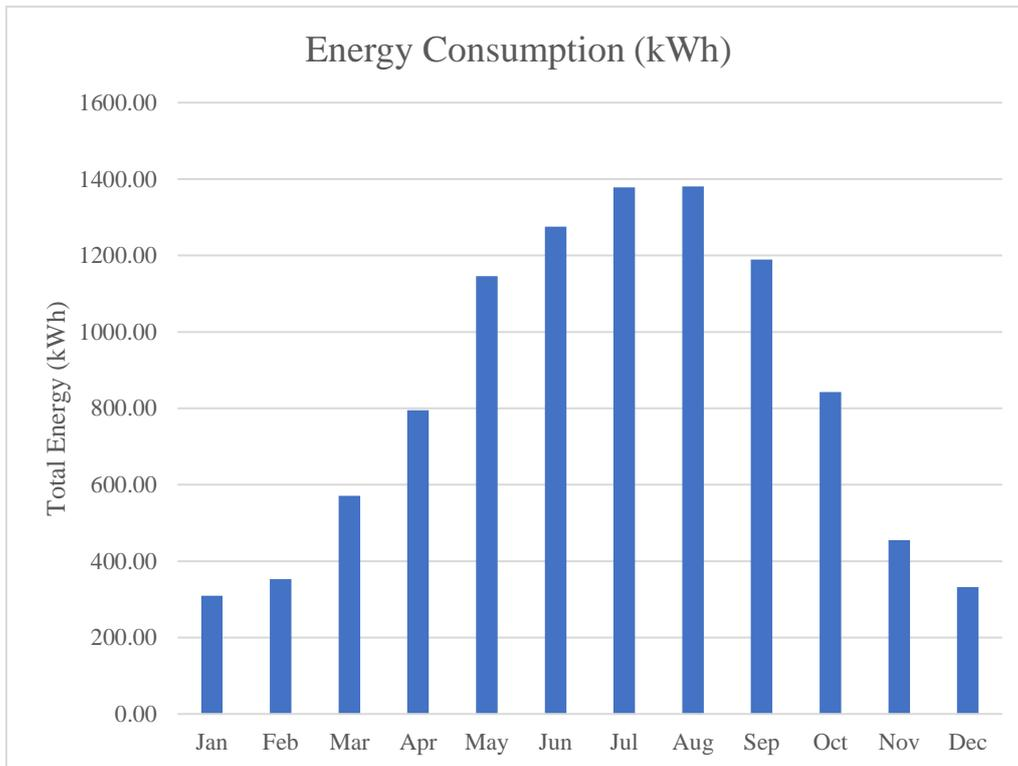
Figure 6.9: Monthly Energy Consumption with Optimized Rawshan for Riyadh
