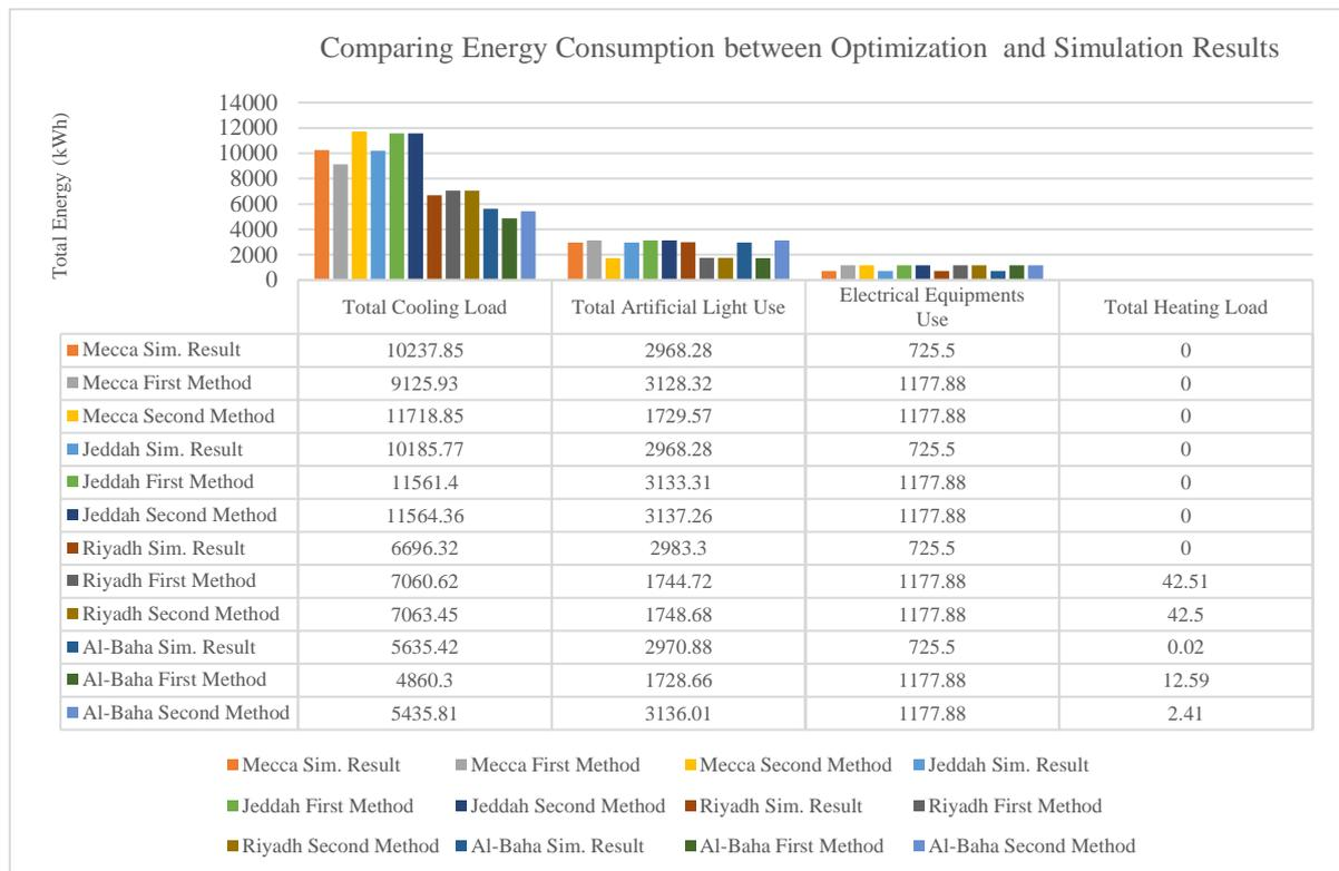
Figure 7.9: Comparison of Energy Consumption between the Optimization and Simulation Results for the Four Cities using the First and Second Method
