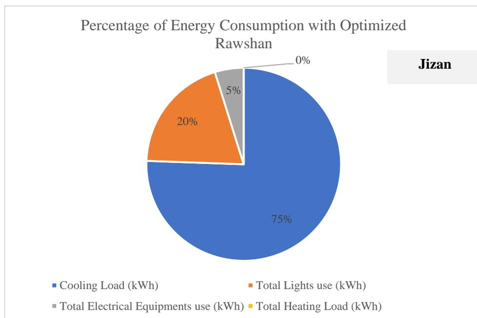
Figure 5.15: Energy Usage Percentages for Jizan Climate Simulation
