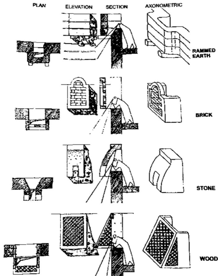
Figure 2.7: Arrangement of loopholes. Source: (Ragette 2003)
