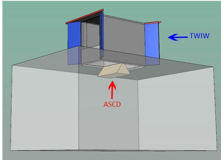
Figure 2.12: Two-sided Windcatcher integrated to Wing Wall (TWIW) and the anti-short-circuiting device (ASCD) Source: (Nejat et al. 2016)
