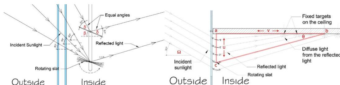
Figure 2.15: Cross-sectional view of the room showing the incident sunlight reflected by the rotating slats to a fixed position on the ceiling. Source: (Eltaweel and Su 2017)
