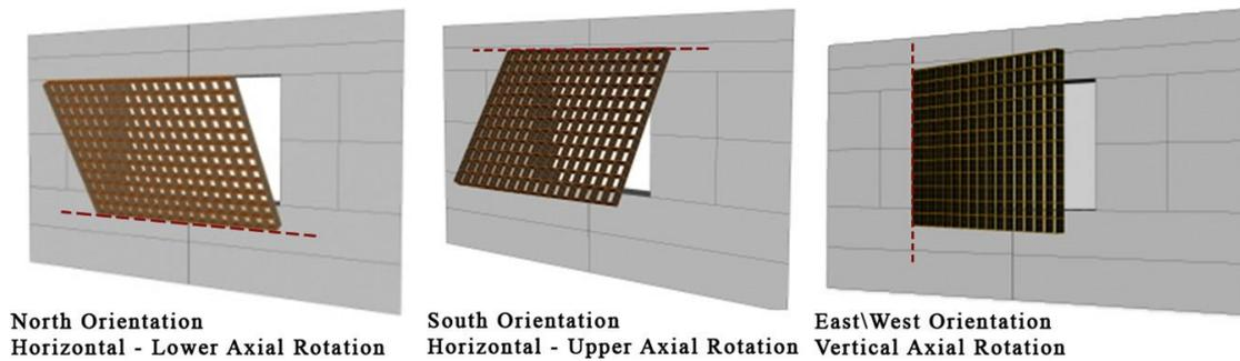
Figure 2.16: Type of solar screen orientations. Source: (Sherif, Sabry et al. 2012)
