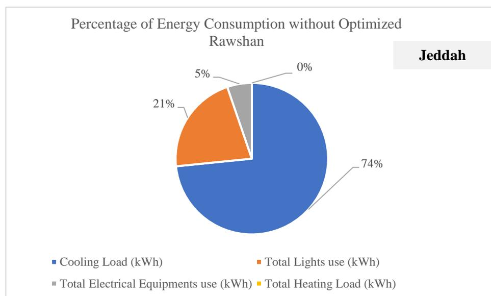
Figure 5.11: Energy Usage Percentages for Jeddah Climate Simulation
