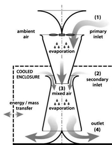
Figure 2.10: A section and perspective of a wind-catcher. Source: (Pearlmutter et al. 1996, da Silva et al. 2006, Erell et al. 2008)
