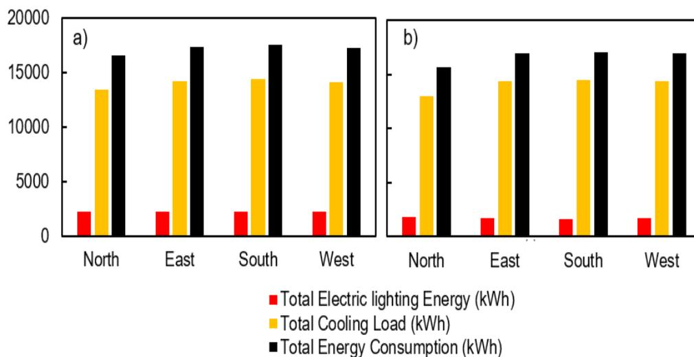
Figure 5.7: a comparison between both cases; a) with the Rawshan, b) without the Rawshan showing that less cooling load in east and west direction when the Rawshan is used.
