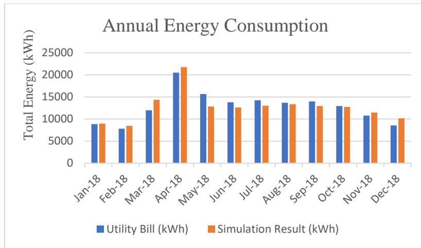
Figure 5.9: Annual Energy Consumption in kWh: Comparing the Simulation with Monthly Utility Bills
