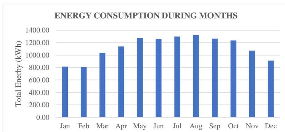
Figure 6.5: Monthly Energy Consumption with Optimized Rawshan for Mecca
