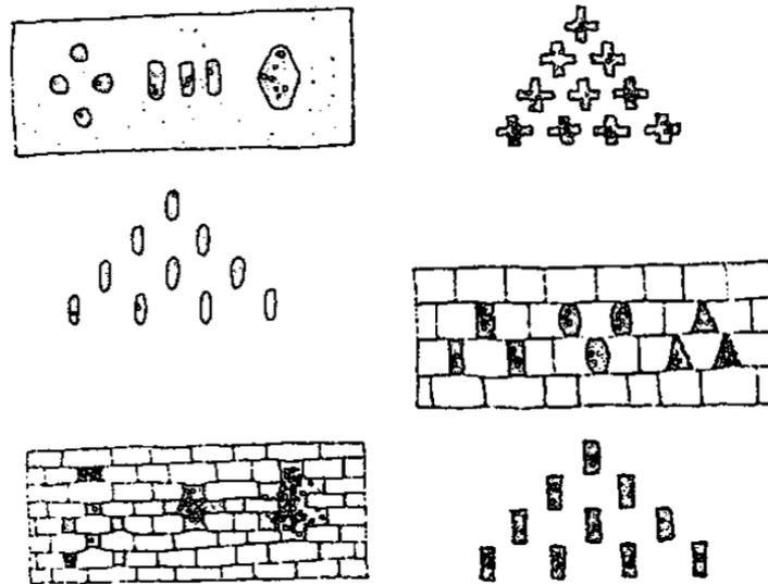
Figure 2.6: Arrangement of loopholes. Source: (Ragette 2003)
