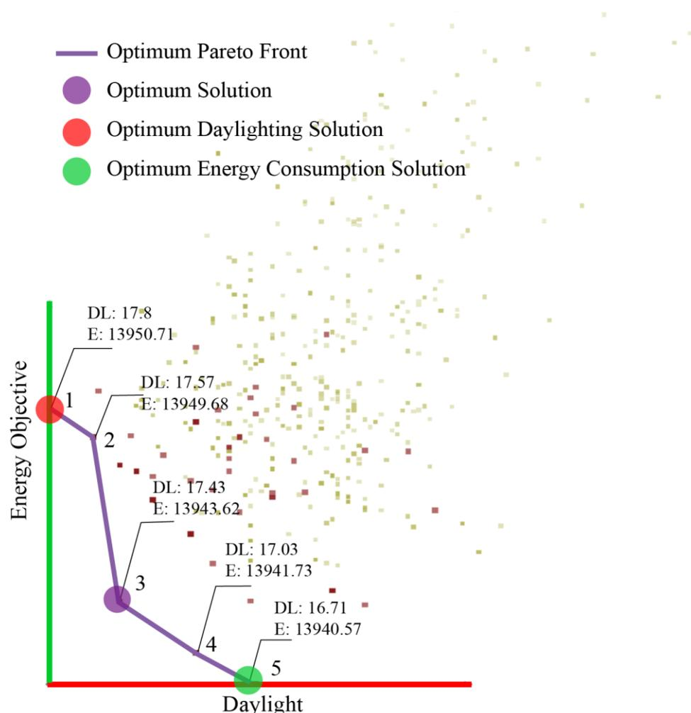
Figure 6.31: Pareto Front and Genome Generations Produced in Octopus for Jizan
