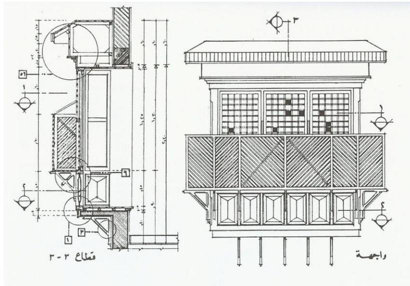
Figure 2.9: The Rawshan dimension details. Source: (Koshak and Gross 1998)
