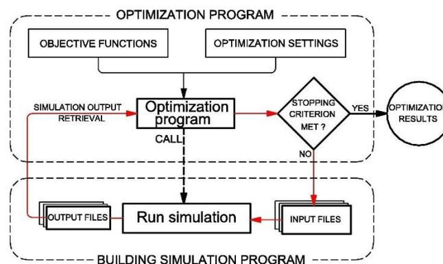
Figure 2.19: The coupling loop applied to simulation-based optimization in building performance studies. Source (Nguyen, Reiter et al, 2014)
