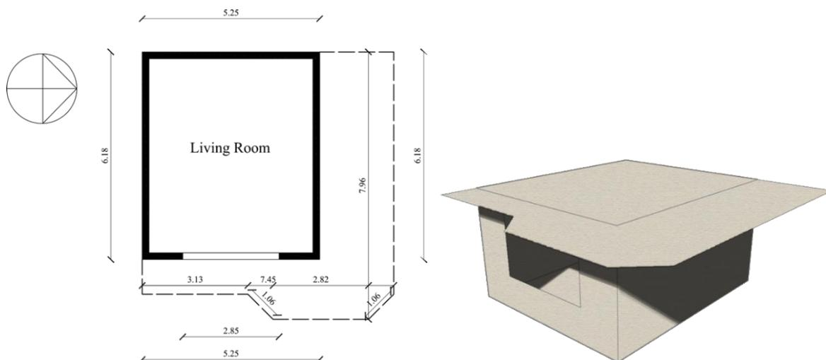
Figure 3.18: Living Room Plan and 3D Schematic without Rawshan
