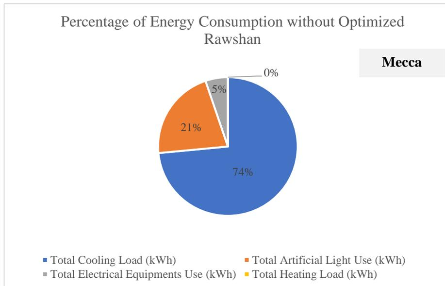
Figure 5.10: Energy Usage Percentages for the Mecca Climate Simulation
