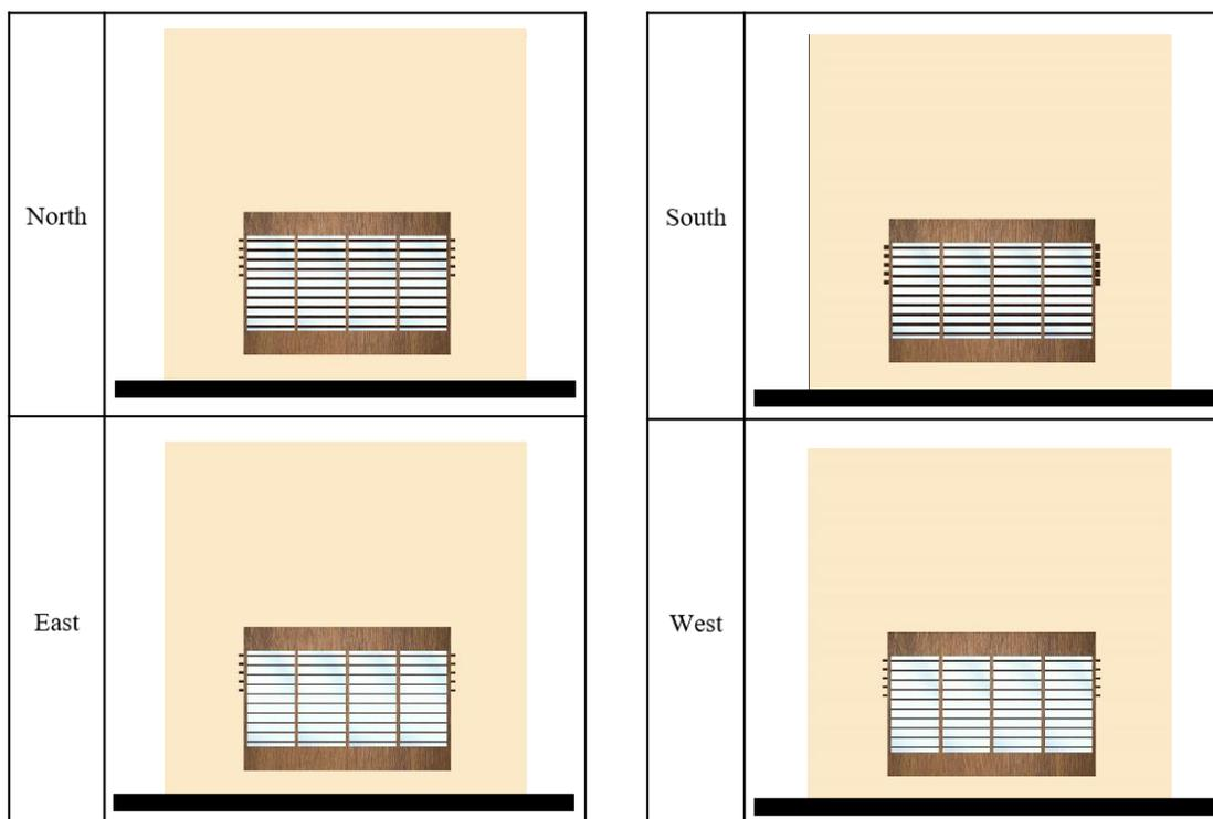
Figure 2.17: Type of the optimized Rawshan for the 4 directions
