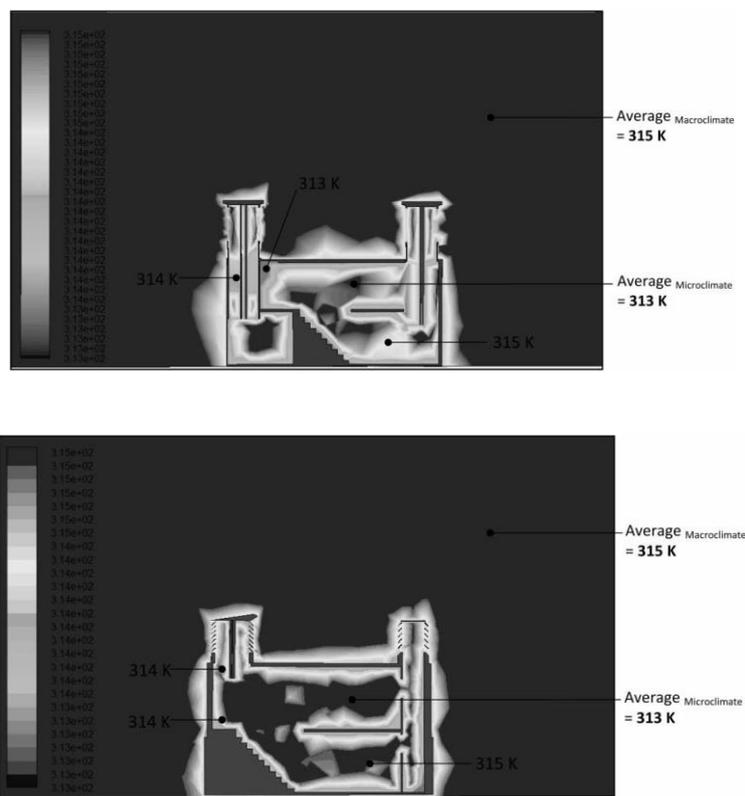
Figure 2.13: Comparing the traditional windcatcher and modified windcatcher
