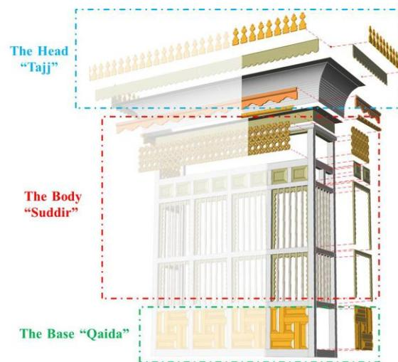
Figure 4.3: The Rawshan construction. Source: (Baik et al. 2014)
