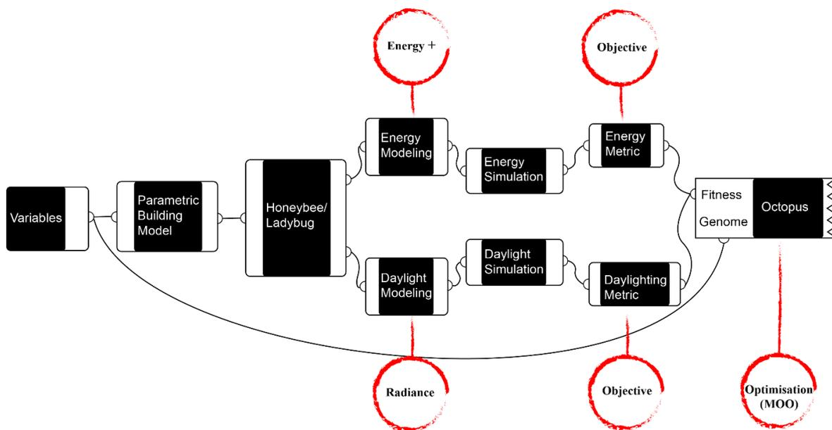
Figure 3.23: Energy and daylight optimization processes and tools for multi-objective optimization
