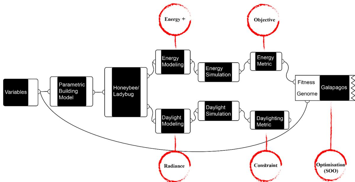
Figure 3.22: Energy and daylight optimization process and tools for single-objective optimization
