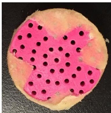
*Figure 4-16. Photograph showing a perforated disk - following use within column to contain sand and to ensure even flow of cementation medium through the column, with layer of glass wool beneath which sits between the sand column and disk.*
