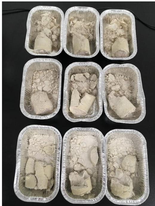
*Figure 7-13. Photograph of columns from Test P2 following UCS2 and oven drying at 105°C.*
