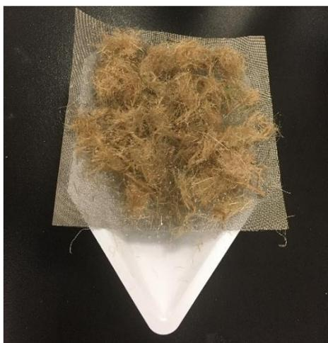
Figure 4-13. Photograph showing 1 g of jute fibres resting on gauze, after the fibres have been sprayed with concentrated cementation medium.
