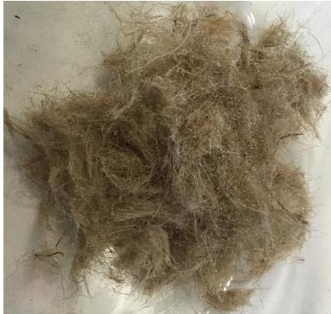
*Figure 4-12. Photograph showing jute fibres, after they have been loaded with concentrated cementation medium, dried and then separated by hand.*
