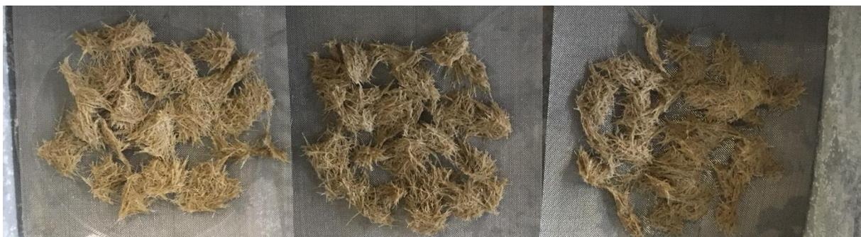
*Figure 4-11. Photograph showing a triplicate set of hemp fibres, after they have been soaked in concentrated cementation medium, transferred to gauze and dried, prior to mixing with sand for use in column studies.*
