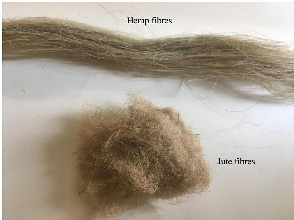
*Figure 4-7. Photograph of hemp and jute fibres used in experiments – prior to cutting and washing.*
