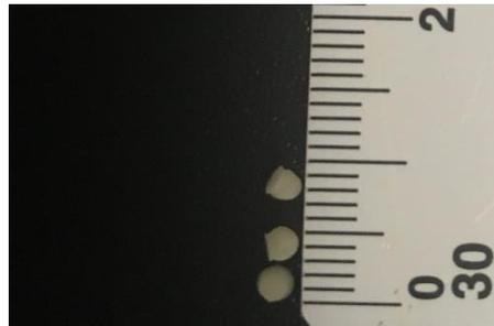
Figure 8-3. Dried alginate- based hydrogel beads encapsulating cementation medium.
