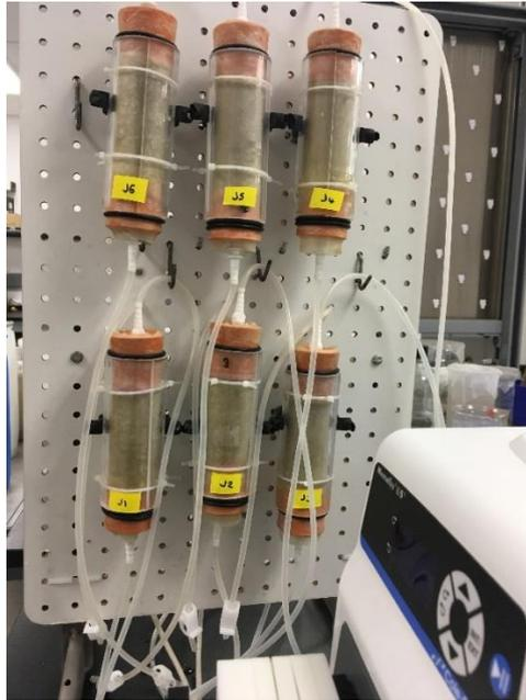
*Figure 7-1. Photograph of prepared columns, showing apparatus used for the column studies completed at Arizona State University.*
