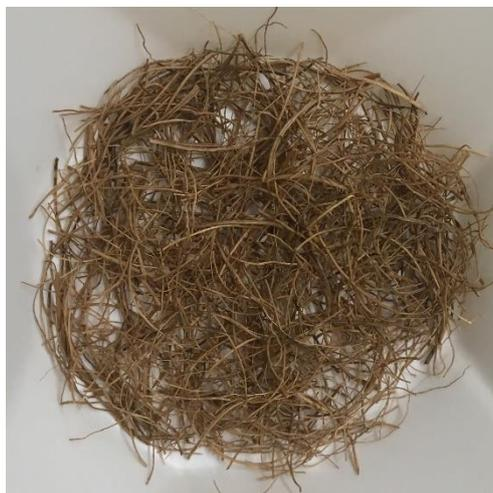
*Figure 4-8. Photograph of coir fibres used in experiments.*
