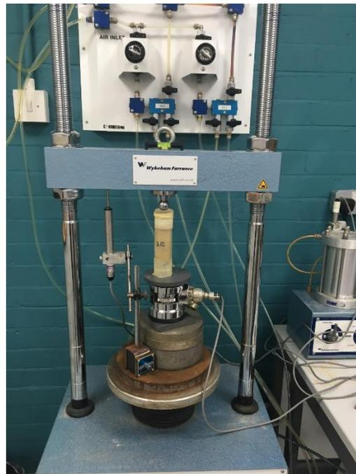
*Figure 6-2. Photograph of the unconfined compression test apparatus used at Cardiff University, showing a column from Columns Test U2 being subjected to loading.*
