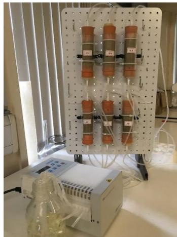
Figure 6-1. Photograph of prepared columns, showing apparatus used for the column studies completed at Cardiff University.
