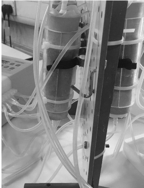
*Figure 4-15. Photograph of assembled sand columns attached to the front and back of the column frame in sets of triplicates, while cementation medium is being injected into the base of the columns using a peristaltic pump.*
