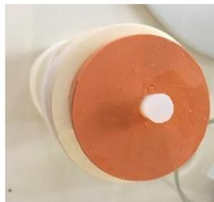
*Figure 4-17. Photograph showing the inlet end of a column during assembly, with silicone plug inserted into the inlet hole within the bung to prevent the cementation medium draining during filling of the column.*
