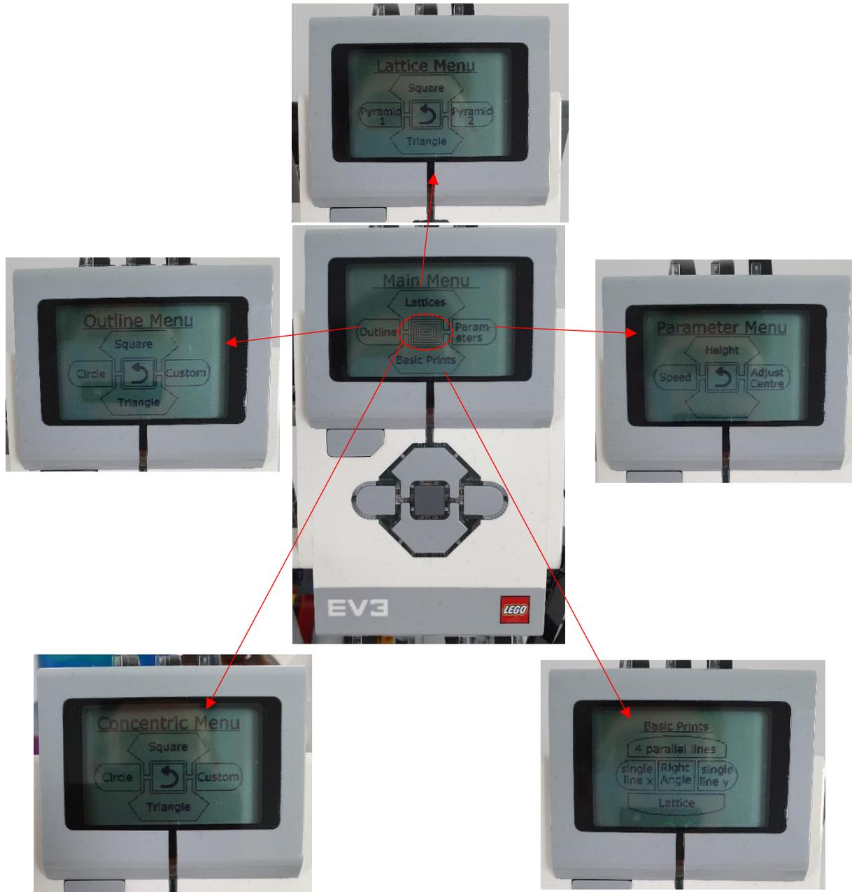
**Figure 5.7 Main menu interface of the LEGO® x/y/z stage as shown on the EV3 programmable brick.**
