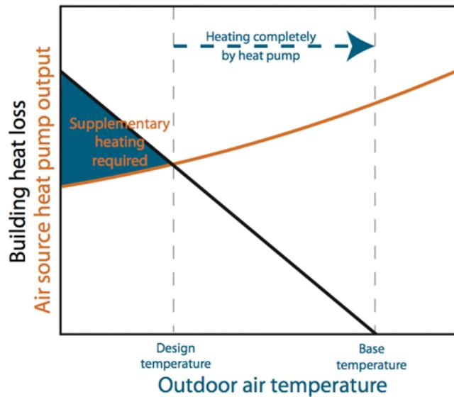
Figure 4-11: Operation of an ASHP and supplementary heat source at various OATs (source: figure from [67])
