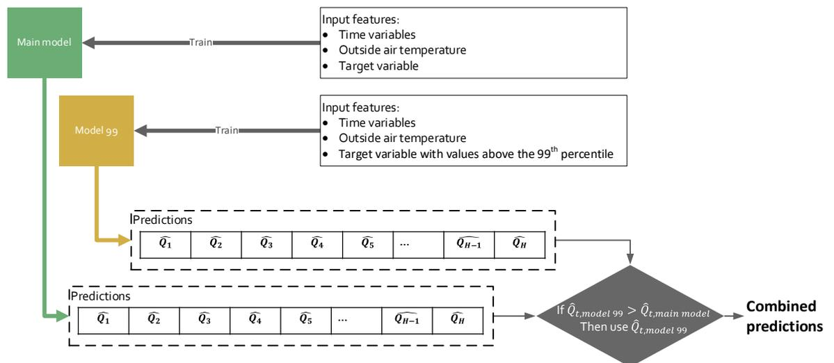
Figure 4-4: Flow chart of an example model that combines the predictions of two sub-models to improve the accuracy in predicting peaks.  $\hat{Q}_t$  is the predicted value of a model for time  $t$  with  $t=1,2,\dots, H$ .
