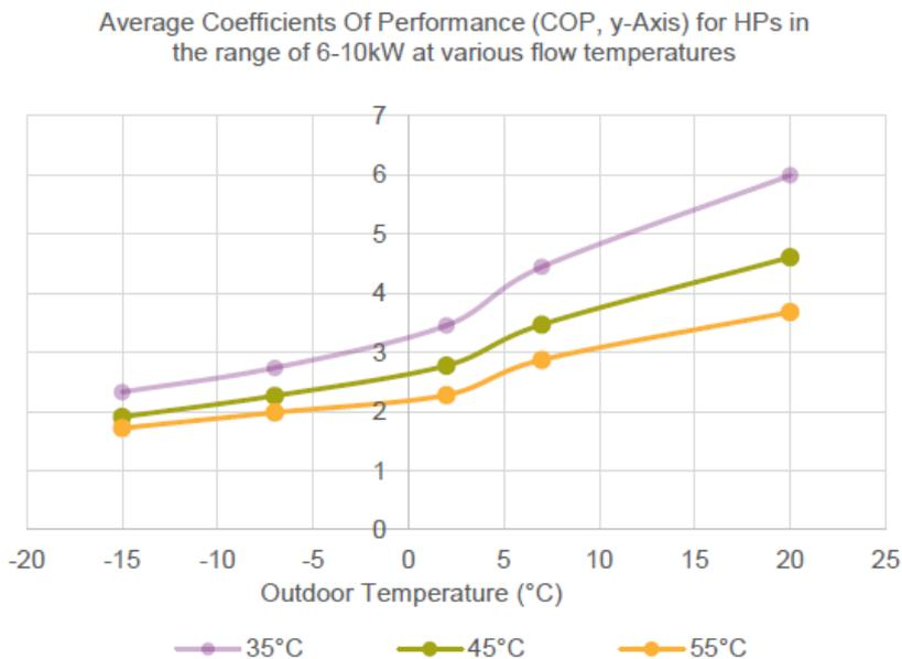
Figure 4-12: Changes in COP against OAT and supply temperature (source: figure from [36])
