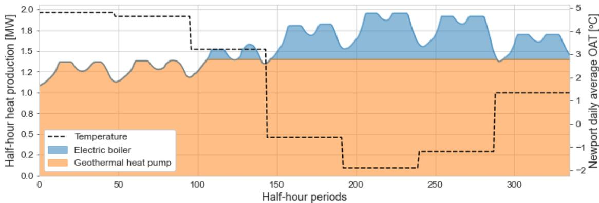
Figure 4-23: An example of the half-hourly heat production of a district heating system with 1.4 MW of geothermal HPs and 0.7 MW of electric boilers for 7 days. The flat tops are due to the use of thermal storage to decrease the peaks.
