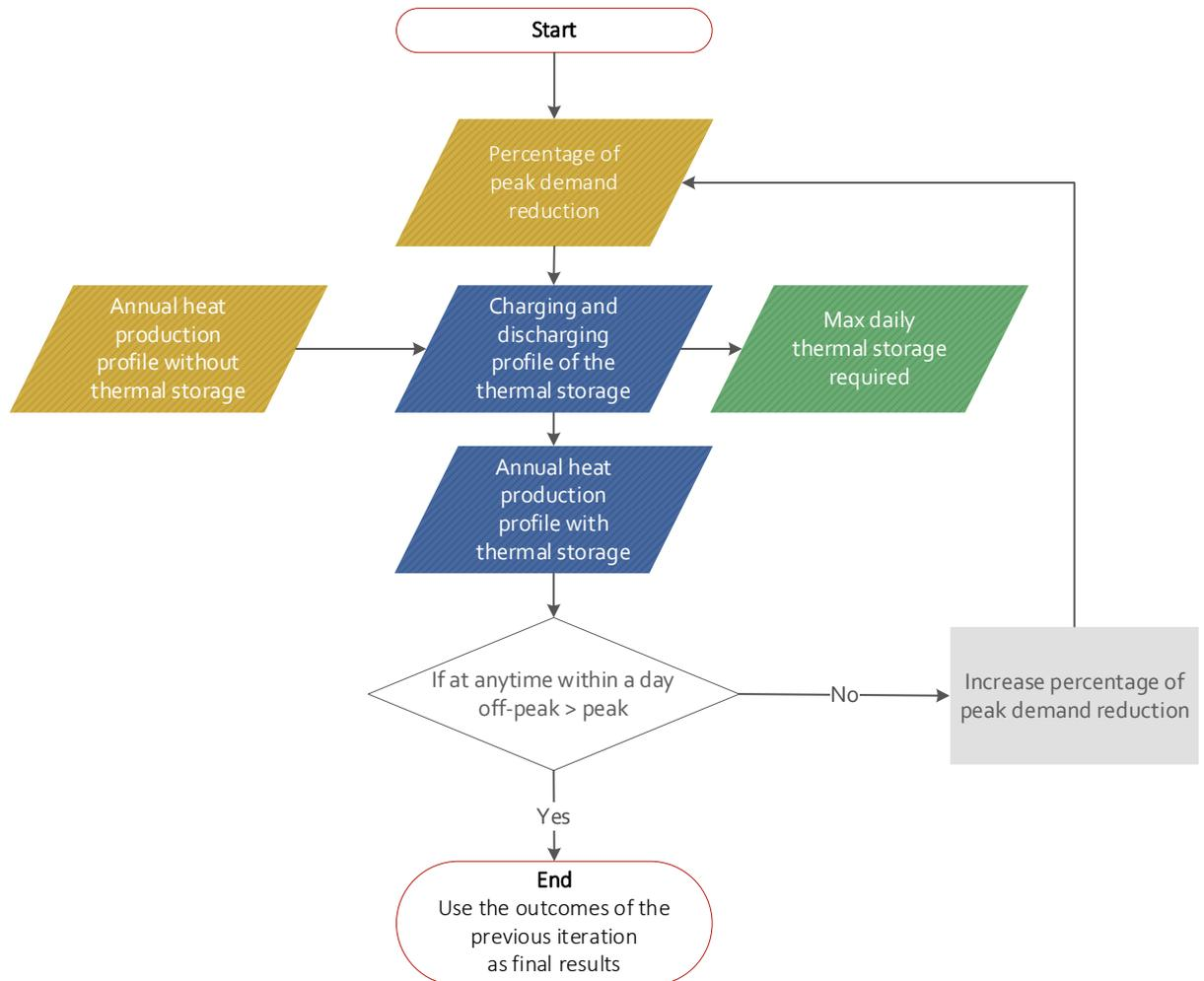
Figure 4-21: The iterative process that was used to calculate the size of the thermal storage and derive the heat production profile of district heating with thermal storage.
