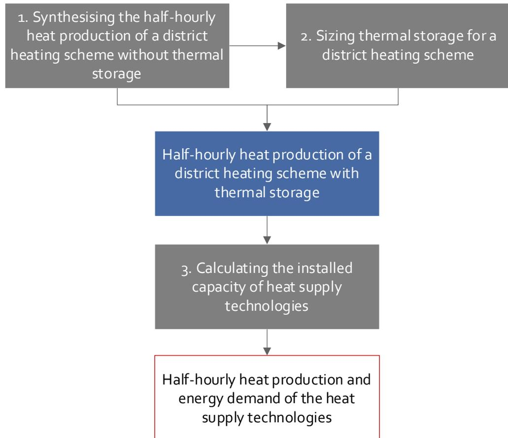
Figure 4-19: Methodology to synthesise half-hourly heat production and energy demand of the heat supply units of a district heating.
