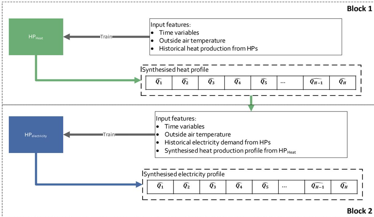
Figure 4-3: Process to produce half-hourly electricity consumption and heat production for HPs with two distinct models  $HP_{heat}$  and  $HP_{electricity}$
