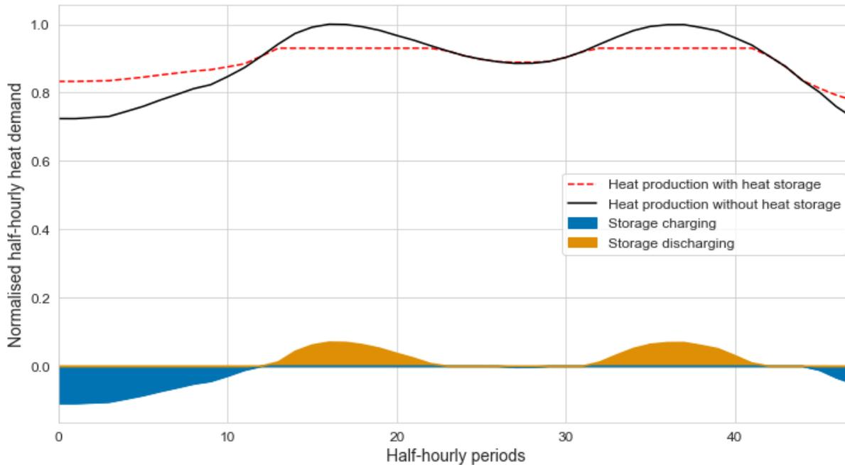
Figure 4-20: Example of the charging and discharging behaviour of a thermal storage unit for a day based on a normalised min-max half-hourly heat production
