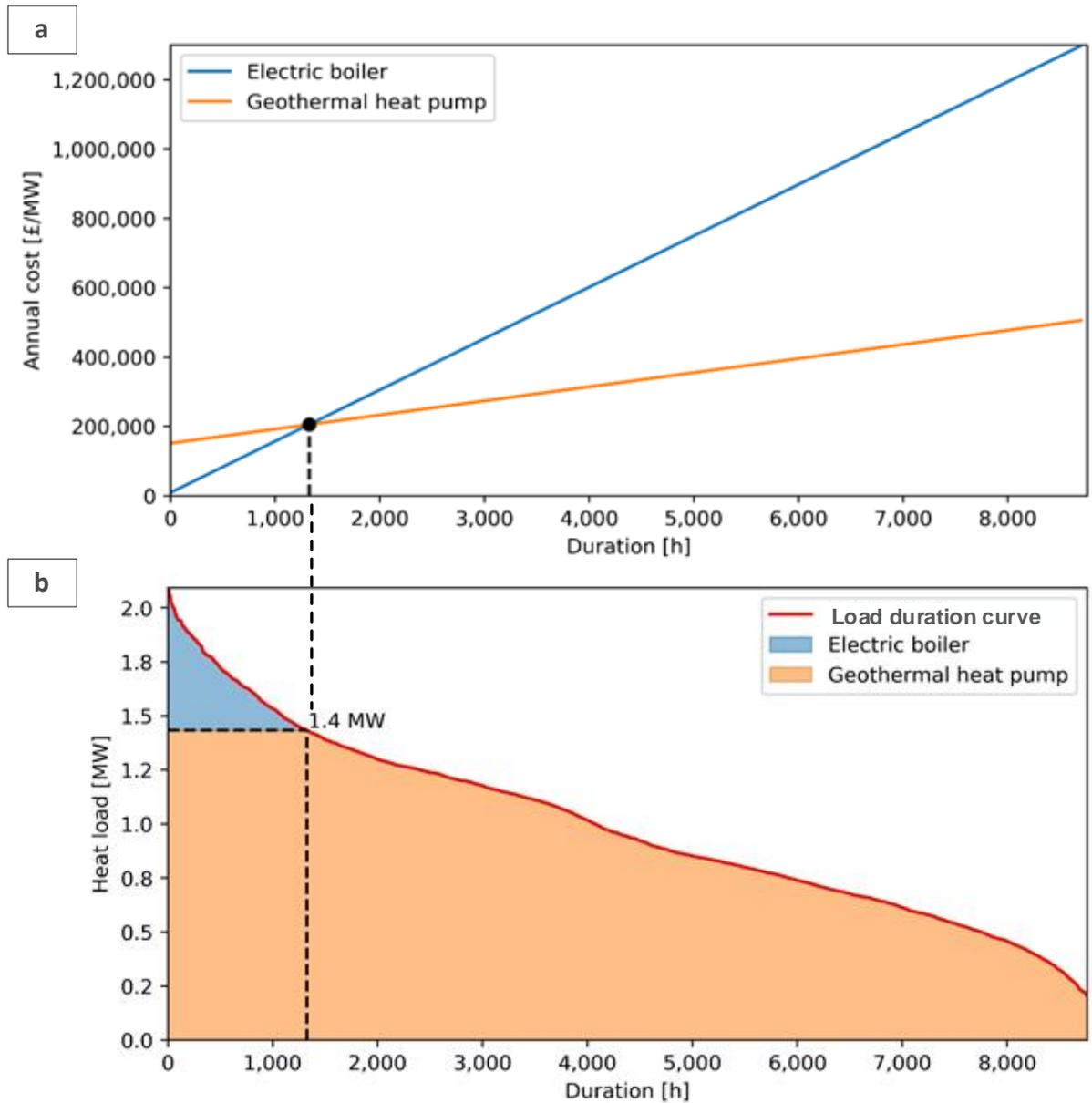
Figure 4-22: Panel a shows the screening curves for two electricity-based units (source of costs from [71]). Panel b shows an example of how the information from the screening curves for electric boiler and geothermal HPs was applied to a load duration curve to calculate the installed capacity of each technology. The load duration curve represents the domestic and non-domestic demand of a LSOA in Swansea.
