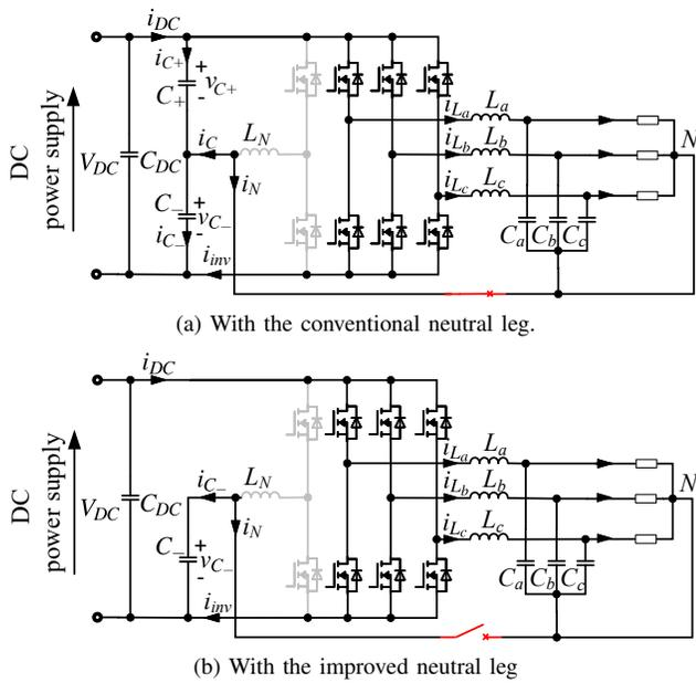
Fig. 28. Three-phase four-wire inverter with neutral legs in open-circuit failure mode.
