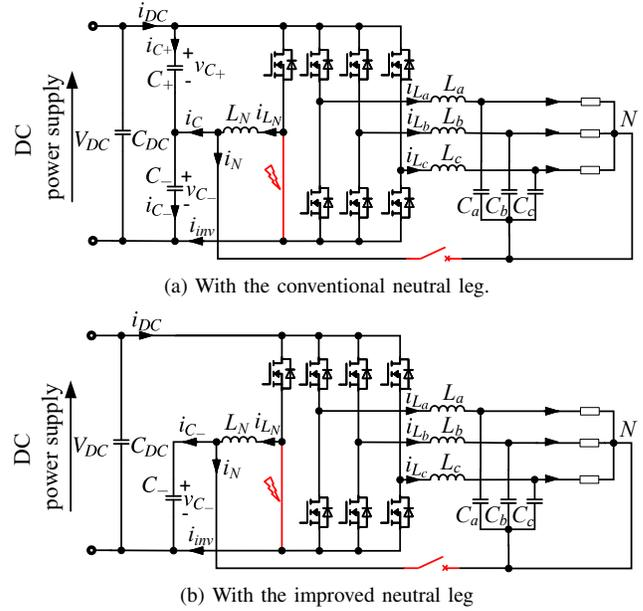
Fig. 27. Three-phase four-wire inverter with neutral legs in short-circuit failure mode (lower switch).
