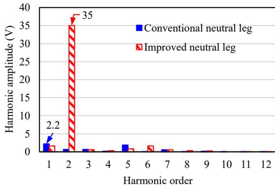
Fig. 18. FFT analysis of capacitor voltage  $V_{C-}$ .
