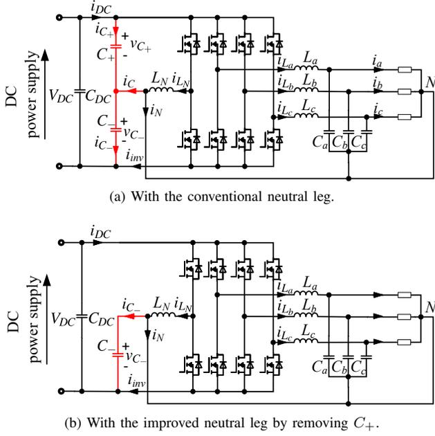
Fig. 2. Three-phase four-wire inverter with neutral legs.
