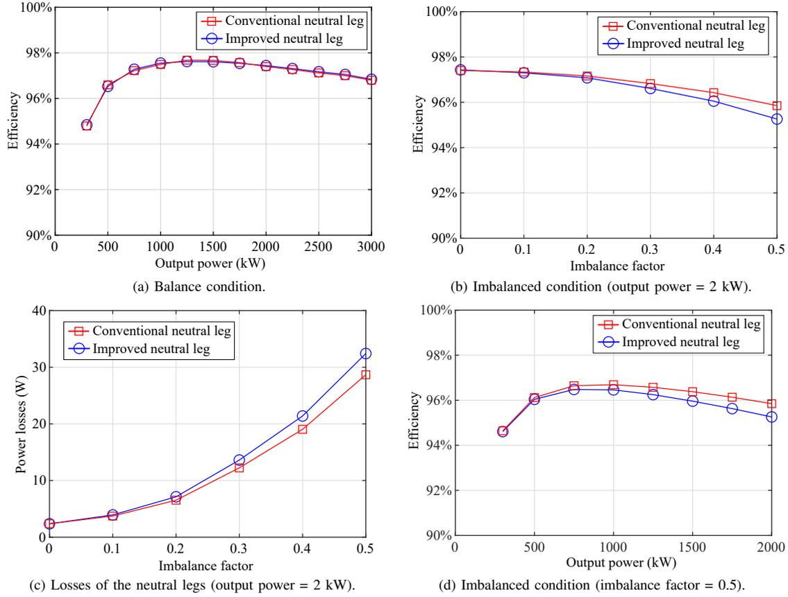
Fig. 23. Efficiency of three-phase four-wire inverters with conventional and improved neutral legs.
