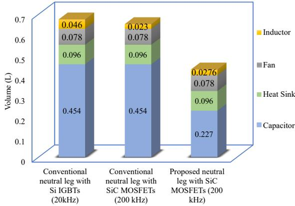
Fig. 3. Volume comparison of main passive components of conventional neutral legs with Si IGBTs, SiC MOSFETs and the improved neutral leg with SiC MOSFETs for a 10 kW three-phase inverter. The total volumes of the components are 0.674 L, 0.651 L, 0.429 L, respectively. Detailed calculations are provided in the Appendix.
