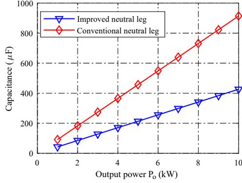
Fig. 4. Comparison of total dc capacitance ( $V_{max} = 750$  V, imbalance factor  $\delta = 0.5$ ).
