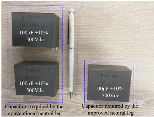
Fig. 16. Size comparison of the capacitors used in the conventional (left) and improved (right) neutral legs.
