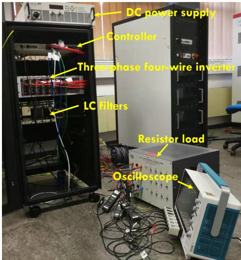
Fig. 15. Experimental setup of the three-phase four-wire inverter.
