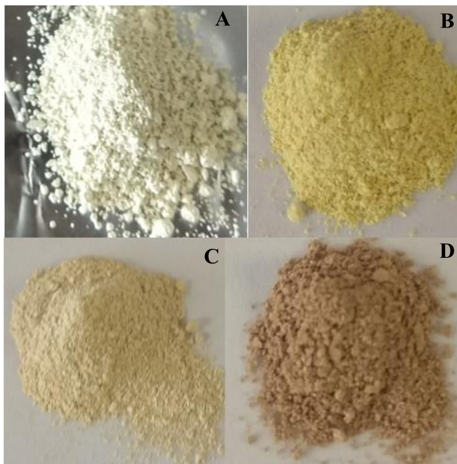
Figure 5.13 UiO-66(Zr)-NH 2 samples before treatment (fresh, A) and after treatment with methanol (B), ethanol (C), and water (D), 120 h at 110°C. Photographs taken by Ricardo Navar.
