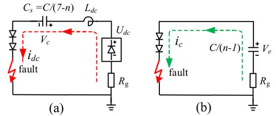
Fig. 9. Equivalent circuits after the fault. Discharging of: (a) dc link; (b) dc capacitors in converter cells.
