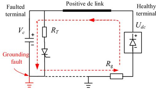
Fig. 12. Equivalent circuit of the post-fault condition (fault occurs at the 6<sup>th</sup> cell).
