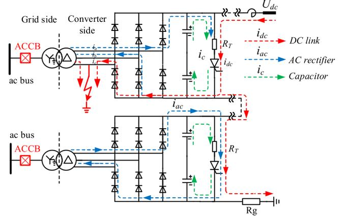
Fig. 11. Current paths after blocking of converters with thyristor branch.
