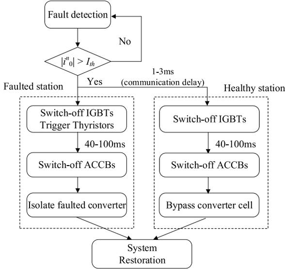
Fig. 14. Fault isolation process.
