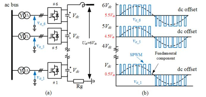
Fig. 6. Relationship of ac-and dc-side voltages. (a) DC-side (b) AC-side.
