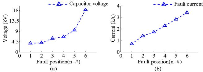
Fig. 16. Effect of the fault location. (a) Capacitor voltages. (b) Peak values of fault current.
