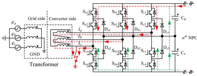
Fig. 7. Zero-sequence current path following a converter-side fault at phase c.
