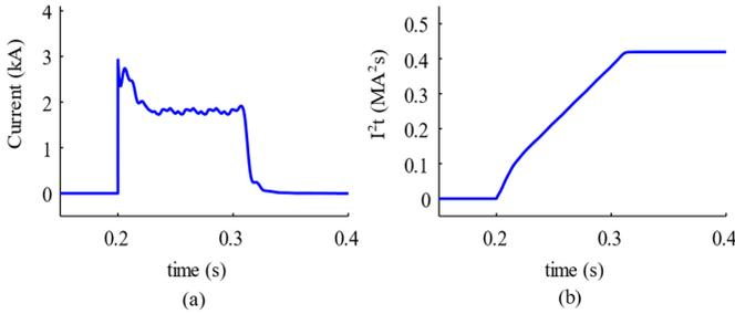
Fig. 19. Waveforms of thyristor branch. (a) Current. (b)  $I^2t$ .
