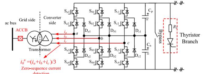
Fig. 10. Thyristor branch-based protection method.
