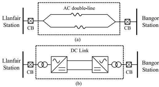
Fig. 2. ANGLE-DC project: conversion from ac into dc. (a) Existing double-circuit ac lines (33 kV). (b) Converted MVDC link ( $\pm 27$  kV dc).
