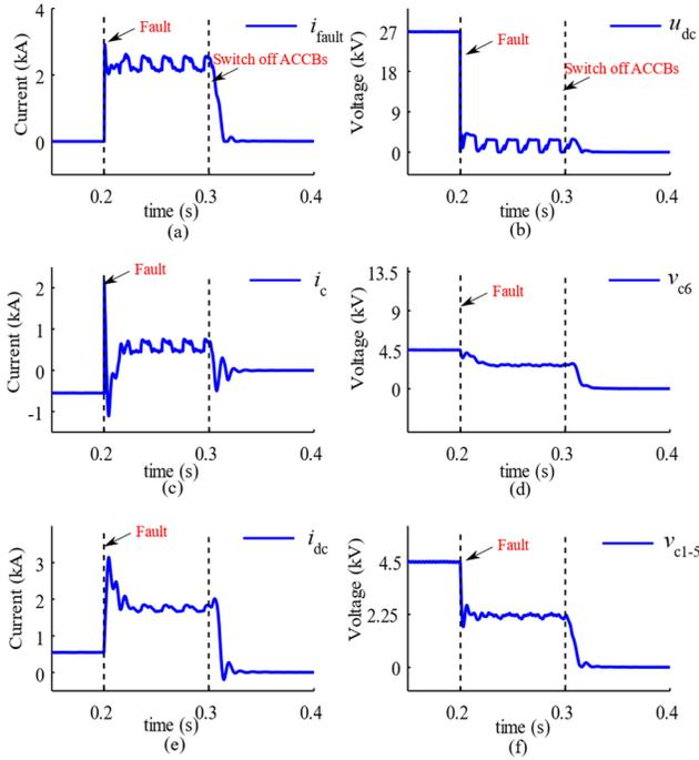
Fig. 18. Trigger the thyristor branch when a fault occurs at  $n = 6$ . (a) Fault current. (b) DC link voltage. (c) Capacitor current. (d) Capacitor voltage  $n = 6$ . (e) DC link current. (f) Capacitor voltage ( $n = 1, \dots, 5$ ).
