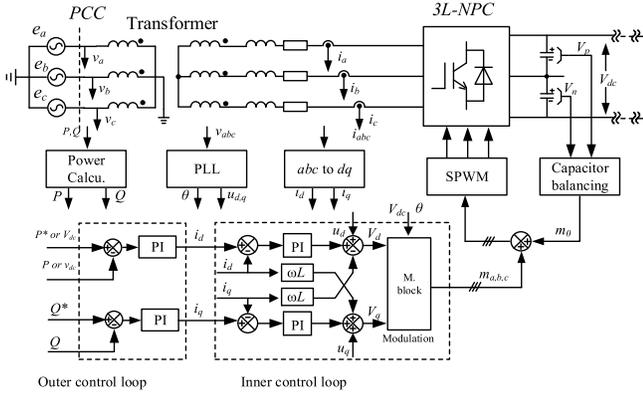
Fig. 5. Control block diagram of the cascaded 3L-NPC converters.
