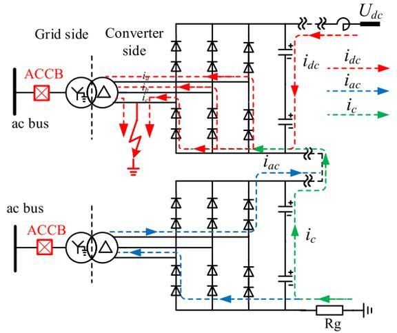
Fig. 8. Current paths through the diodes after blocking of converters.
