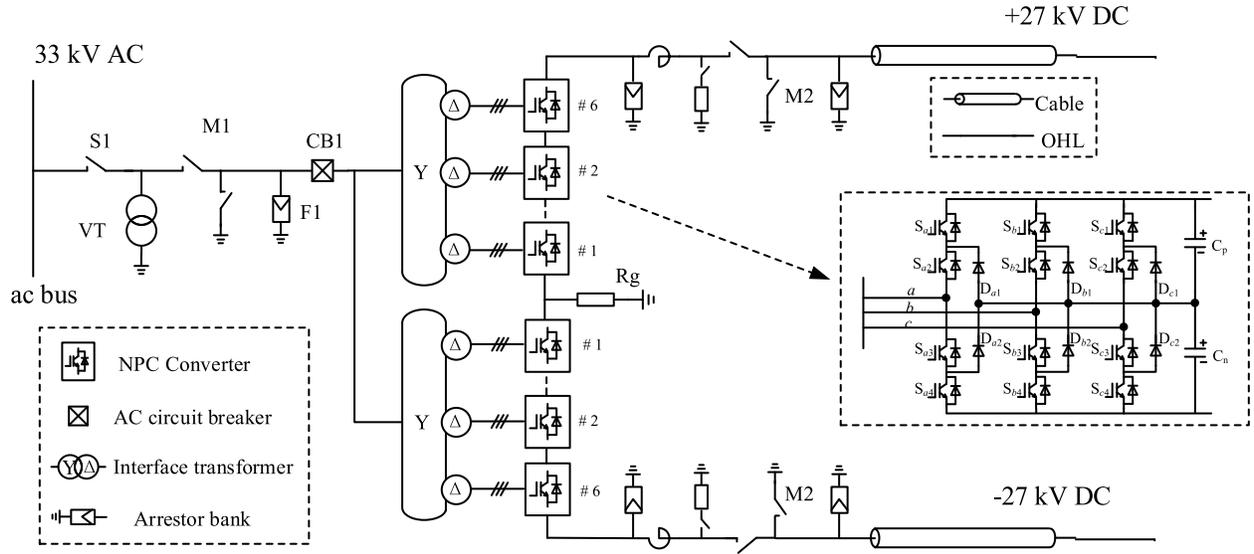
Fig. 3. System configuration of the ANGLE-DC project with cascaded 3L-NPC converters.
