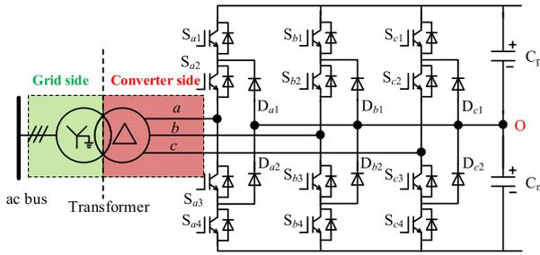
Fig. 4. Topology of 3L-NPC converter cell with interface transformer.
