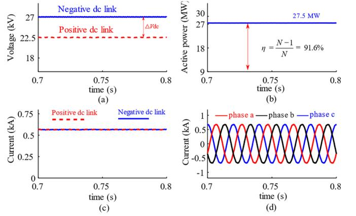
Fig. 20. Post-fault operation. (a) DC link voltage. (b) Active power. (c) DC link current. (d) Grid-side ac currents.
