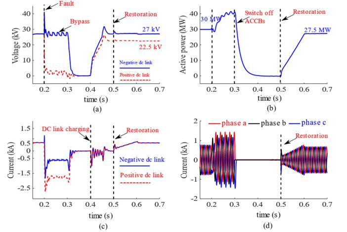
Fig. 21. System protection and restoration following a converter-side ac fault. (a) DC link voltage. (b) Active power. (c) DC link current. (d) Grid-side ac currents.
