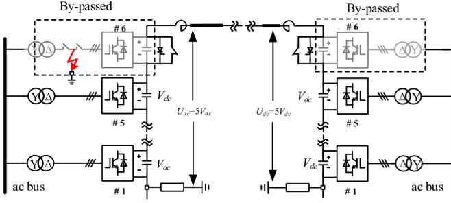
Fig. 13. Post-fault operation (only positive pole is given).
