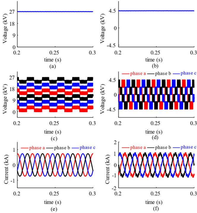
Fig. 15. Relevant waveforms under normal conditions. (a) DC link voltage. (b) DC voltage of one 3L-NPC converter cell. (c) Converter-side phase-to-ground voltages of six 3L-NPC converter cells (phase A). (d) Converter-side line-to-line voltage of one 3L-NPC converter cell. (e) Grid-side ac currents. (f) Converter-side ac currents of one 3L-NPC converter cell.
