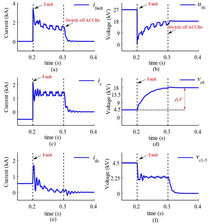
Fig. 17. Blocking the converter only when a fault occurs at  $n = 6$ . (a) Fault current. (b) DC link voltage. (c) Capacitor discharging current. (d) Capacitor voltage of the 6<sup>th</sup> cell. (e) DC link current. (f) Capacitor voltage of the cells ( $n = 1, \dots, 5$ ).
