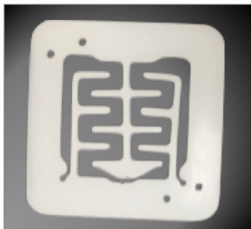
Figure 1.32. FEP spacer with flow channel design.
